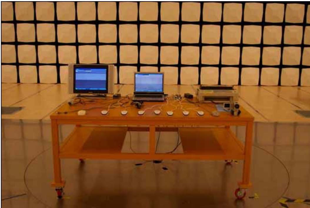
Picture 3. Radiated emission (Front)
