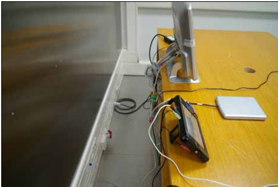
Picture 2. Conducted emission (Rear)
