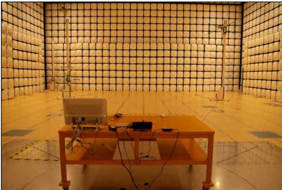
Picture 4. Radiated emission (Rear)
