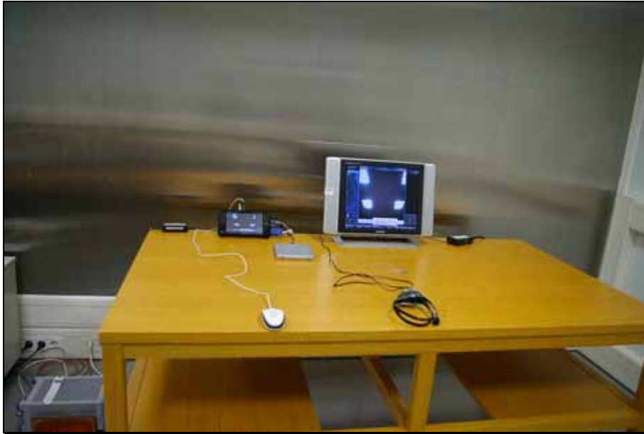
Picture 1. Conducted emission (Front)
