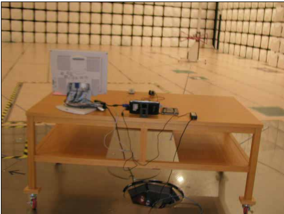
Picture 4. Radiated emission (Rear)
