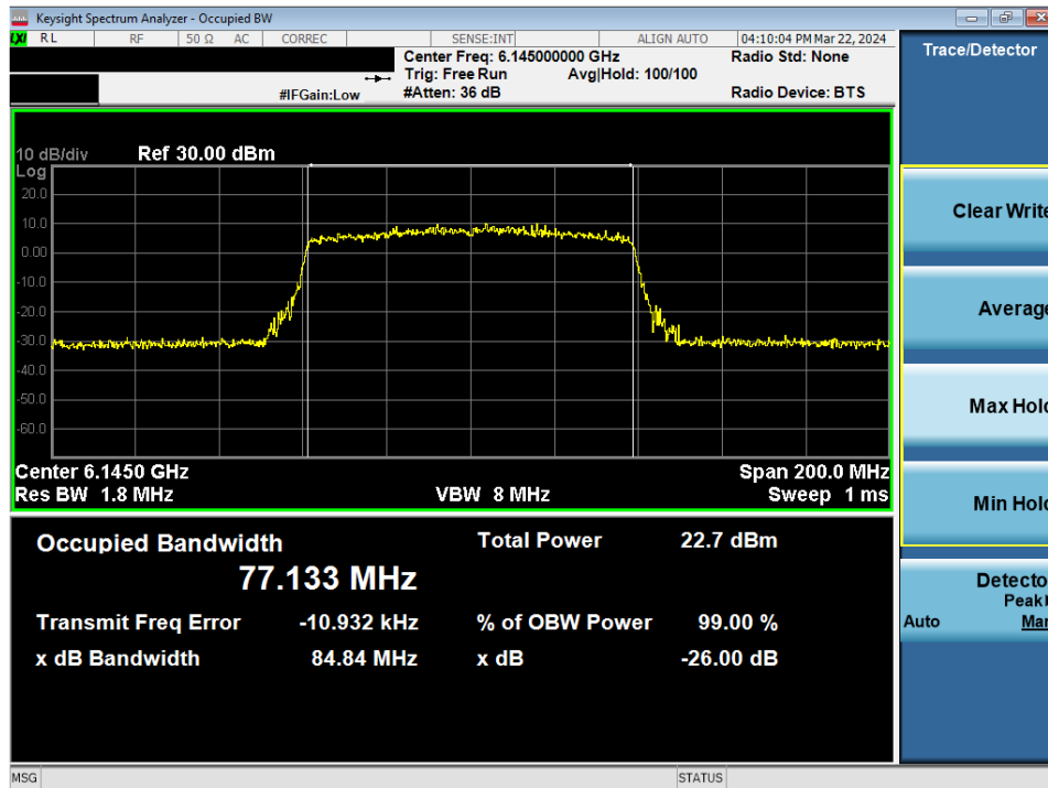
Plot 7-30. 26dB Bandwidth Plot MIMO ANT2 (80MHz 802.11ax/be (UNII Band 5) – Ch. 39)
