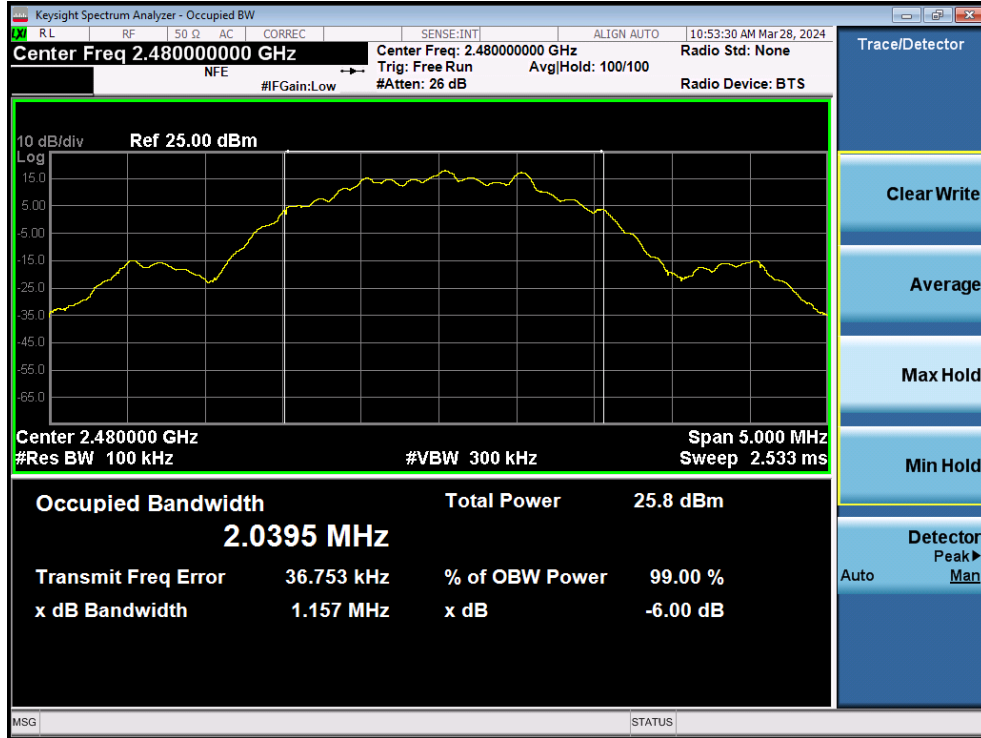
Plot 7-19. 6dB Bandwidth Plot (Bluetooth (LE), 2Mbps – Ch. 39 – Ant2)
