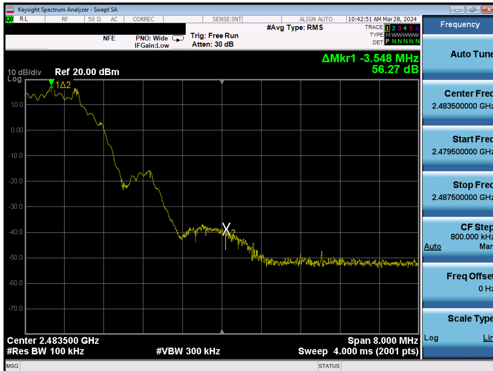
Plot 7-99. Band Edge Plot (Bluetooth (LE), 2Mbps – Ch. 39) – Ant1
