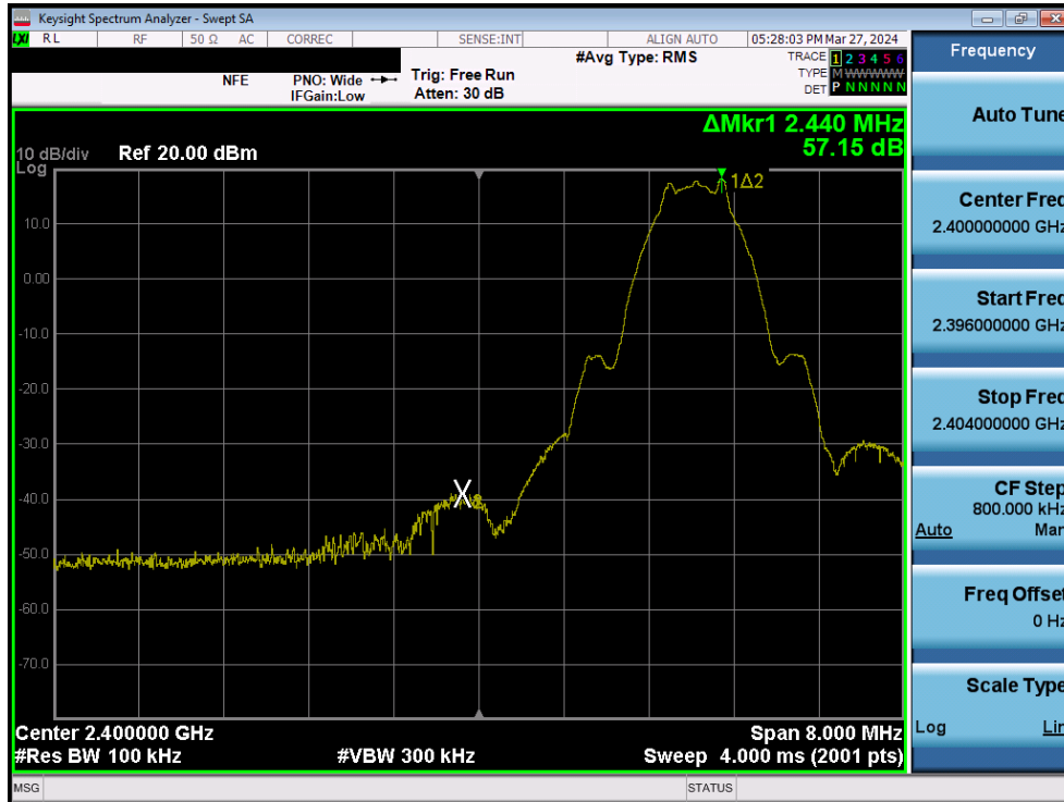
Plot 7-96. Band Edge Plot (Bluetooth (LE), 1Mbps – Ch. 0) – Ant1
