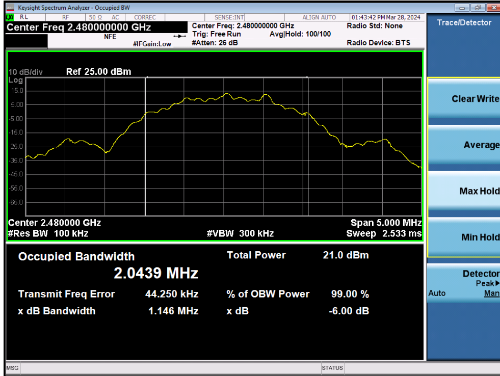
Plot 7-31. 6dB Bandwidth Plot (Bluetooth (LE), 2Mbps – Ch. 39 – Dual Ant2)
