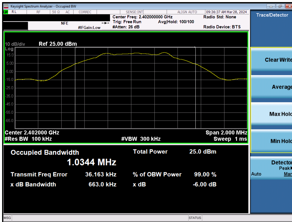
Plot 7-14. 6dB Bandwidth Plot (Bluetooth (LE), 1Mbps – Ch. 0 – Ant2)
