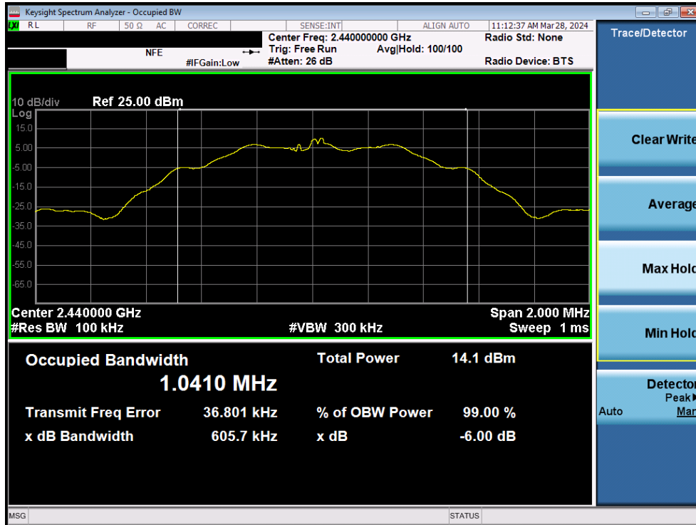
Plot 7-3. 6dB Bandwidth Plot (Bluetooth (LE), 125kbps – Ch. 19 – Ant1)
