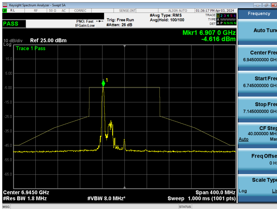
Plot 7-325. In-Band Emission Plot MIMO ANT2 (80MHz BW 802. 11be (26 Tones) (UNII Band 8) – Ch. 199)
