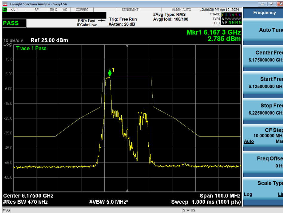
Plot 7-285. In-Band Emission Plot MIMO ANT1 (20MHz BW 802.11be (26 Tones) (UNII Band 5) – Ch. 45) - SP
