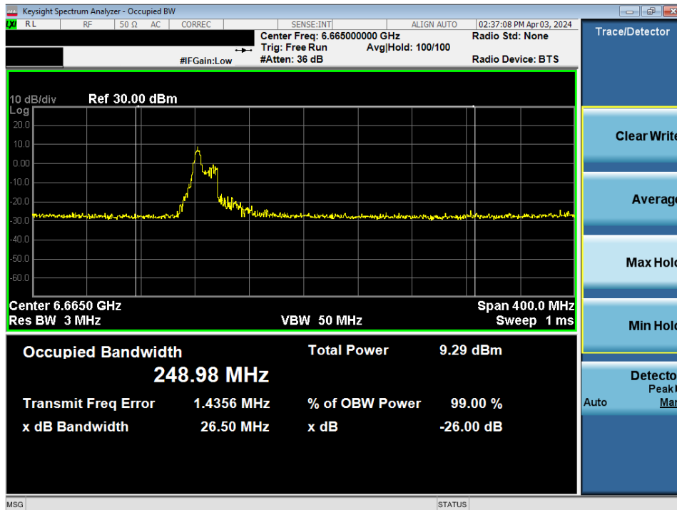
Plot 7-56. Occupied Bandwidth Plot MIMO ANT2 (160MHz BW 802. 11be (26 Tones) (UNII Band 7) – Ch. 143)
