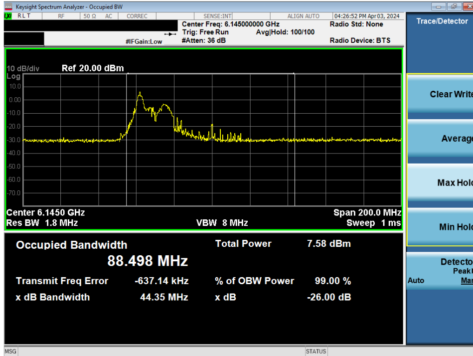
Plot 7-5. Occupied Bandwidth Plot MIMO ANT1 (80MHz BW 802. 11be (26 Tones) (UNII Band 5) – Ch. 39)
