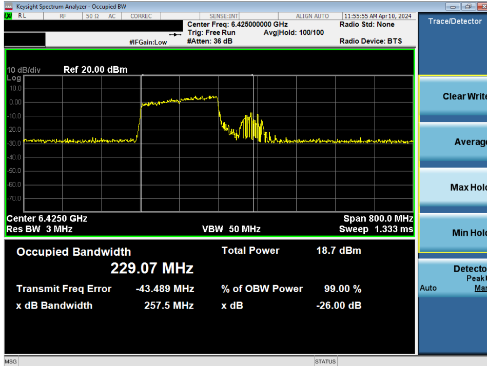
Plot 7-72. Occupied Bandwidth Plot MIMO ANT2 (320MHz BW 802. 11be (Full Tones) (UNII Band 6) – Ch. 95)
