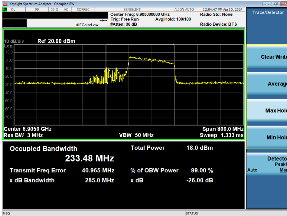
Plot 7-82. Occupied Bandwidth Plot MIMO ANT2 (320MHz BW 802. 11be (Full Tones) (UNII Band 8) – Ch. 191)
