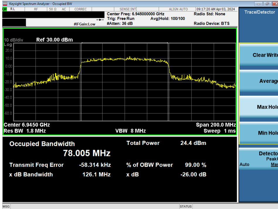
Plot 7-80. Occupied Bandwidth Plot MIMO ANT2 (80MHz BW 802. 11be (Full Tone) (UNII Band 8) – Ch. 199)
