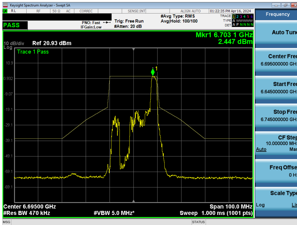
Plot 7-272. In-Band Emission Plot MIMO ANT1 (20MHz BW 802.11be (26 Tone) (UNII Band 7) – Ch. 149) – SP
