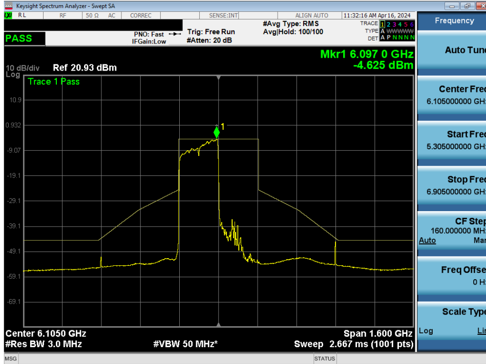
Plot 7-239. In-Band Emission Plot MIMO ANT1 (320MHz BW 802. 11be (Full Tones) (UNII Band 5) – Ch. 31) – LPI & SP
