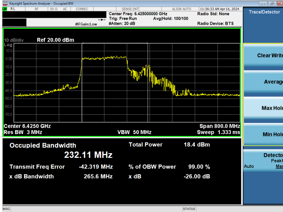
Plot 7-30. Occupied Bandwidth Plot MIMO ANT1 (320MHz BW 802. 11be (Full Tones) (UNII Band 6) – Ch. 95)
