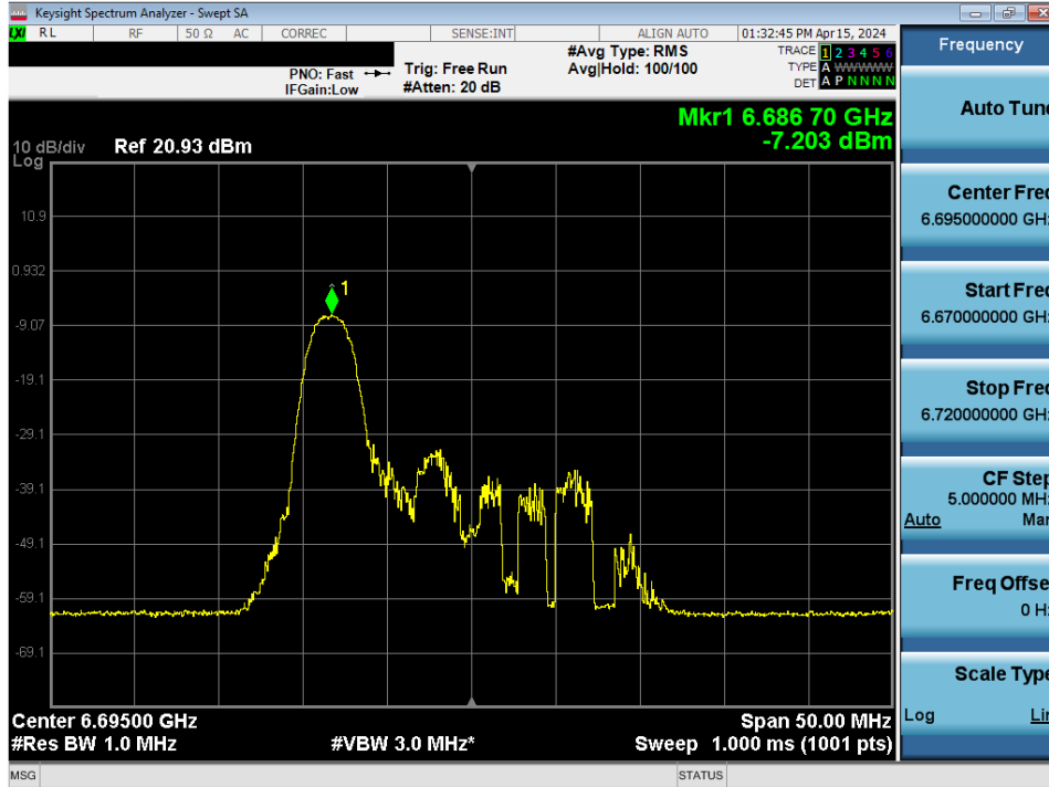
Plot 7-91. Power Spectral Density Plot MIMO ANT1 (20MHz BW 802. 11be (26 Tones) (UNII Band 7) – Ch. 149) - LPI
