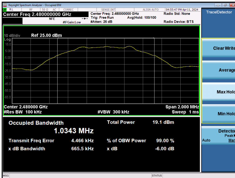
Plot 7-27. 6dB Bandwidth Plot (Bluetooth (LE), 1Mbps – Ch. 39 – Dual Ant2)
