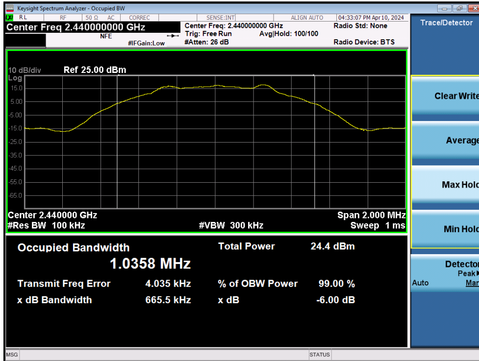
Plot 7-8. 6dB Bandwidth Plot (Bluetooth (LE), 1Mbps – Ch. 19 – Ant1)
