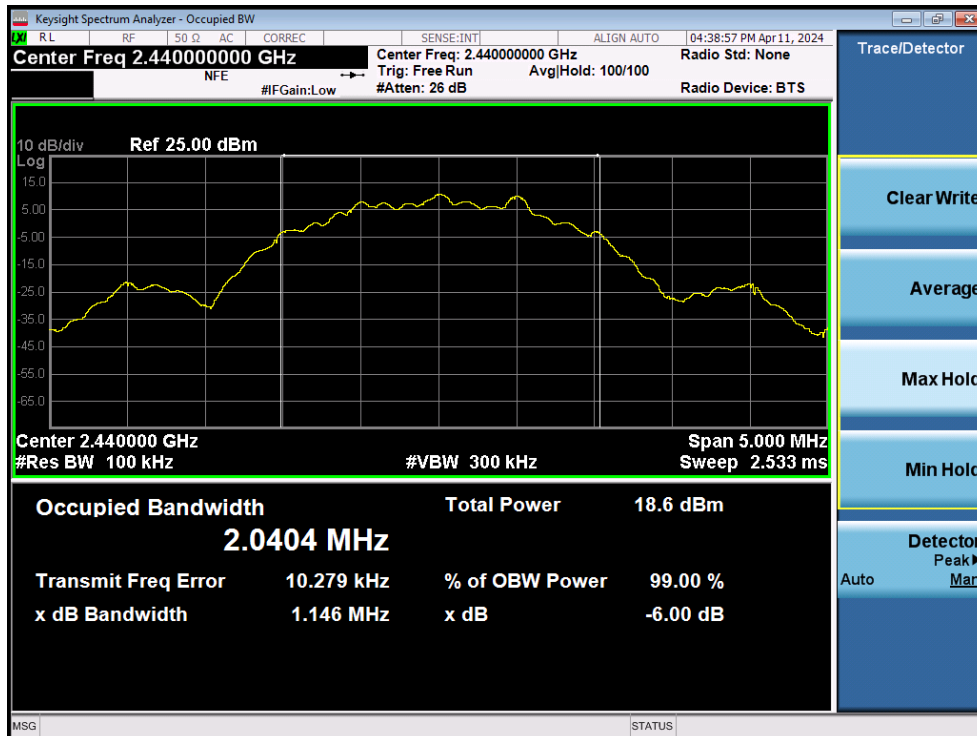
Plot 7-23. 6dB Bandwidth Plot (Bluetooth (LE), 2Mbps – Ch. 19 – Dual Ant1)
