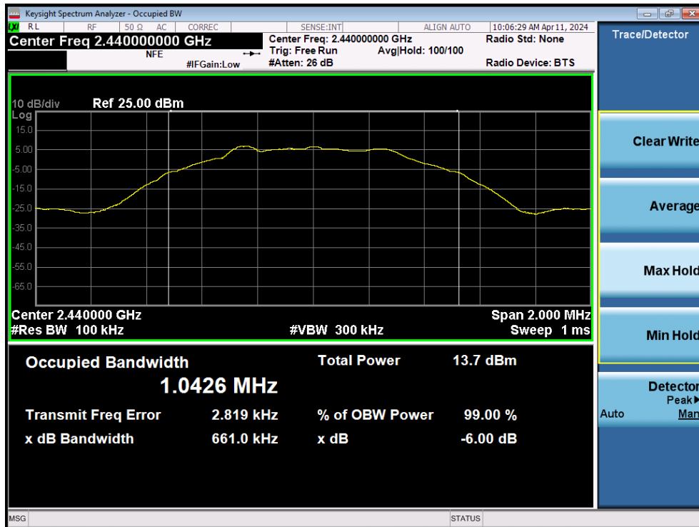
Plot 7-5. 6dB Bandwidth Plot (Bluetooth (LE), 500kbps – Ch. 19 – Ant1)
