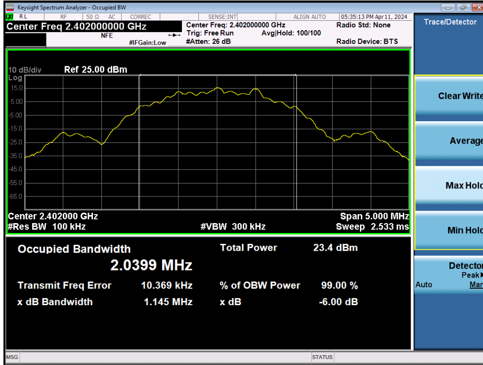
Plot 7-16. 6dB Bandwidth Plot (Bluetooth (LE), 2Mbps – Ch. 0 – Ant2)
