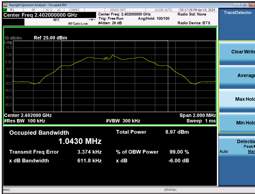
Plot 7-1. 6dB Bandwidth Plot (Bluetooth (LE), 125kbps – Ch. 0 – Ant1)
