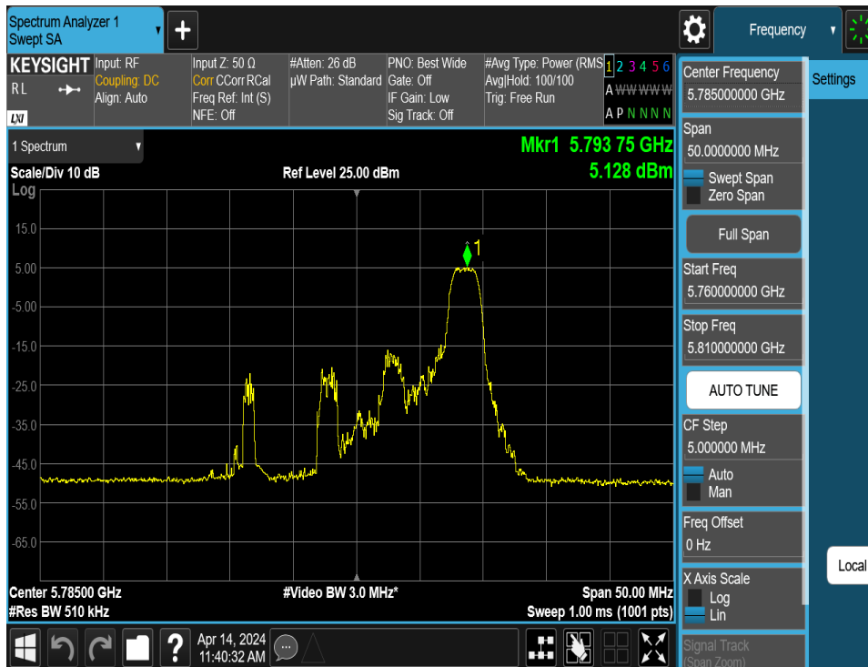
Plot 7-138. Power Spectral Density Plot MIMO ANT2 (20MHz BW 802.11be – 26 Tones (UNII Band 3) – Ch. 157)
