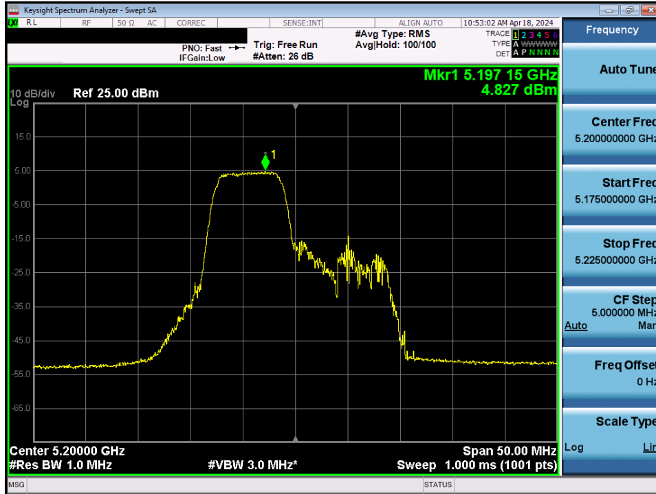
Plot 7-163. Power Spectral Density Plot MIMO ANT2 (20MHz BW 802.11be – 52+26 Tones (UNII Band 1) – Ch. 40)
