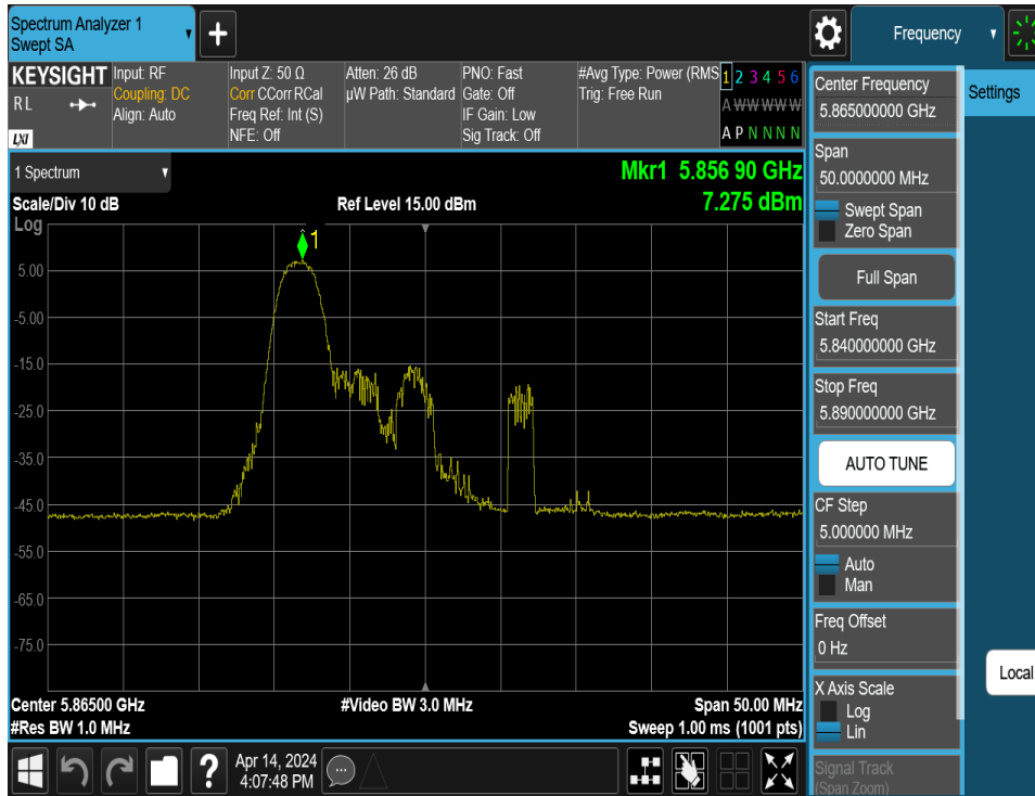
Plot 7-141. Power Spectral Density Plot MIMO ANT2 (20MHz BW 802.11be – 26 Tones (UNII Band 4) – Ch. 173)
