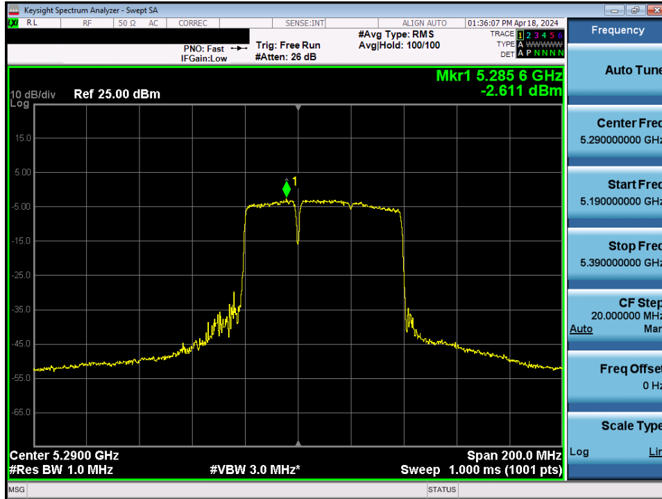
Plot 7-169. Power Spectral Density Plot MIMO ANT2 (80MHz BW 802.11be – 484+242Tones (UNII Band 2A) – Ch. 58)
