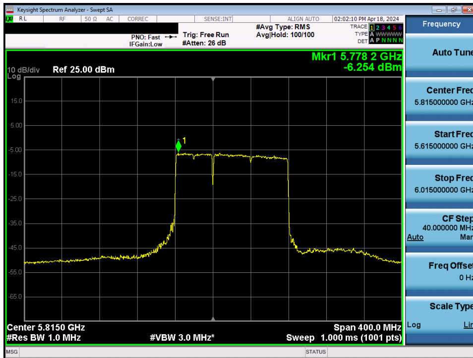
Plot 7-180. Power Spectral Density Plot MIMO ANT2 (160MHz BW 802.11be – 996+484 Tones (UNII Band 3/4) – Ch. 163)
