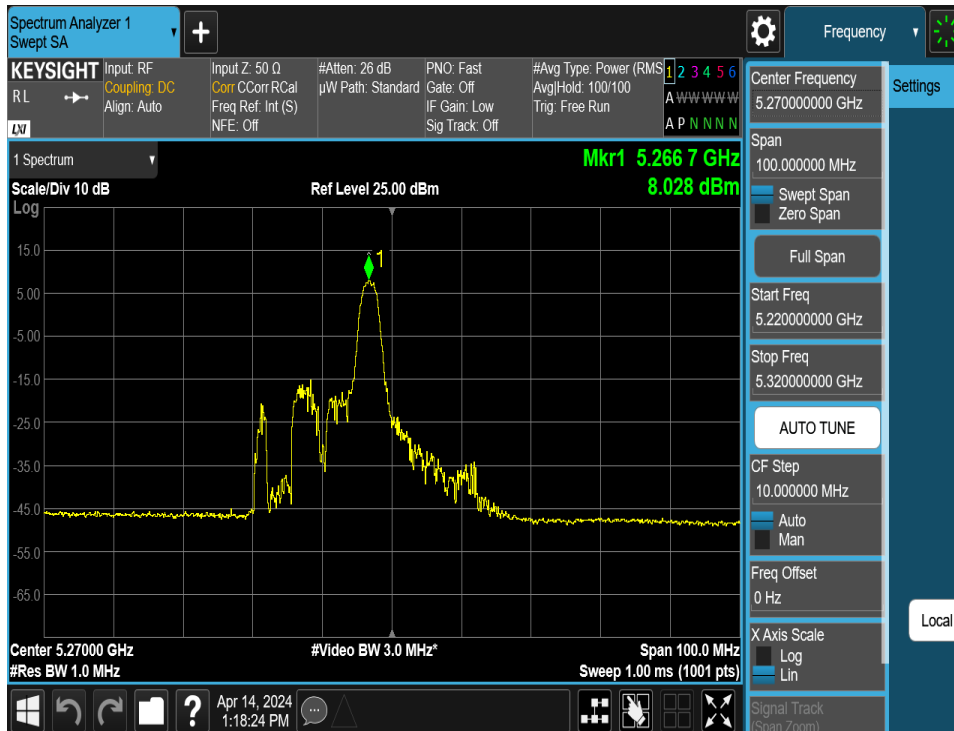
Plot 7-132. Power Spectral Density Plot MIMO ANT2 (40MHz BW 802.11be – 26 Tones (UNII Band 2A) – Ch. 54)
