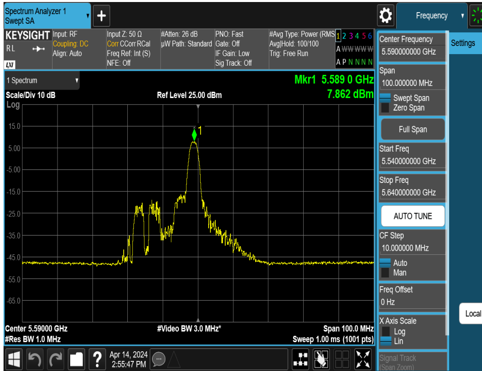
Plot 7-135. Power Spectral Density Plot MIMO ANT2 (40MHz BW 802.11be – 26 Tones (UNII Band 2C) – Ch. 118)
