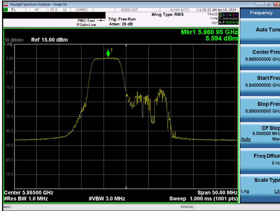
Plot 7-123. Power Spectral Density Plot MIMO ANT1 (20MHz BW 802.11be – 52+26 Tones (UNII Band 4) – Ch. 173)
