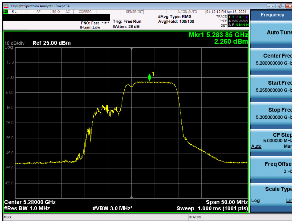
Plot 7-114. Power Spectral Density Plot MIMO ANT1 (20MHz BW 802.11be – 106+26 Tones (UNII Band 2A) – Ch. 56)
