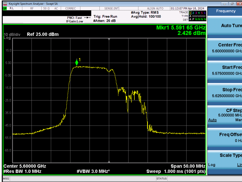
Plot 7-117. Power Spectral Density Plot MIMO ANT1 (20MHz BW 802.11be – 106+26 Tones (UNII Band 2C) – Ch. 120)
