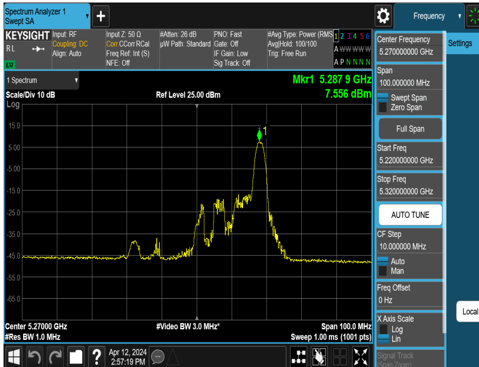
Plot 7-78. Power Spectral Density Plot MIMO ANT1 (40MHz BW 802.11be – 26 Tones (UNII Band 2A) – Ch. 54)
