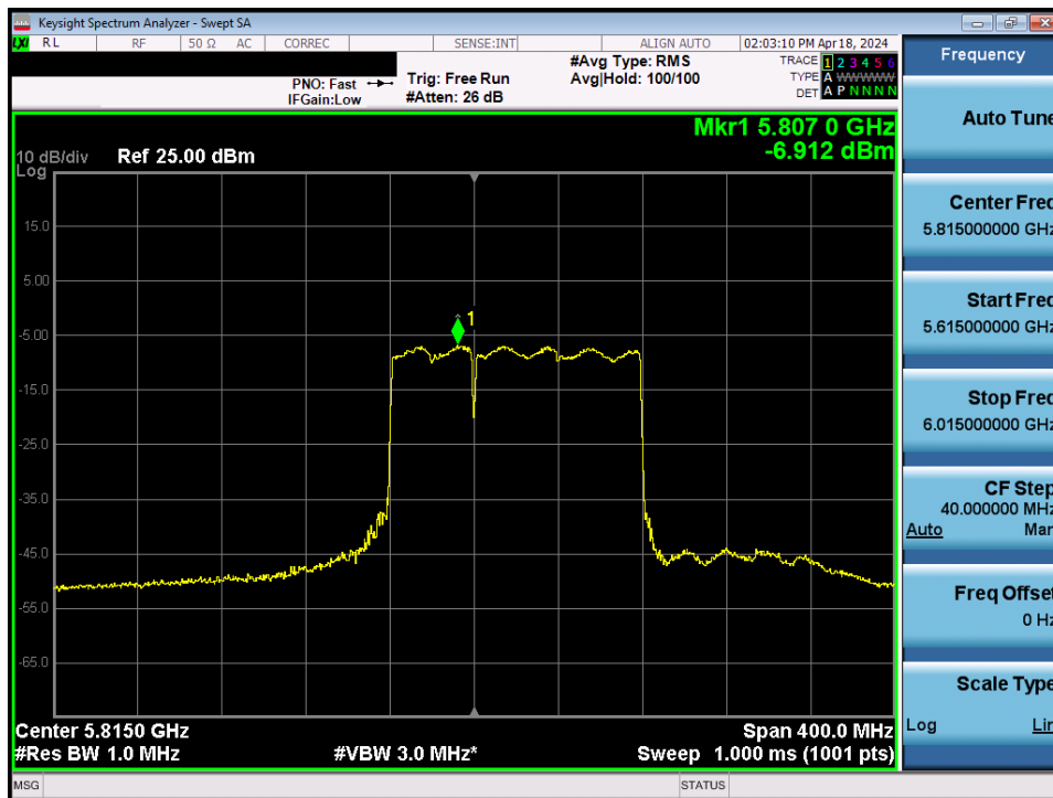
Plot 7-126. Power Spectral Density Plot MIMO ANT1 (160MHz BW 802.11be – 996+484 Tones (UNII Band 3/4) – Ch. 163)
