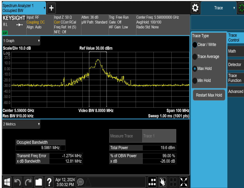
Plot 7-9. 26dB Bandwidth Plot MIMO ANT1 (40MHz BW 802.11be – 26 Tones (UNII Band 2C) – Ch. 118)
