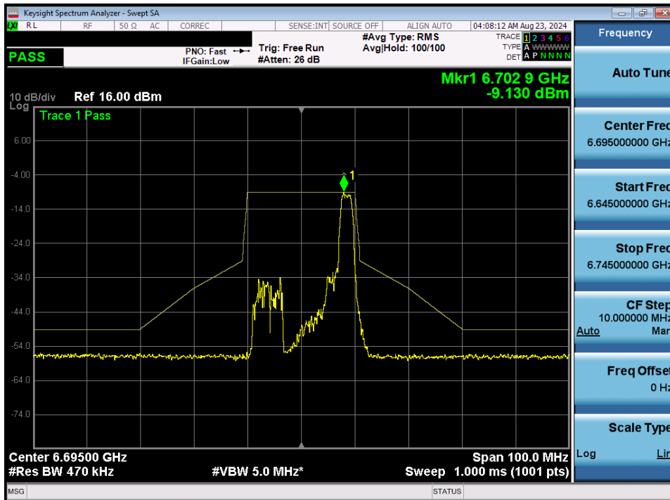
Plot 7-338. In-Band Emission Plot MIMO ANT2 (20MHz BW 802.11ax/be (26 Tones) (UNII Band 7) – Ch. 149) – LPI
