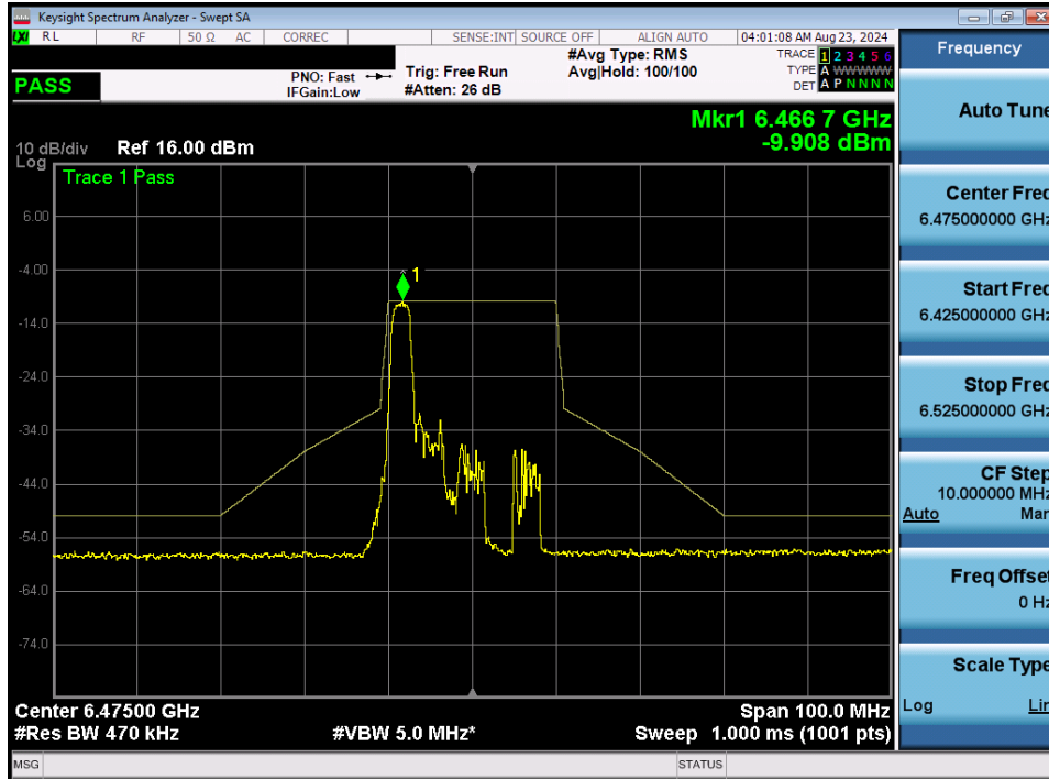
Plot 7-333. In-Band Emission Plot MIMO ANT2 (20MHz BW 802.11ax/be (26 Tones) (UNII Band 6) – Ch. 105) – LPI
