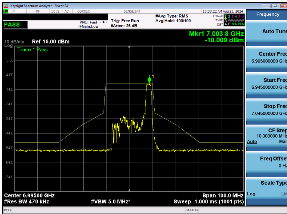
Plot 7-278. In-Band Emission Plot MIMO ANT1 (20MHz BW 802.11ax/be (26 Tones) (UNII Band 8) – Ch. 209) – LPI
