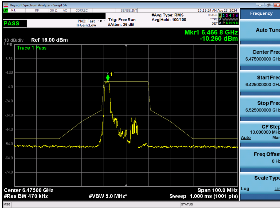
Plot 7-263. In-Band Emission Plot MIMO ANT1 (20MHz BW 802.11ax/be (26 Tones) (UNII Band 6) – Ch. 105) – LPI
