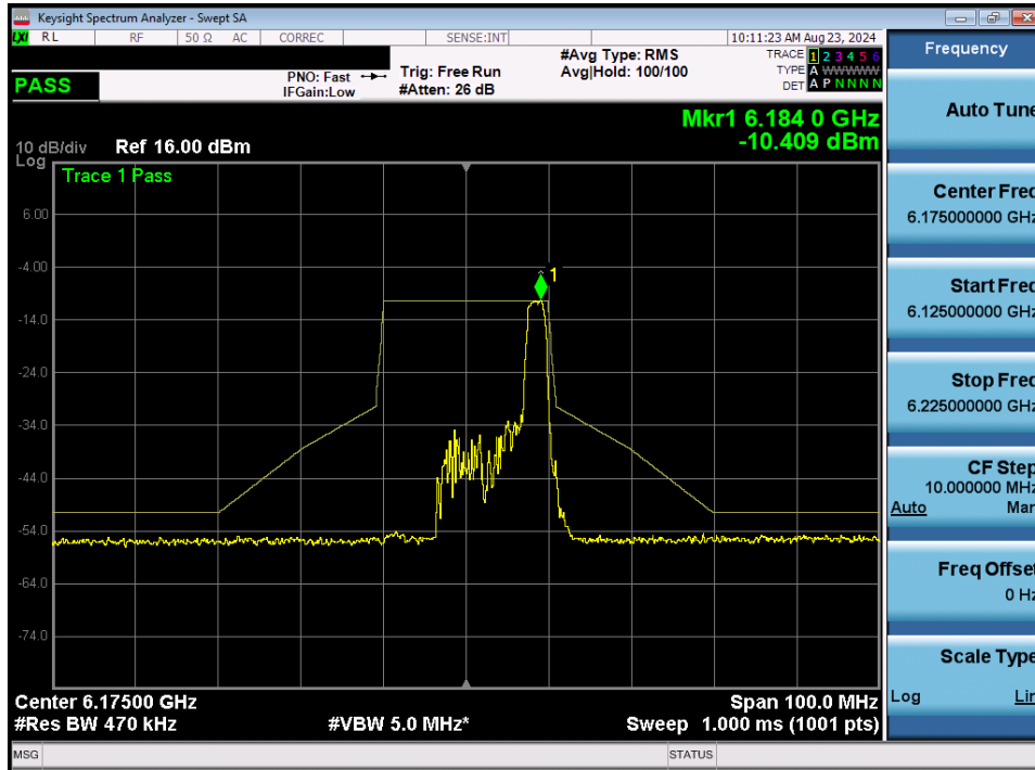
Plot 7-253. In-Band Emission Plot MIMO ANT1 (20MHz BW 802.11ax/be (26 Tones) (UNII Band 5) – Ch. 45) – LPI
