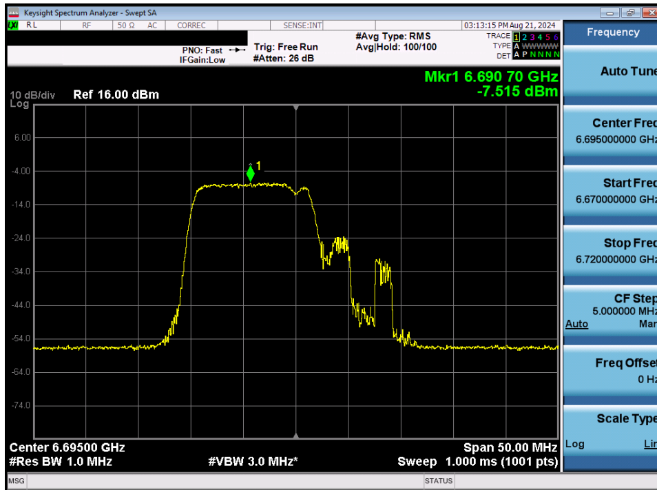
Plot 7-175. Power Spectral Density MIMO ANT1 (20MHz BW 802.11be (106+26 Tones) (UNII Band 7) – Ch. 149)
