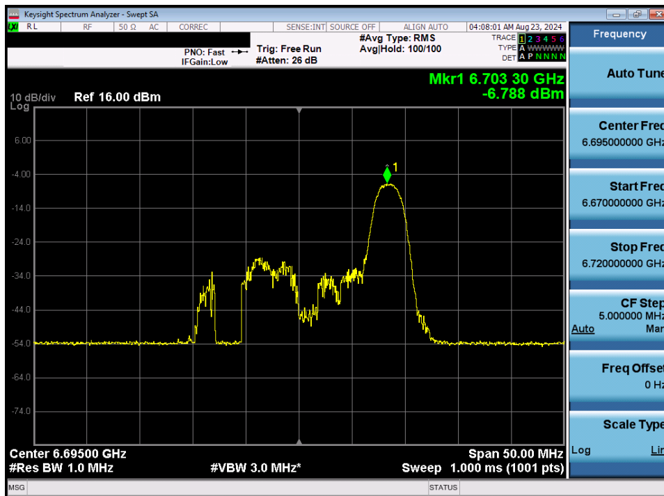
Plot 7-198. Power Spectral Density Plot MIMO ANT2 (20MHz BW 802.11ax/be (26 Tones) (UNII Band 7) – Ch. 149) – LPI
