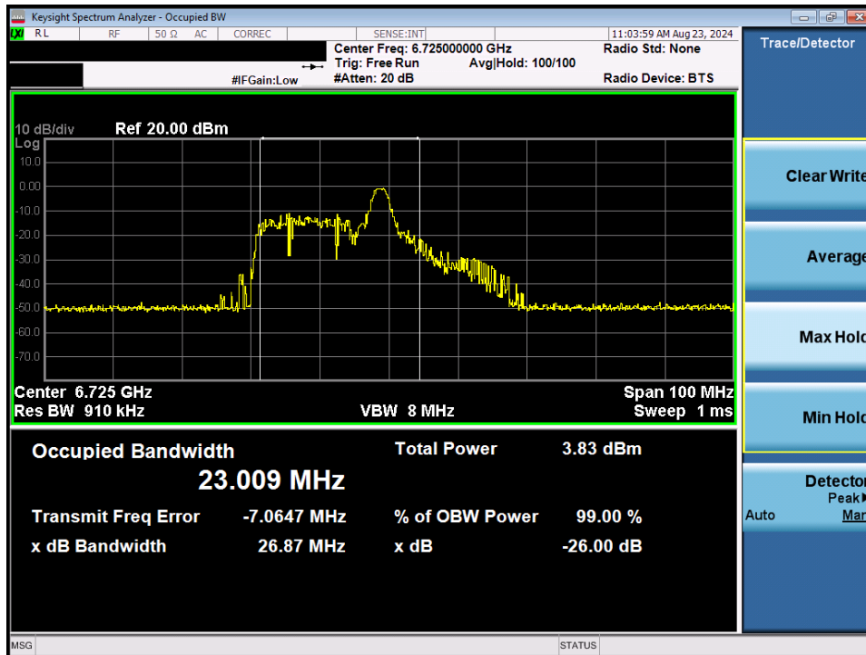
Plot 7-12. Occupied Bandwidth Plot MIMO ANT1 (40MHz BW 802.11ax/be (26 Tones) (UNII Band 7) – Ch. 155)
