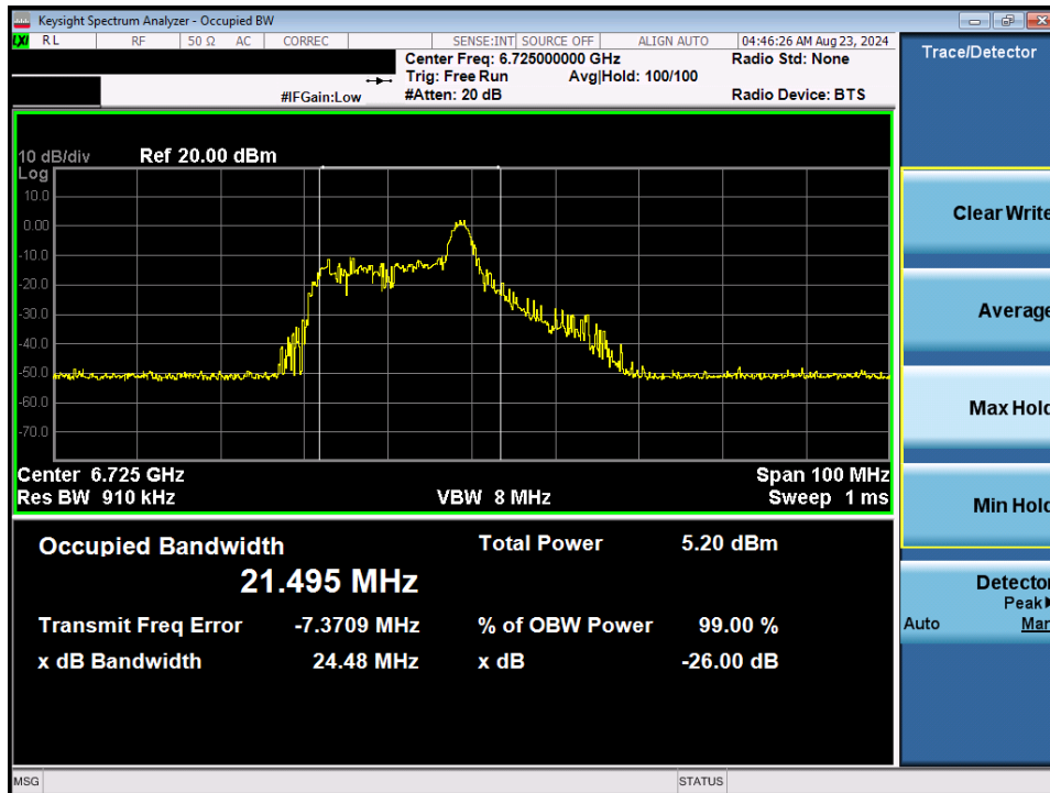
Plot 7-68. Occupied Bandwidth Plot MIMO ANT2 (40MHz BW 802.11ax/be (26 Tones) (UNII Band 7) – Ch. 155)
