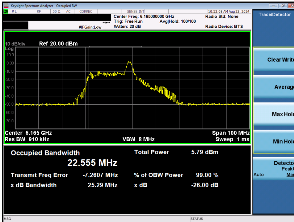
Plot 7-2. Occupied Bandwidth Plot MIMO ANT1 (40MHz BW 802.11ax/be (26 Tones) (UNII Band 5) – Ch. 43)
