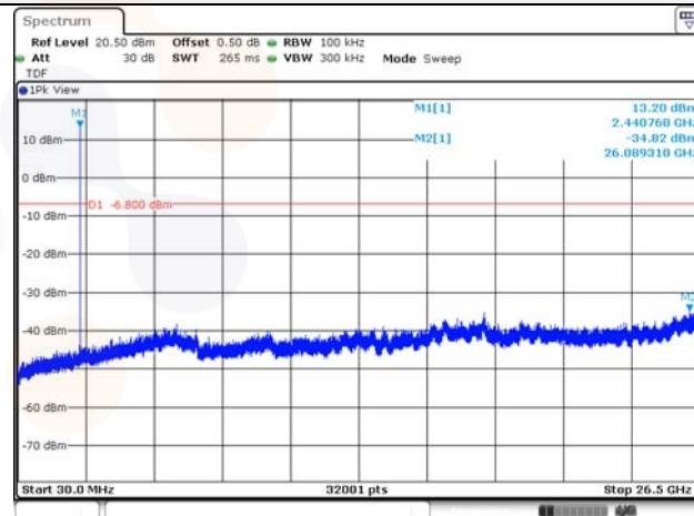
**Conducted band-edge / Hopping ch.**
