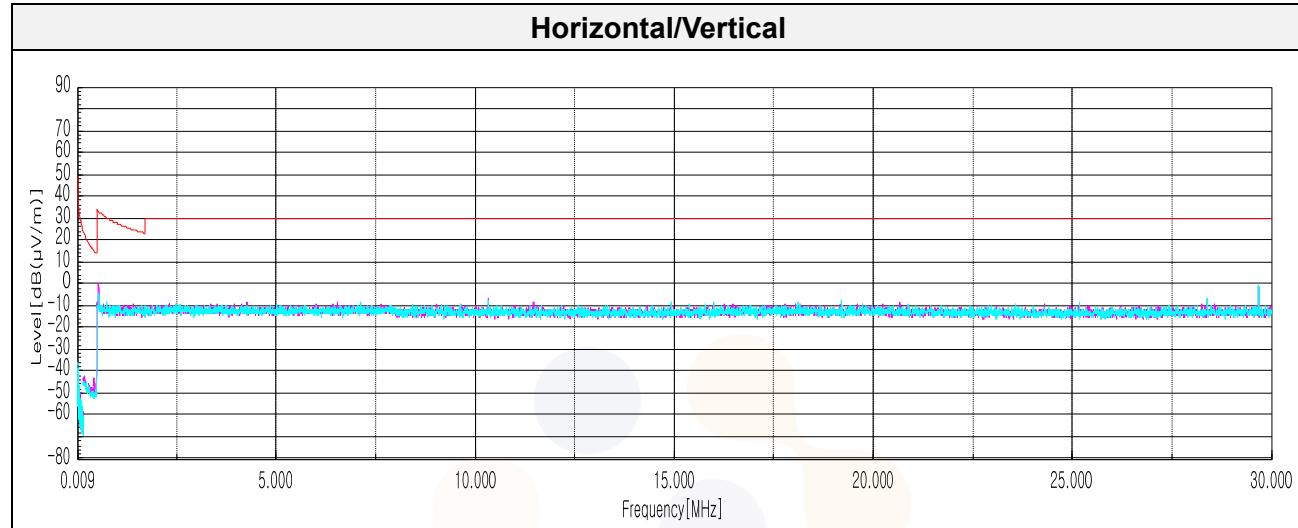
**Test results (Below 1 000 MHz) – Worst case: GFSK 2 441 MHz**
