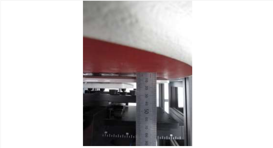
Distance of 6 mm from the EUT (WLAN ANT.1)
