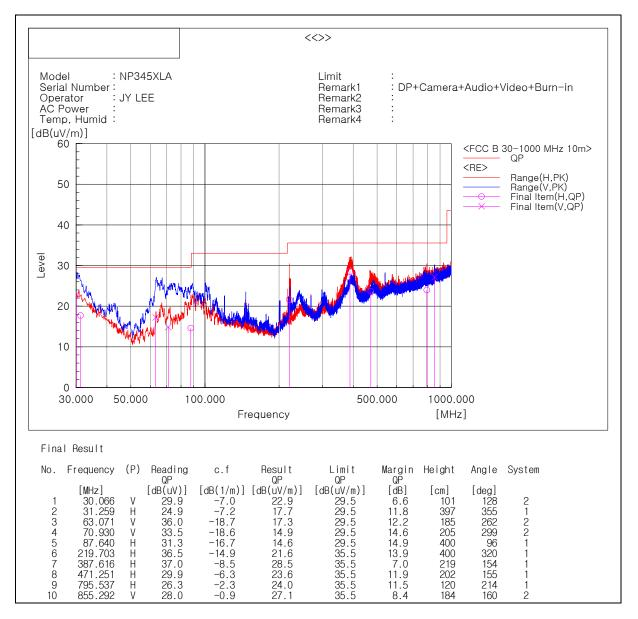
Note1) Receiving antenna polarization : Horizontal, Vertical Test Distance : 10 m, Antenna Height : 1 to 4 meters Result (QP) = Reading (QP) + c.f (Antenna Factor + Cable Loss - Amp. Gain) Margin (QP) = Limit - Level (QP)QP = Quasi-Peak, c.f = Correction Factor
