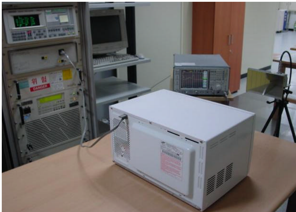
Fig. 2 Test Setup for Operating Frequency Measurements
