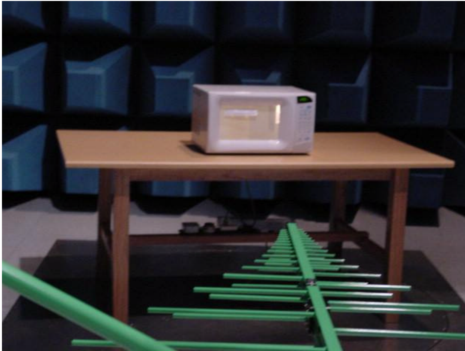
Fig. 3 Test Setup for Radiated Emission(30 - 1000MHz)
