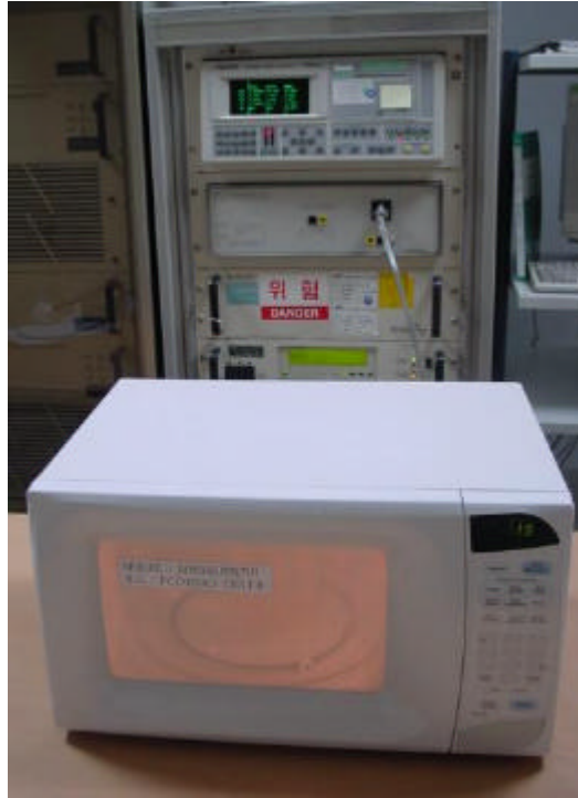
Fig. 2 Test Setup for Operating Frequency Measurements
