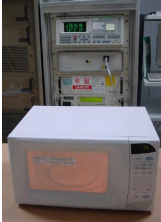
Fig. 2 Test Setup for Operating Frequency Measurements
