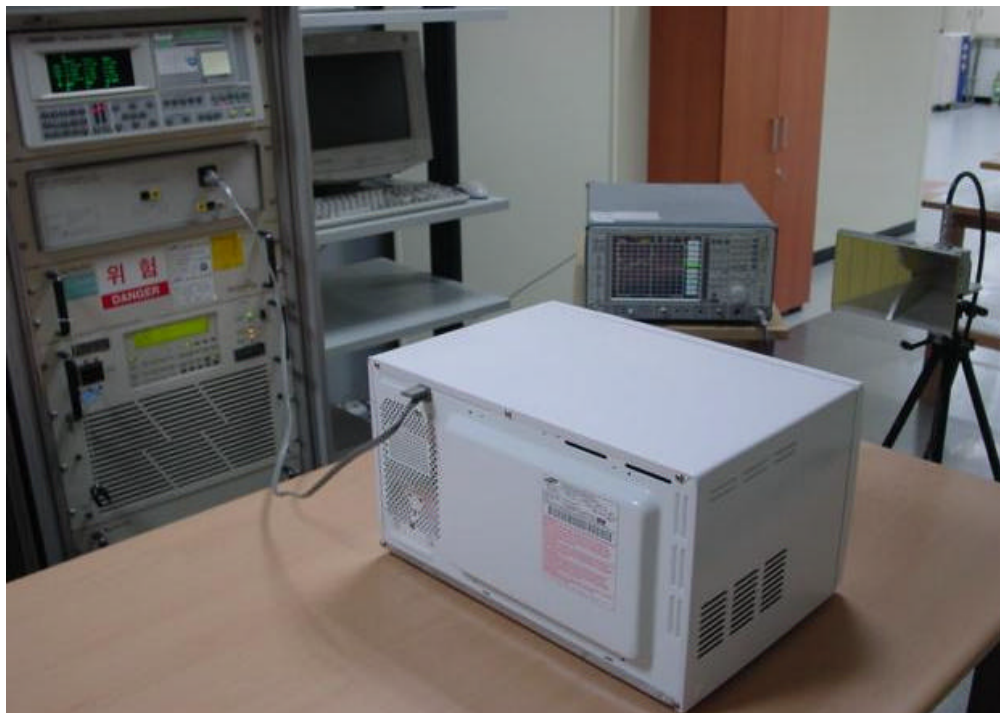
Fig. 2 Test Setup for Operating Frequency Measurements
