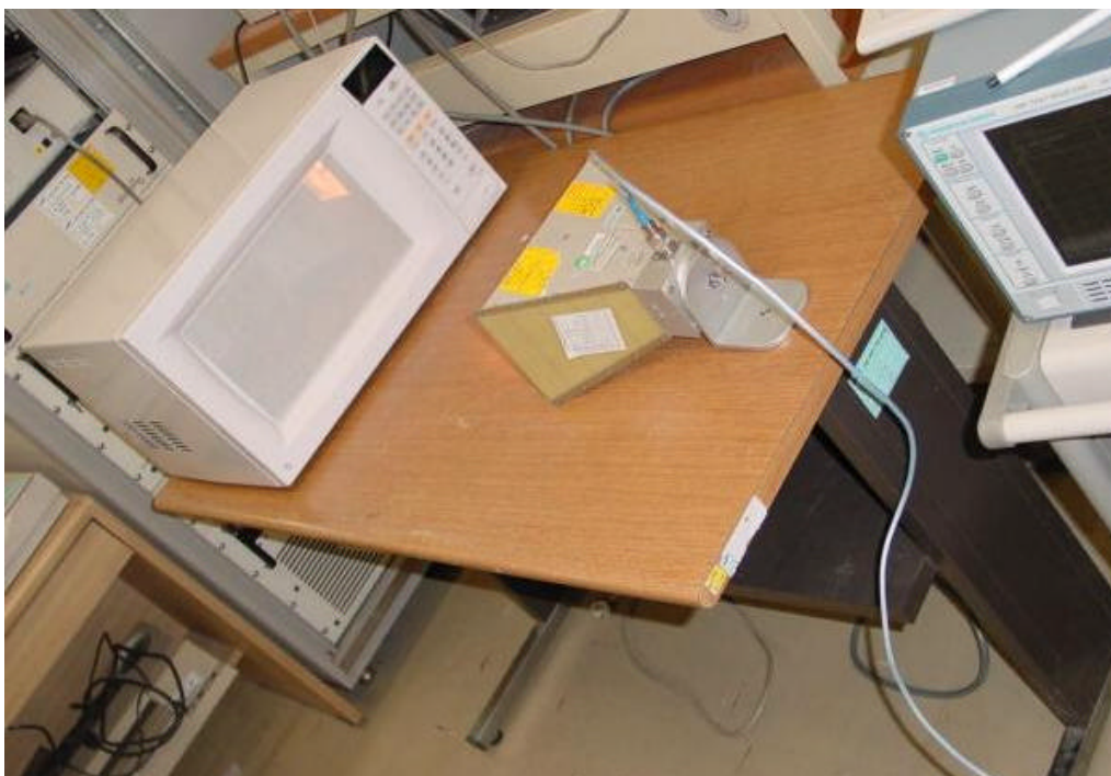
Fig. 5 Test Setup for Operating Frequency Measurements
