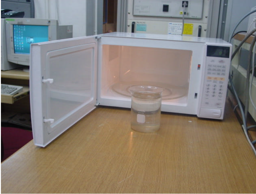
Fig.3 Test Setup for RF output power
