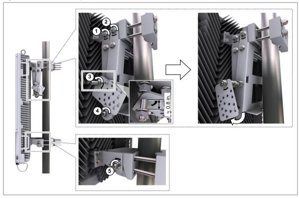
Adjust the down tilt of the MMU with the down tilting holes on the angle plate and place the angle plate on the scissors bracket.
