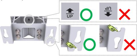
3 Insert the stud bolts into the wall mounting bracket holes and tighten the fasteners temporarily.
