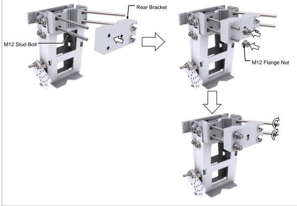
Fixing Bracket Assembly to the MMU
