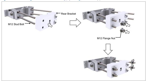
To assemble Scissors Bracket Assembly
