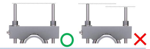
4 Check if the sides of the MMU are vertical using a level.
