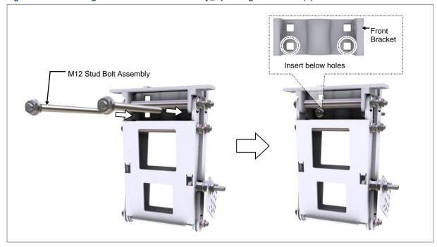
4 Tilt the unit bracket downward, tighten the M12 flange nut. Make sure the unit bracket is vertical when tilting it back to the original position.
