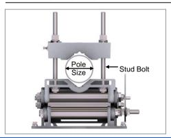
Figure 6. MMU Arrangement\_Wall Type
