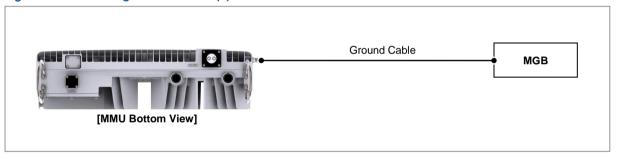
3 Remove the fastener (M6 SEMS) from the MMU ground terminal.
