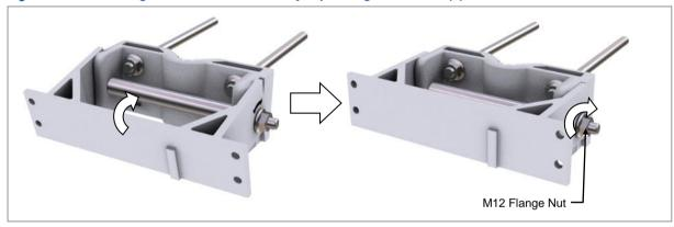
5 Pass the stud bolt assembly through the front bracket holes.
