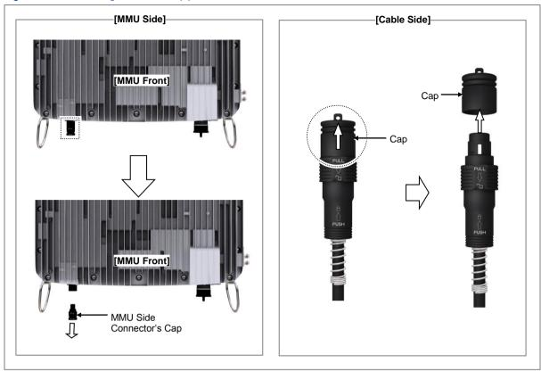
4 Insert the connector aligning the cable side connector's white marking and system side connector's white dot. When inserting the connector, push the shell to upper side.
