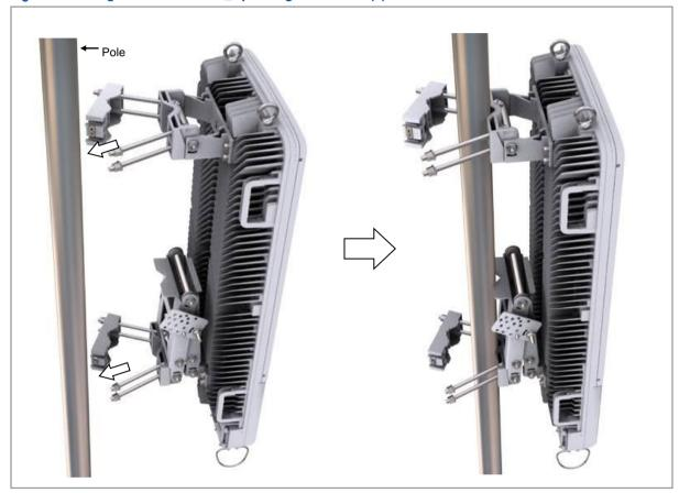
3 Place the stud bolts on the open side holes of the rear brackets at the top and bottom of the back of the MMU, and tighten the fasteners on both sides.
