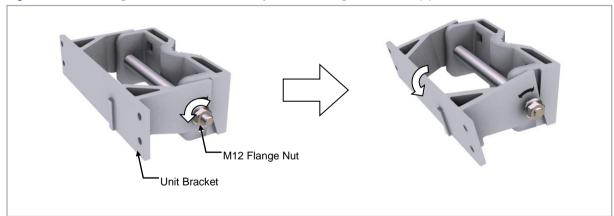
**3** Pass the stud bolt assembly through the front bracket holes.
