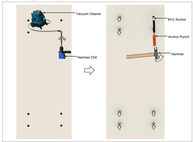
**3** Fix fasteners to anchor bolt temporarily.
