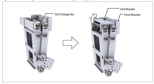
3 Pass the stud bolt assembly through the front bracket holes.
