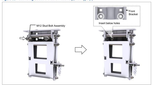
4 Tilt the unit bracket downward, tighten the M12 flange nut. Make sure the unit bracket is vertical when tilting it back to the original position.
