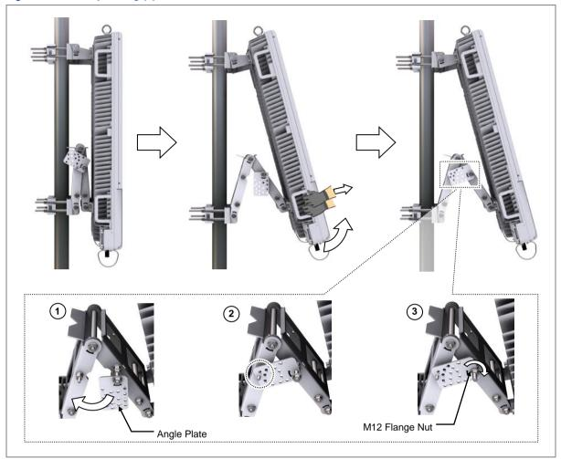
4 Re-tighten the loosened fasteners.
