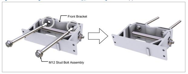
4 Tilt the unit bracket upward, tighten the M12 flange nut. Make sure the unit bracket is vertical when tilting it back to the original position.
