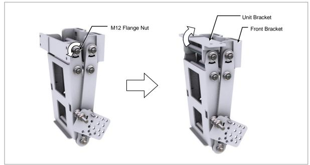
**3** Pass the stud bolt assembly through the front bracket holes.
