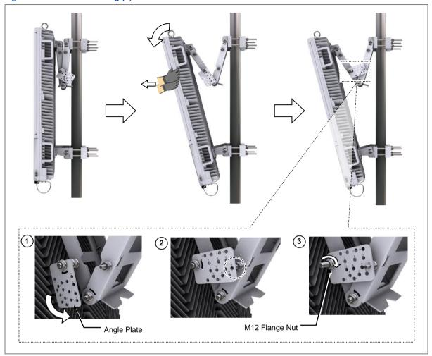
4 Re-tighten the loosened fasteners.
