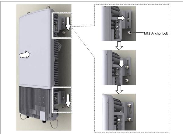
3 Fix MMU using fasteners at the right/left and top/bottom side of it.
