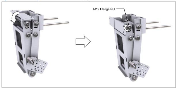
5 Pass the stud bolt assembly through the front bracket holes.
