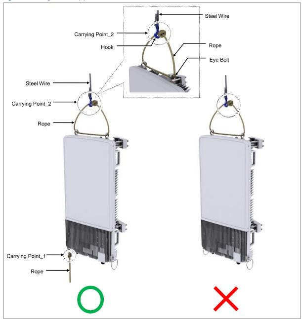
2 Operator A operates the winch to lift the MMU while Operator B pulls the
