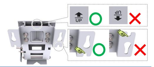
**6** Insert the stud bolts into the rear bracket holes and tighten the fasteners temporarily.
