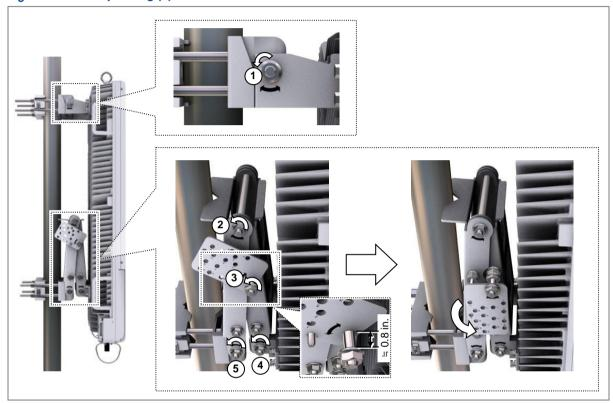
3 Adjust the up tilt of the MMU with the down tilting holes on the angle plate and place the angle plate on the scissors bracket.
