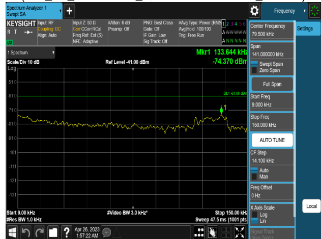
Plot 8-88. Conducted Spurious Emission Plot (9kHz to 150kHz) (n77_2C_100M+100M_QPSK - Mid Channel_Port 31)
