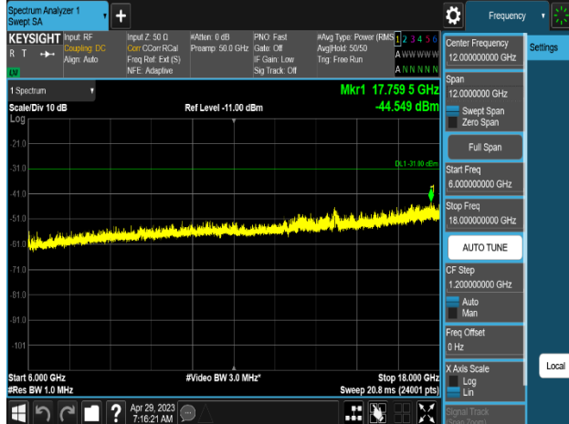
Plot 8-77. Conducted Spurious Emission Plot (6GHz to 18GHz) (n77_1C_100M_QPSK - Low Channel_Port 47)
