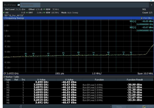
Plot 8-84. Conducted Spurious Emission Plot (3692MHz to 3699MHz) (n77_2C_100M+40M_QPSK - Mid Channel_Port 31)
