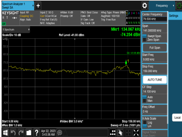
Plot 8-61. Conducted Spurious Emission Plot (9KHz to 150KHz) (n77_1C_80M_QPSK - Low Channel_Port 19)
