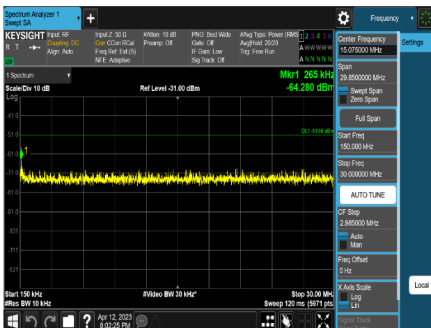
Plot 8-71. Conducted Spurious Emission Plot (150kHz to 30MHz) (n77_1C_100M_QPSK - Low Channel_Port 47)
