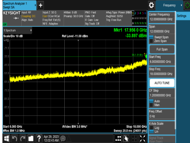
Plot 8-59. Conducted Spurious Emission Plot (6GHz to 18GHz) (n77_1C_60M_QPSK - Low Channel_Port 31)
