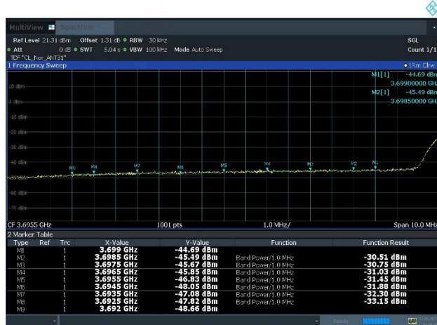
Plot 8-57. Conducted Spurious Emission Plot (3692MHz to 3699MHz) (n77_1C_60M_QPSK - Low Channel_Port 31)
