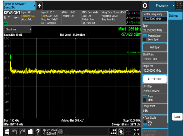
Plot 8-62. Conducted Spurious Emission Plot (150KHz to 30MHz) (n77_1C_80M_QPSK - Low Channel_Port 19)
