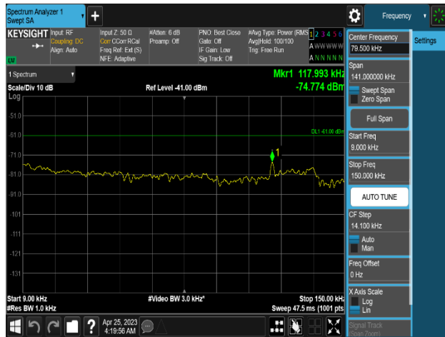
Plot 8-79. Conducted Spurious Emission Plot (9kHz to 150kHz) (n77_2C_100M+40M_QPSK - Mid Channel_Port 31)
