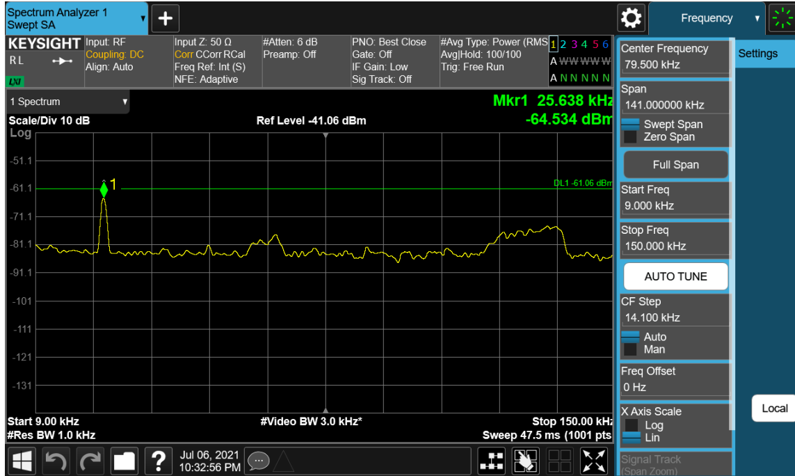
Plot 7-147. Conducted Spurious Emission Plot 9 kHz to 150 kHz (Multi-RAT LTE 3C_20M+20M+20M & NR 1C_100M_Contiguous - High Channel_Port 56)
