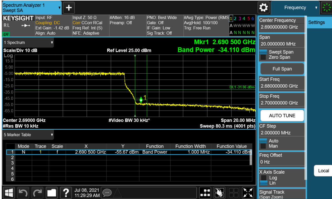
Plot 7-103. Band Edge Emission (2690MHz to 2691MHz) Plot (Multi-RAT LTE 3C_20M+20M+20M & NR 1C_100M_Non-Contiguous - High Channel_Port 63)
