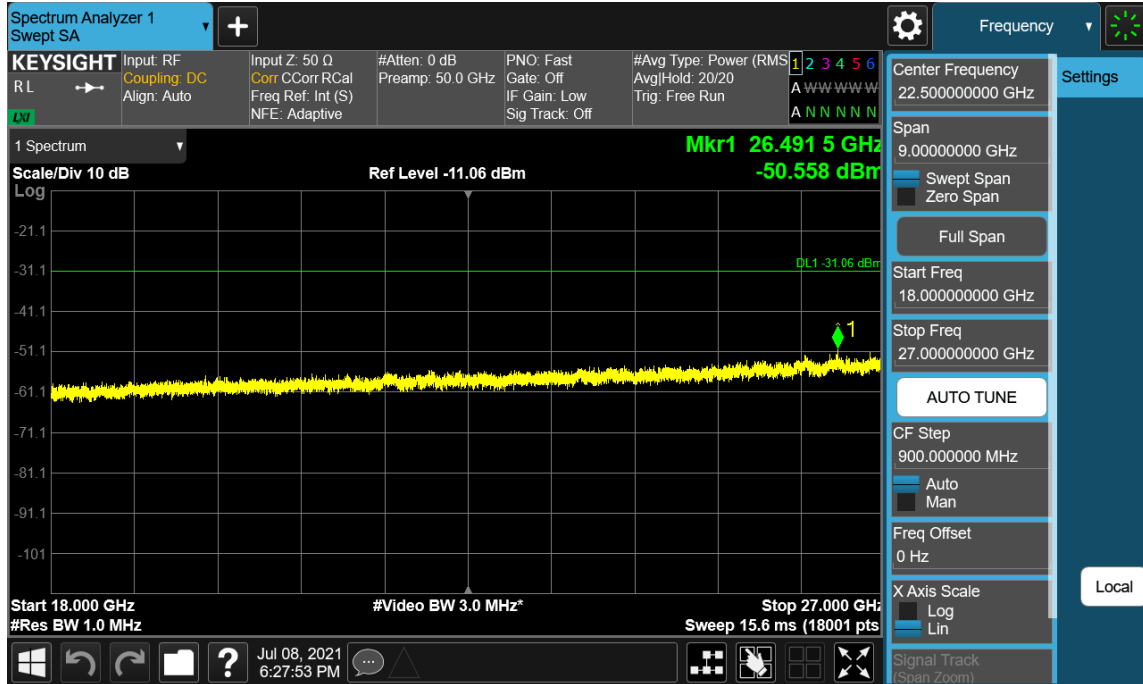
Plot 7-132. Conducted Spurious Emission Plot 18 GHz to 27 GHz (Multi-RAT LTE 3C_20M+20M+20M & NR 1C_80M_Non-contiguous - Port 41)
