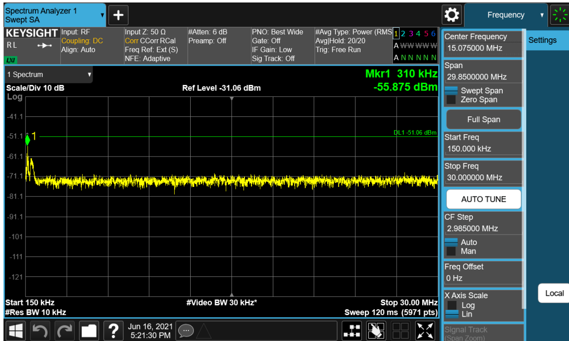
Plot 7-113. Conducted Spurious Emission Plot 150 kHz to 30 MHz (Multi-RAT LTE 3C_20M+20M+20M & NR 1C_80M_Contiguous - Middle Channel_Port 49)
