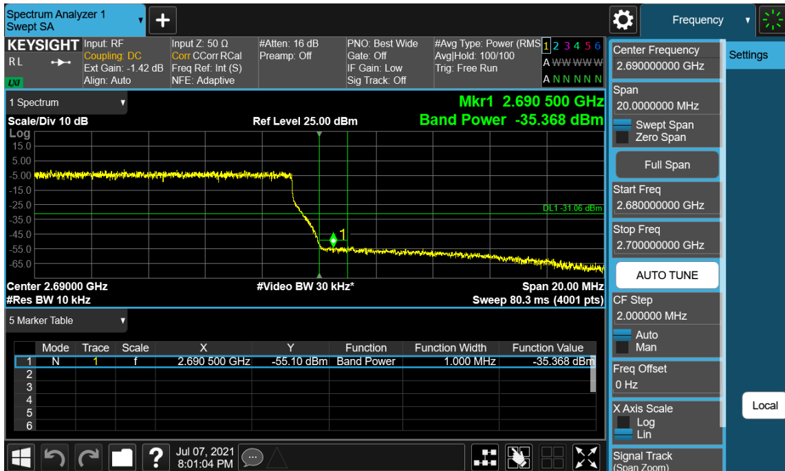
Plot 7-91. Band Edge Emission (2690MHz to 2691MHz) Plot (Multi-RAT LTE 3C_20M+20M+20M & NR 1C_80M_Contiguous - High Channel_Port 36)
