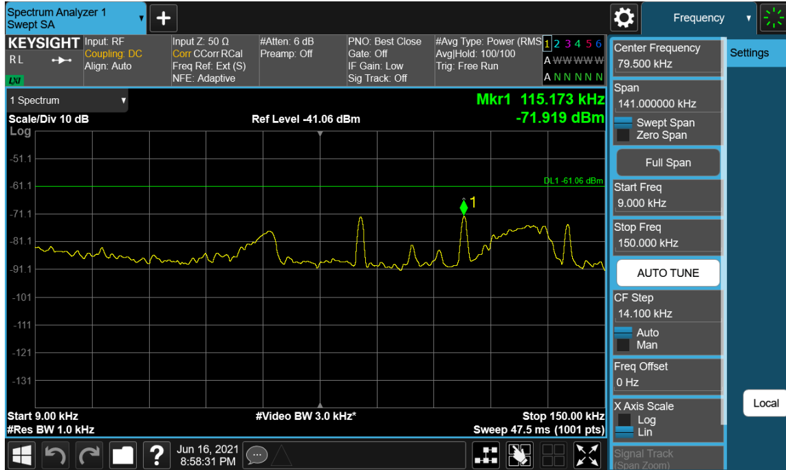
Plot 7-119. Conducted Spurious Emission Plot 9 kHz to 150 kHz (Multi-RAT LTE 3C_20M+20M+20M & NR 1C_80M_Contiguous - High Channel_Port 16)
