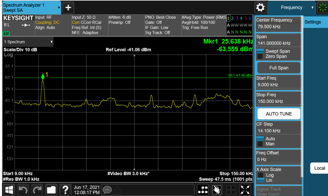
Plot 7-126. Conducted Spurious Emission Plot 9 kHz to 150 kHz (Multi-RAT LTE 3C_20M+20M+20M & NR 1C_80M_Non-contiguous - Port 48)
