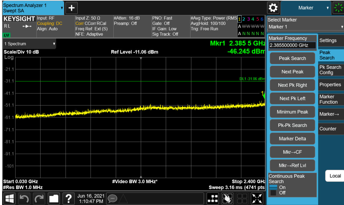
Plot 7-107. Conducted Spurious Emission Plot 30 MHz to 2400 MHz (Multi-RAT LTE 3C_20M+20M+20M & NR 1C_80M_Contiguous - Low Channel_Port 53)
