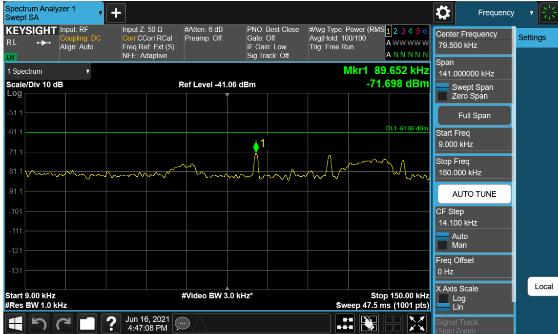
Plot 7-112. Conducted Spurious Emission Plot 9 kHz to 150 kHz (Multi-RAT LTE 3C_20M+20M+20M & NR 1C_80M_Contiguous - Middle Channel_Port 27)
