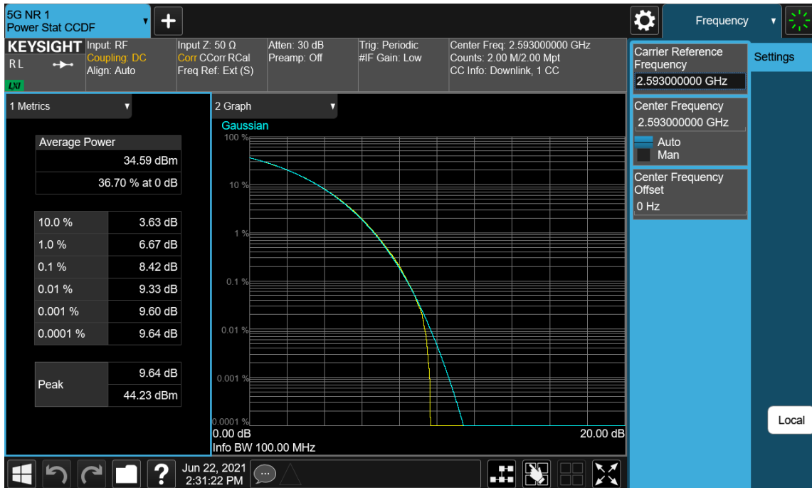
Plot 7-73. Peak To Average Power Ratio Plot (NR 1C_100M - Middle Channel_QPSK_Port 42)
