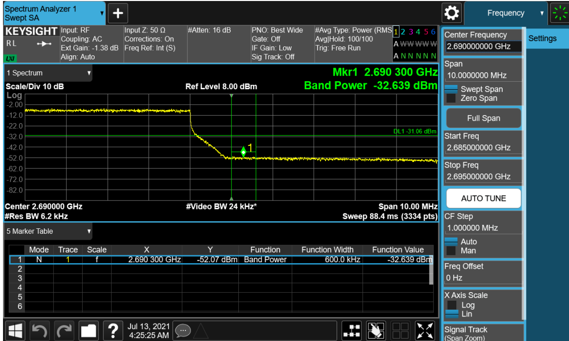
Plot 7-79. Band Edge Emission (2690MHz to 2691MHz) Plot (LTE 3C_20M+20M+20M - High Channel_QPSK_Port 0)
