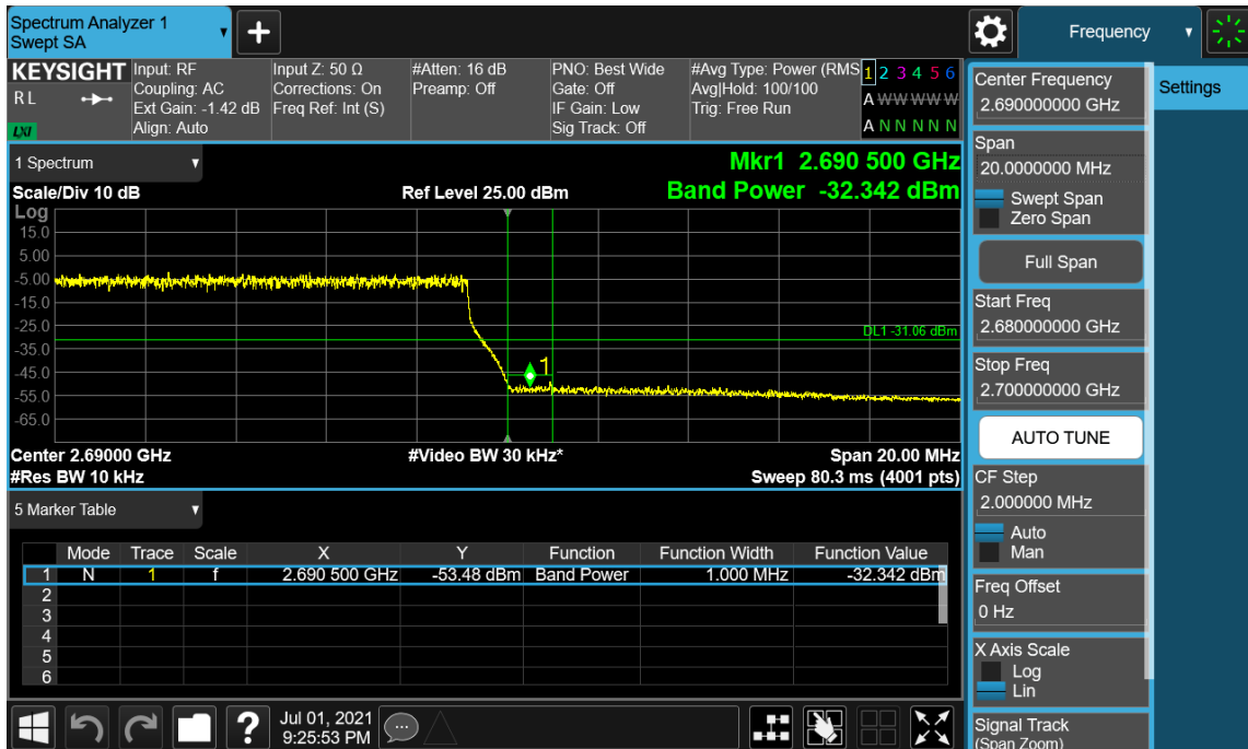
Plot 7-87. Band Edge Emission (2690MHz to 2691MHz) Plot (NR 1C_100M - High Channel_256QAM_Port 0)
