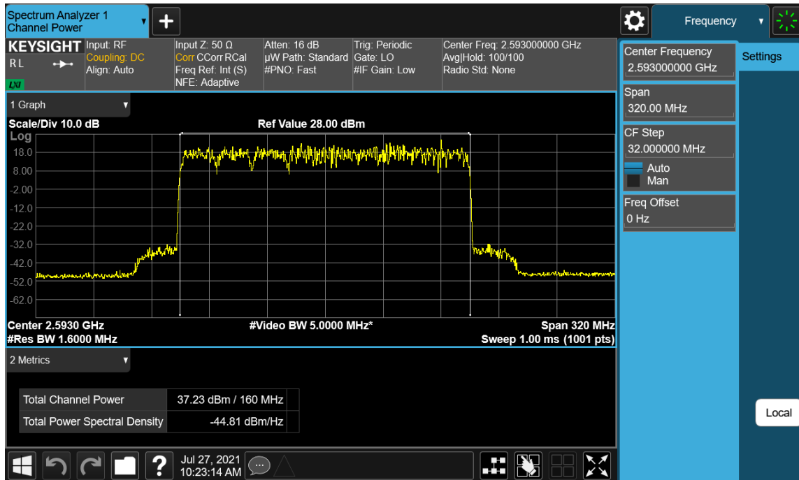
Plot 7-61. Conducted Average Output Power Plot (Multi-RAT LTE 3C_20M+20M+20M & NR 1C_100M - QPSK, Port 47)
