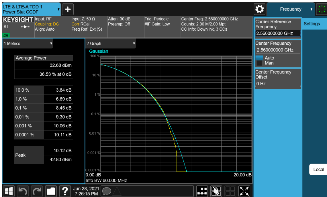
Plot 7-66. Peak To Average Power Ratio Plot (LTE 3C_20M+20M+20M - Middle Channel_16QAM_Port 38)
