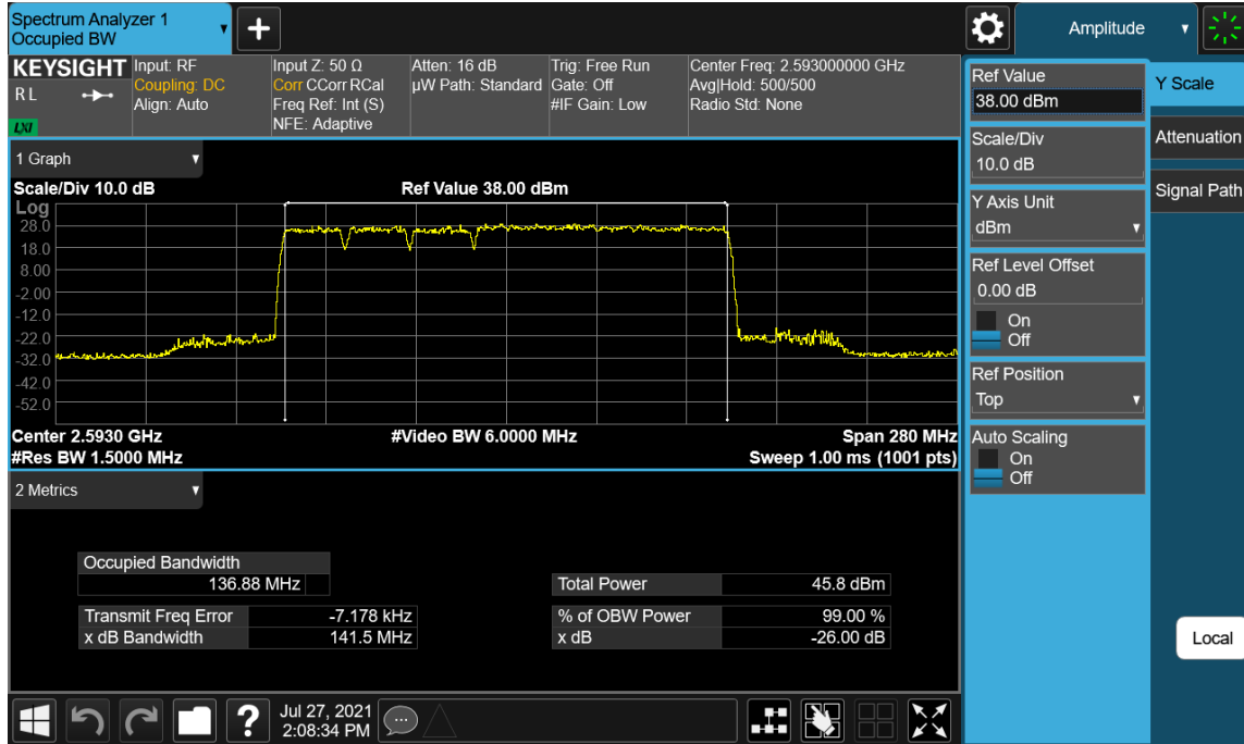
Plot 7-13. Occupied Bandwidth Plot (Multi-RAT LTE 3C_20M+20M+20M & NR 1C_80M - QPSK_Port 4)
