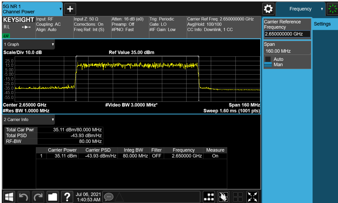
Plot 7-44. Conducted Average Output Power Plot (NR 1C_80M - High Channel_256QAM, Port 36)
