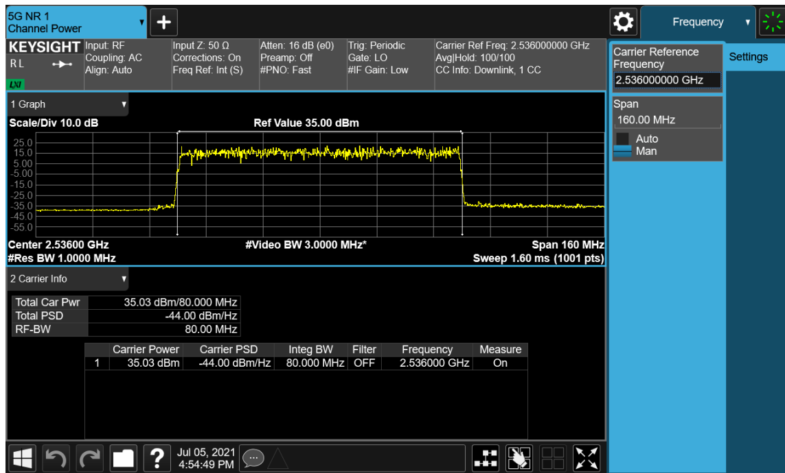
Plot 7-36. Conducted Average Output Power Plot (NR 1C_80M - Low Channel_256QAM, Port 47)
