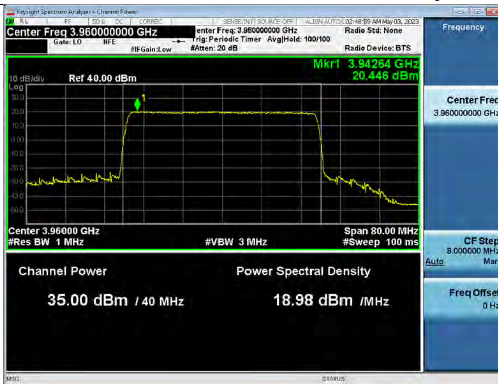
Antenna 19 / (64 Port) 5G NR n77 40 MHz [1 Carrier] / 256QAM / High
