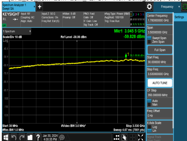
Plot 8-86. Conducted Spurious Emission Plot 30 MHz to 3.53 GHz (NR_1C_20M_16QAM - High Channel, Port 57)
