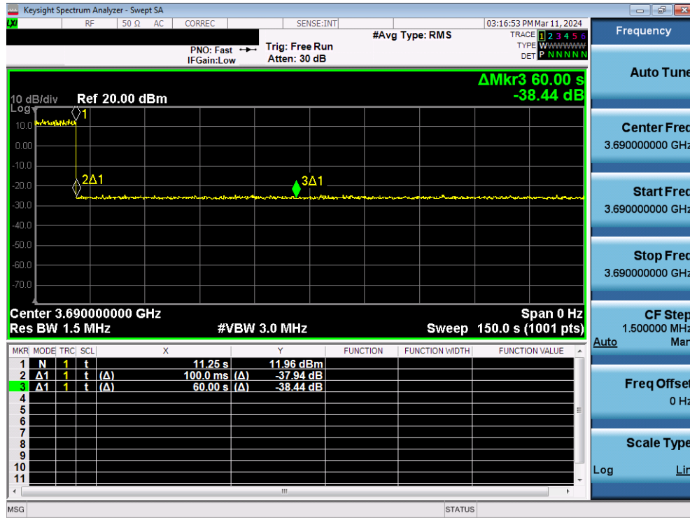
Plot 12. Conducted Measurement – RF transmission stops within 60s of SAS heartbeat response (Marker 1) (WINNF.FT.C.HBT.4)
