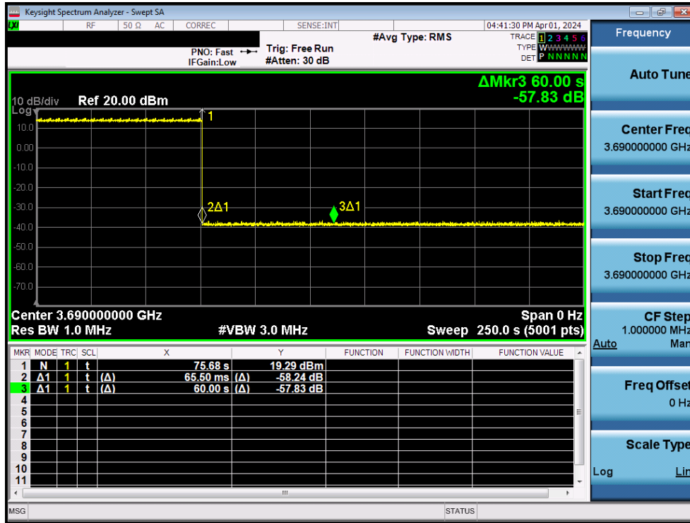
Plot 17. Conducted Measurement - RF transmission stops within 60s of SAS heartbeat response (Marker 1) (WINNF.FT.C.HBT.10)
