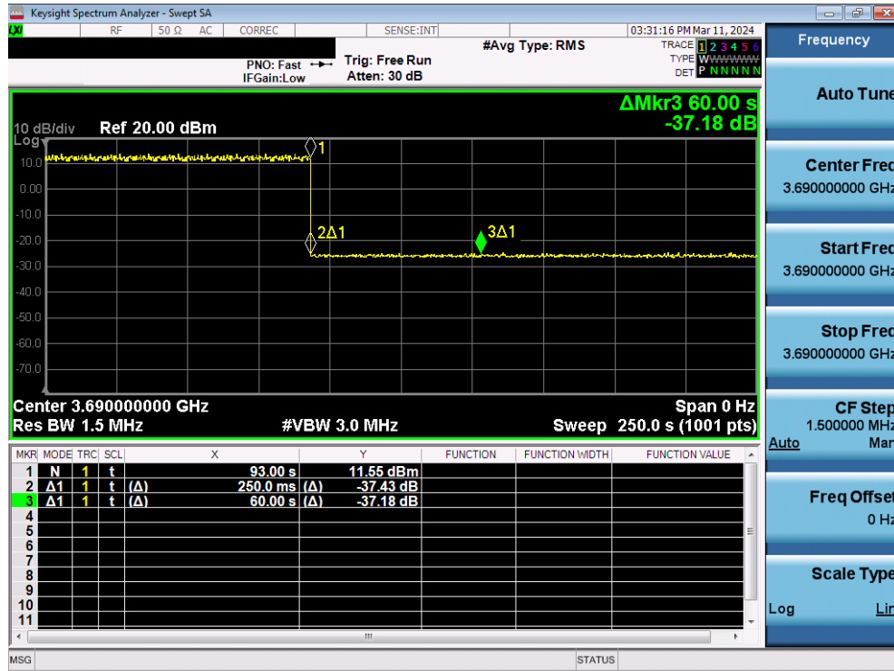
Plot 15. Conducted Measurement – RF transmission stops within 60s of SAS heartbeat response (Marker 1) (WINNF.FT.C.HBT.7)
