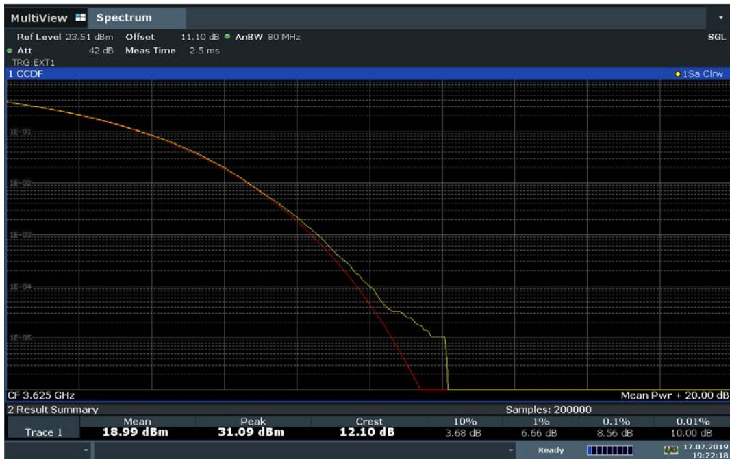
Plot 7-111. 16 User Beam PAR Plot (50.0MHz Total Bandwidth 256QAM - Mid Channel-SISO)
