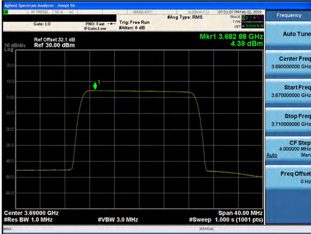
Plot 7-385. Peak Power Spectral Density Plot (1CC– 3690 MHz- 20.0MHz 256QAM- High Channel) Port 07
