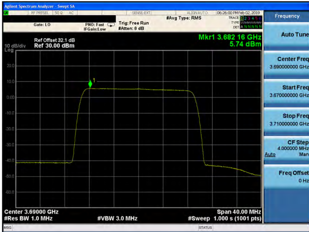
Plot 7-399. Peak Power Spectral Density Plot (1CC- 3690 MHz- 20.0MHz 256QAM- High Channel) Port 26
