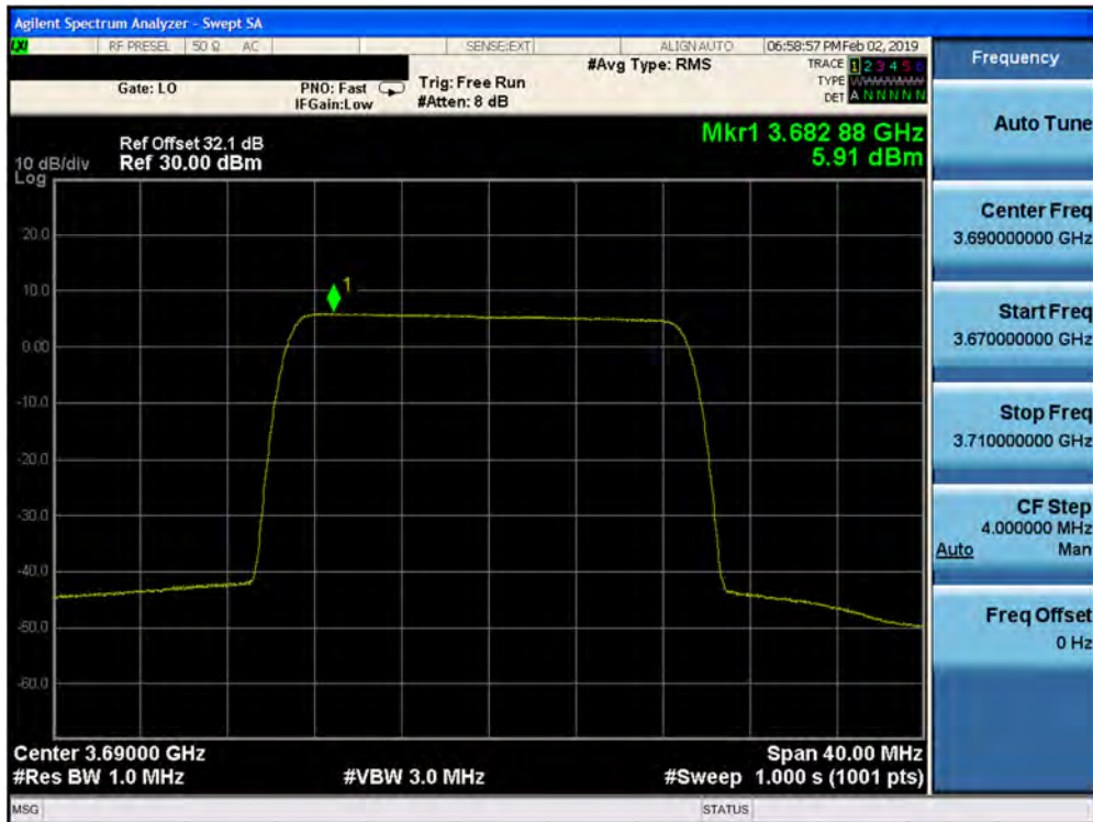
Plot 7-384. Peak Power Spectral Density Plot (1CC– 3690 MHz- 20.0MHz 256QAM- High Channel) Port 19
