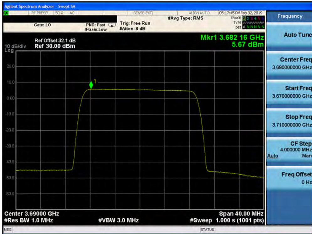
Plot 7-391. Peak Power Spectral Density Plot (1CC– 3690 MHz- 20.0MHz 256QAM- High Channel) Port 22
