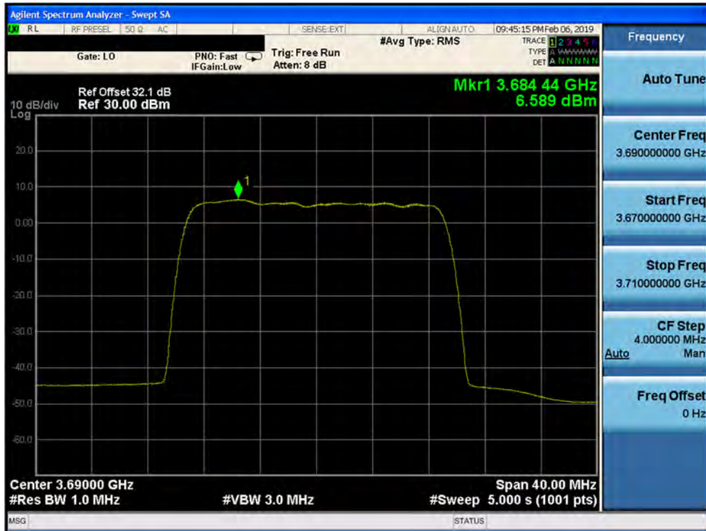
Plot 7-343. Peak Power Spectral Density Plot (1CC– 3690 MHz- 20.0MHz 16QAM- High Channel) Port 30
