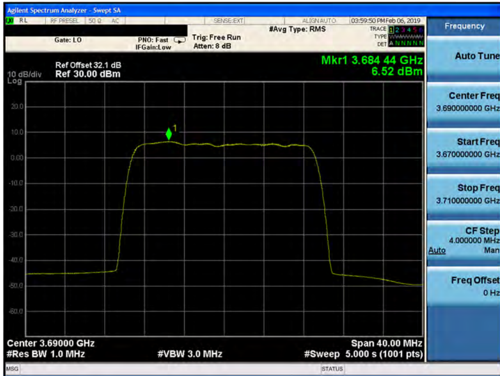
Plot 7-325. Peak Power Spectral Density Plot (1CC– 3690 MHz- 20.0MHz 16QAM- High Channel) Port 20
