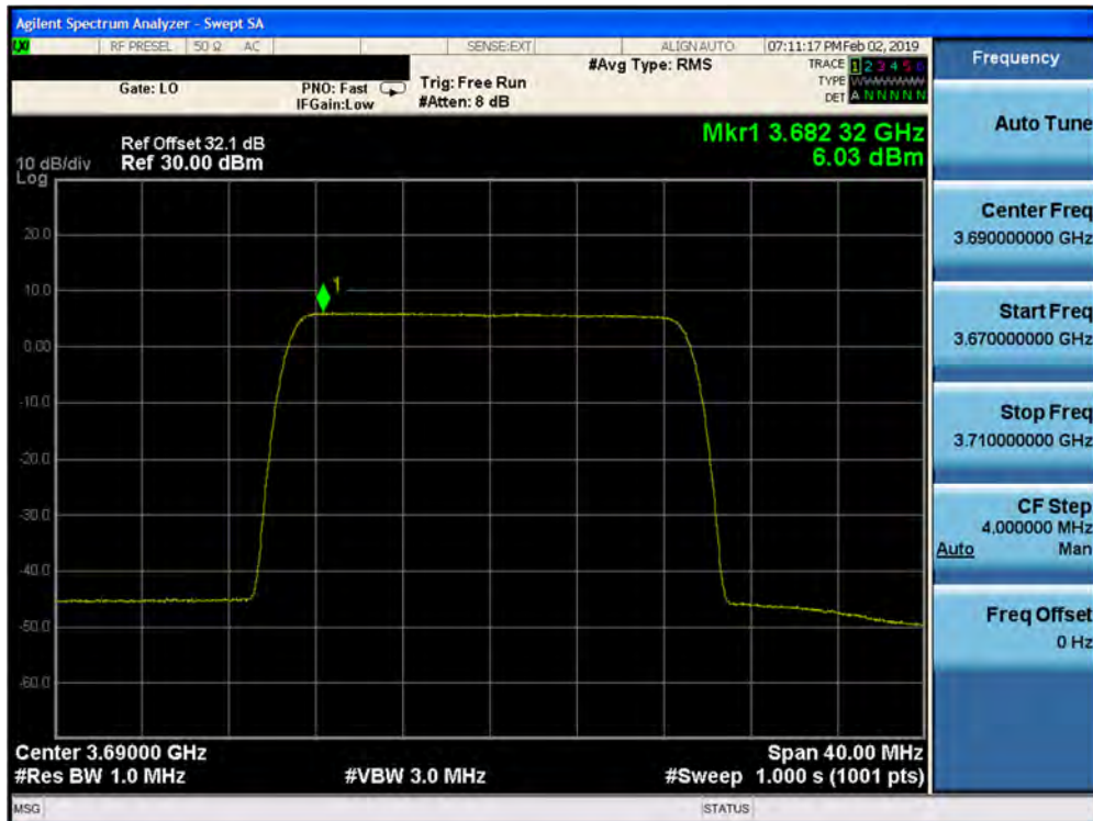
Plot 7-360. Peak Power Spectral Density Plot (1CC- 3690 MHz- 20.0MHz 64QAM- High Channel) Port 23
