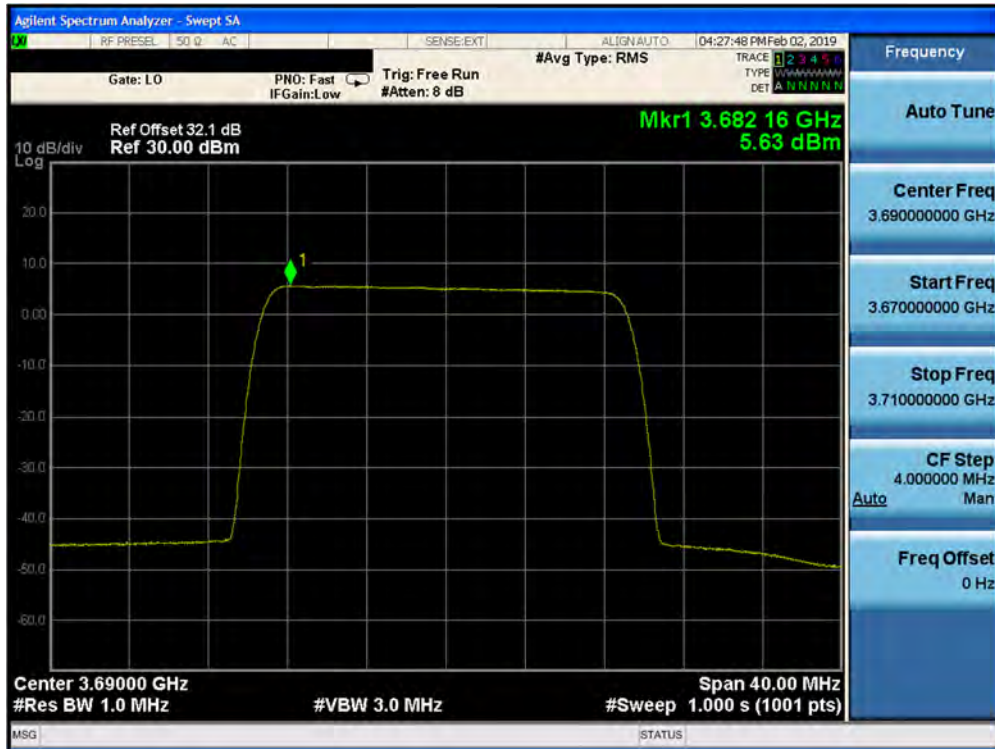
Plot 7-403. Peak Power Spectral Density Plot (1CC– 3690 MHz- 20.0MHz 256QAM- High Channel) Port 13
