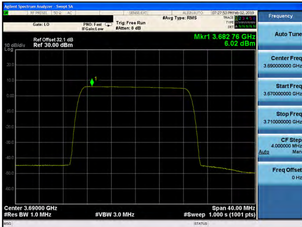
Plot 7-312. Peak Power Spectral Density Plot (1CC– 3690 MHz- 20.0MHz QPSK- High Channel) Port 31
