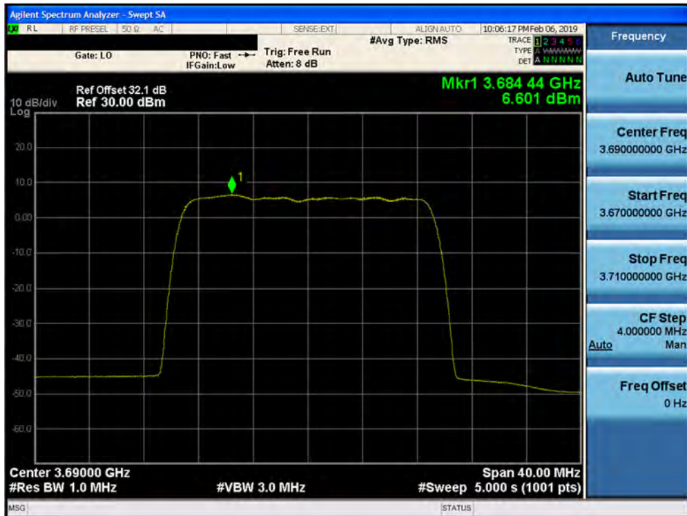
Plot 7-344. Peak Power Spectral Density Plot (1CC– 3690 MHz- 20.0MHz 16QAM- High Channel) Port 31
