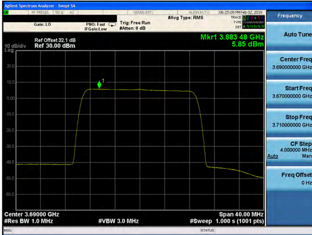
Plot 7-367. Peak Power Spectral Density Plot (1CC- 3690 MHz- 20.0MHz 64QAM- High Channel) Port 26
