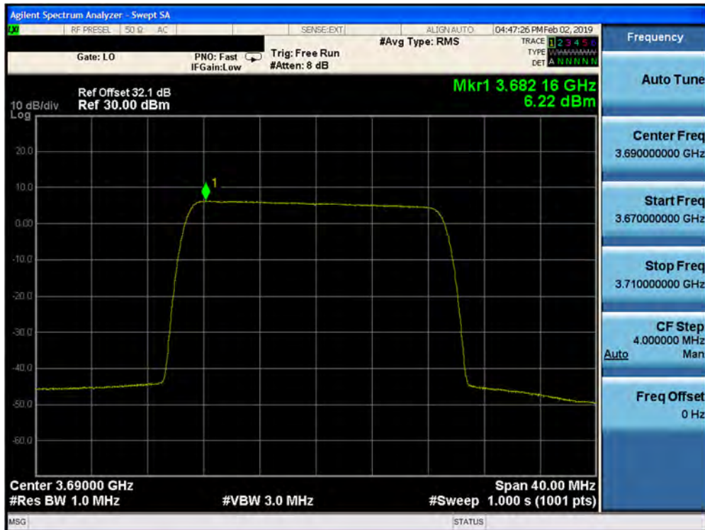
Plot 7-382. Peak Power Spectral Density Plot (1CC– 3690 MHz- 20.0MHz 256QAM- High Channel) Port 17
