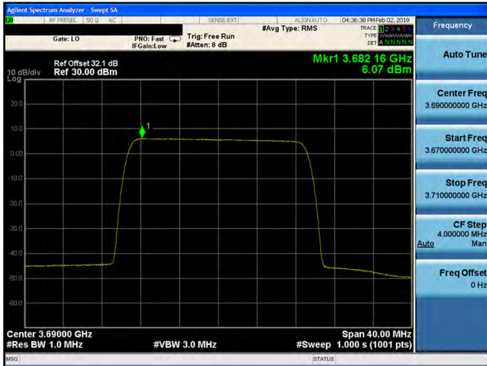
Plot 7-395. Peak Power Spectral Density Plot (1CC– 3690 MHz- 20.0MHz 256QAM- High Channel) Port 09
