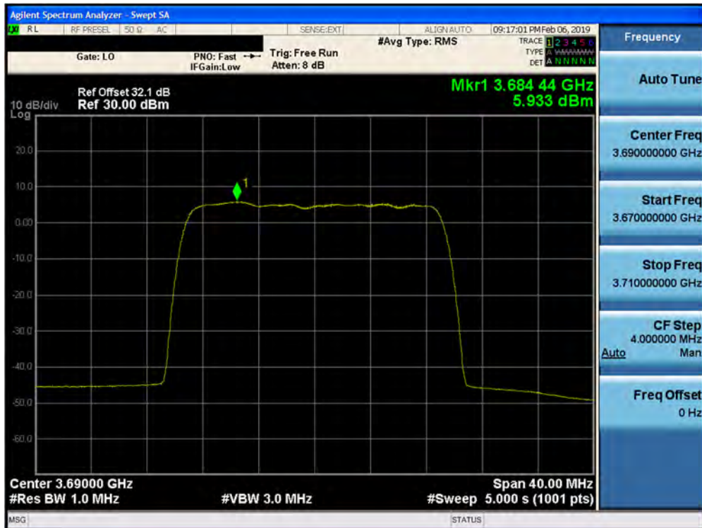
Plot 7-334. Peak Power Spectral Density Plot (1CC- 3690 MHz- 20.0MHz 16QAM- High Channel) Port 25
