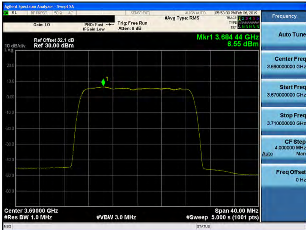
Plot 7-326. Peak Power Spectral Density Plot (1CC– 3690 MHz- 20.0MHz 16QAM- High Channel) Port 21
