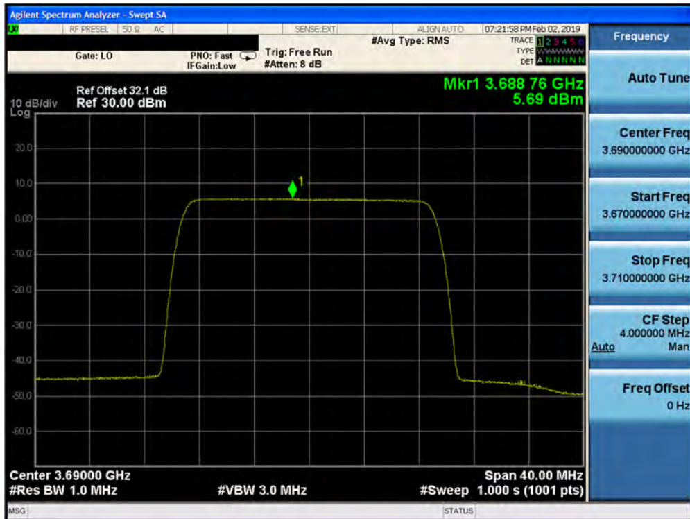
Plot 7-400. Peak Power Spectral Density Plot (1CC- 3690 MHz- 20.0MHz 256QAM- High Channel) Port 27
