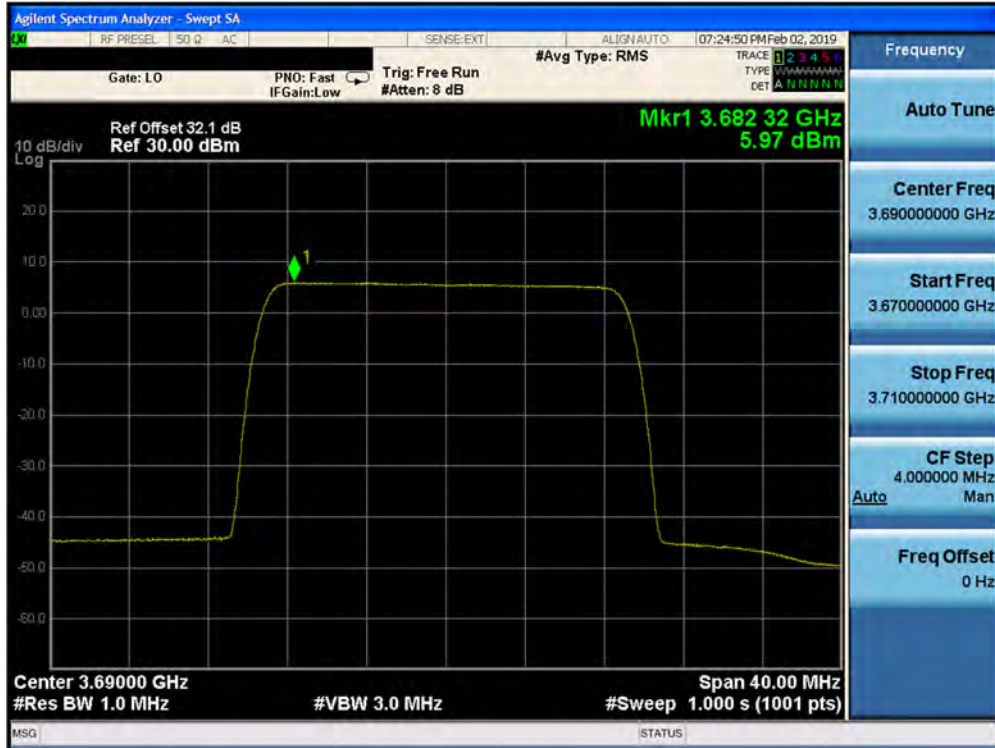
Plot 7-369. Peak Power Spectral Density Plot (1CC– 3690 MHz- 20.0MHz 64QAM- High Channel) Port 15
