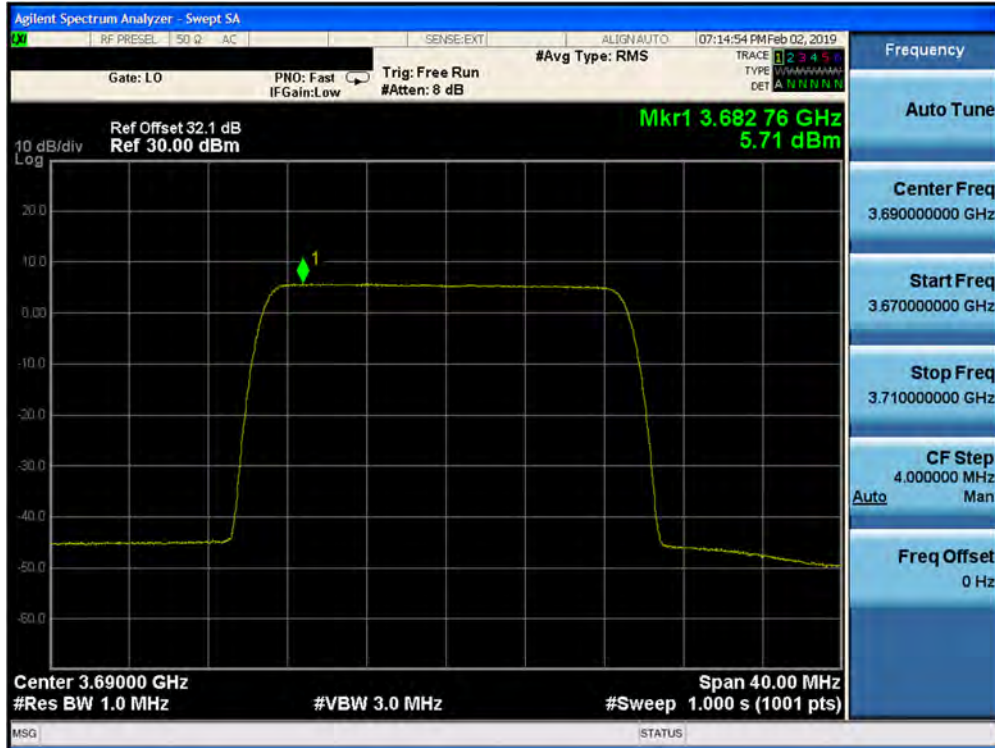
Plot 7-361. Peak Power Spectral Density Plot (1CC- 3690 MHz- 20.0MHz 64QAM- High Channel) Port 11
