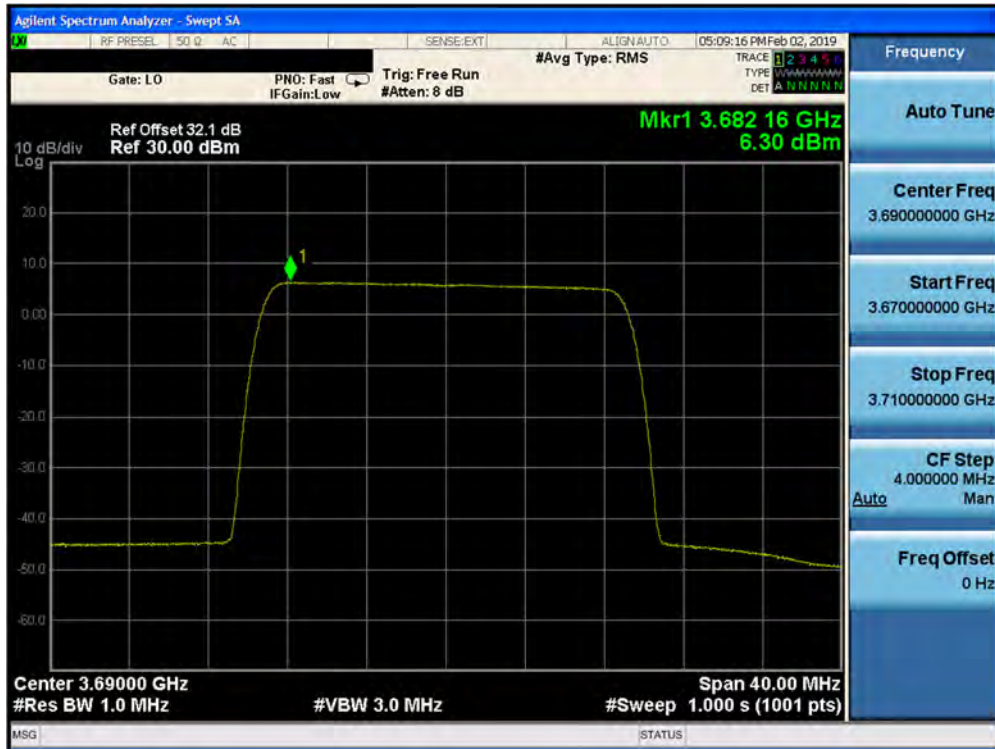
Plot 7-383. Peak Power Spectral Density Plot (1CC– 3690 MHz- 20.0MHz 256QAM- High Channel) Port 18
