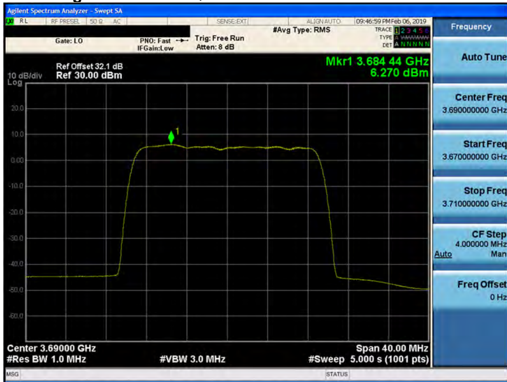
Plot 7-313. Peak Power Spectral Density Plot (1CC– 3690 MHz- 20.0MHz 16QAM- High Channel) Port 03
