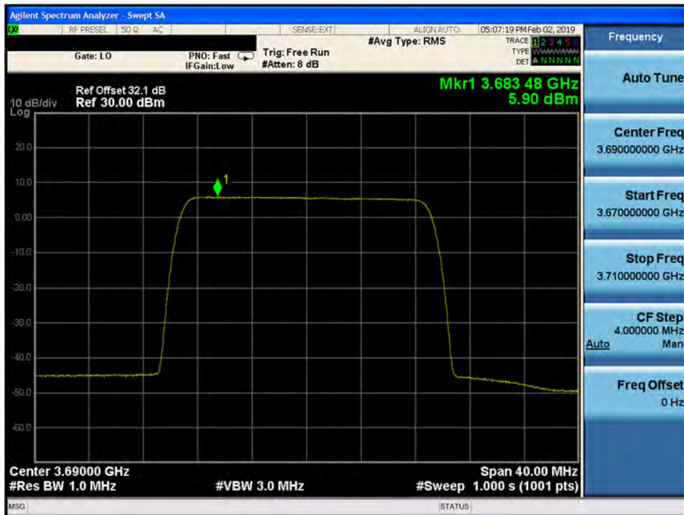
Plot 7-346. Peak Power Spectral Density Plot (1CC– 3690 MHz- 20.0MHz 64QAM- High Channel) Port 02
