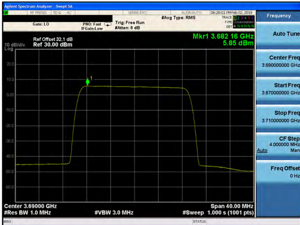
Plot 7-402. Peak Power Spectral Density Plot (1CC– 3690 MHz- 20.0MHz 256QAM- High Channel) Port 14
