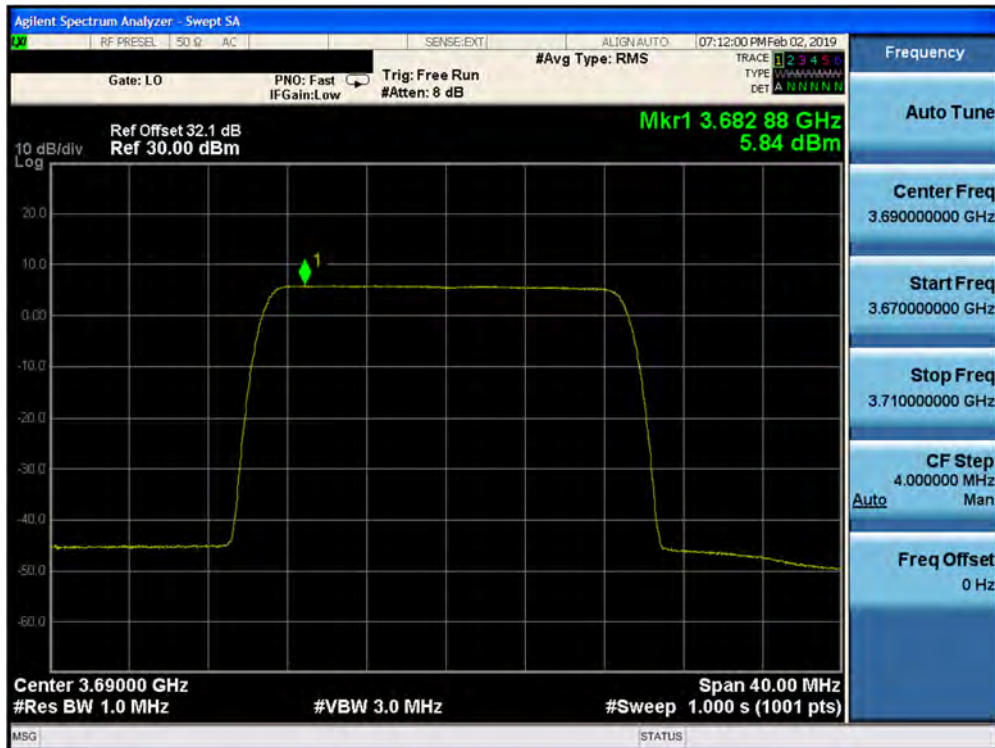
Plot 7-392. Peak Power Spectral Density Plot (1CC– 3690 MHz- 20.0MHz 256QAM- High Channel) Port 23
