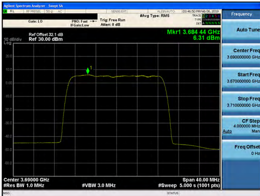
Plot 7-316. Peak Power Spectral Density Plot (1CC– 3690 MHz- 20.0MHz 16QAM- High Channel) Port 00
