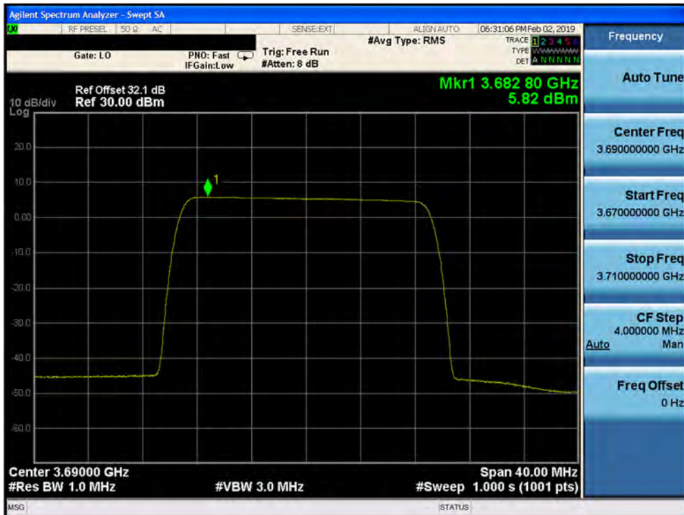
Plot 7-306. Peak Power Spectral Density Plot (1CC– 3690 MHz- 20.0MHz QPSK- High Channel) Port 14
