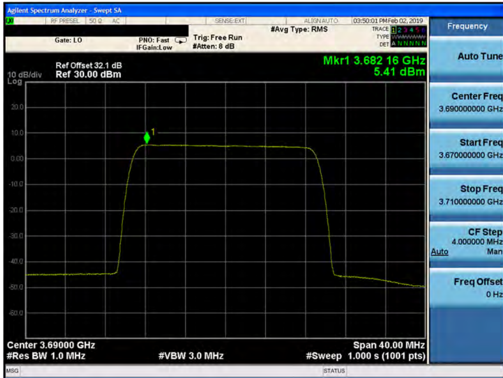
Plot 7-381. Peak Power Spectral Density Plot (1CC– 3690 MHz- 20.0MHz 256QAM- High Channel) Port 16
