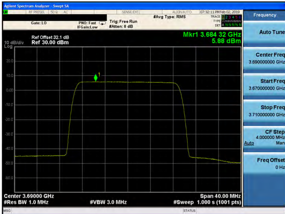
Plot 7-408. Peak Power Spectral Density Plot (1CC– 3690 MHz- 20.0MHz 256QAM- High Channel) Port 31
