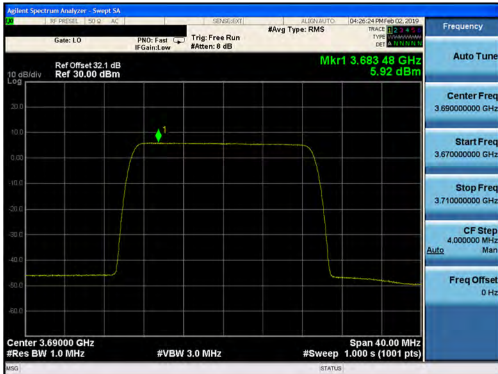
Plot 7-374. Peak Power Spectral Density Plot (1CC– 3690 MHz- 20.0MHz 64QAM- High Channel) Port 29
