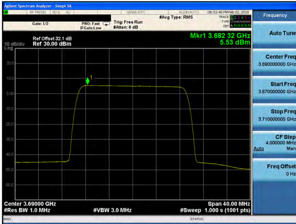
Plot 7-345. Peak Power Spectral Density Plot (1CC– 3690 MHz- 20.0MHz 64QAM- High Channel) Port 03
