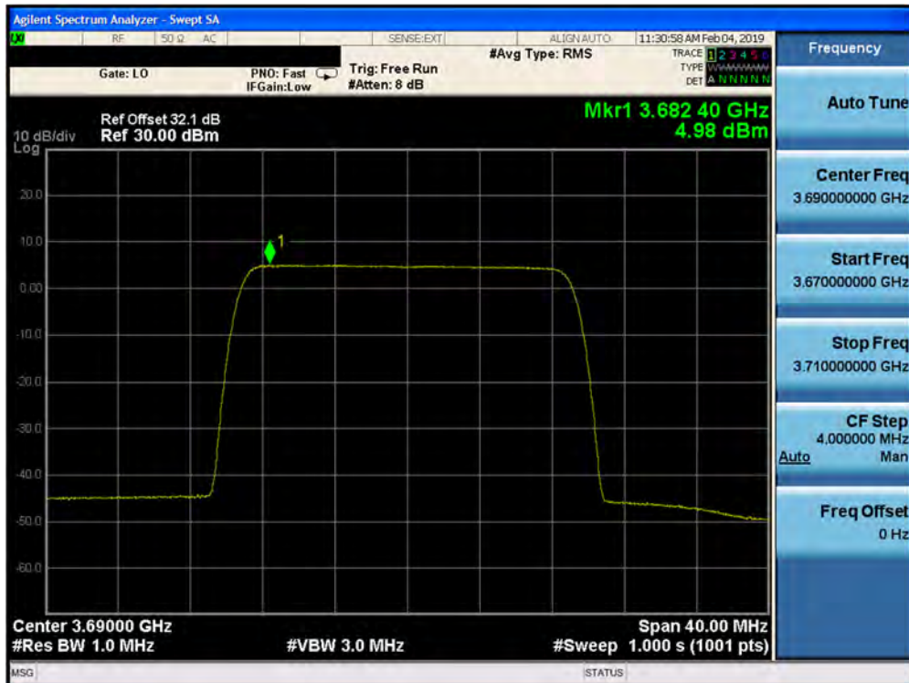
Plot 7-362. Peak Power Spectral Density Plot (1CC- 3690 MHz- 20.0MHz 64QAM- High Channel) Port 10
