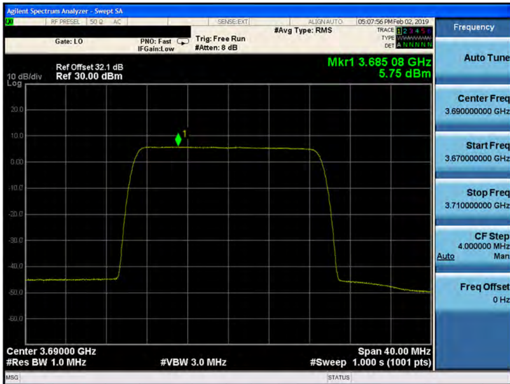
Plot 7-378. Peak Power Spectral Density Plot (1CC– 3690 MHz- 20.0MHz 256QAM- High Channel) Port 02
