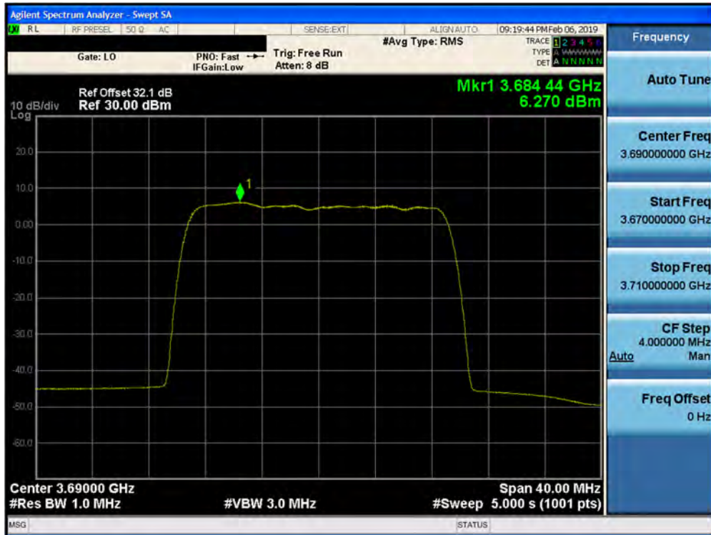
Plot 7-339. Peak Power Spectral Density Plot (1CC- 3690 MHz- 20.0MHz 16QAM- High Channel) Port 13
