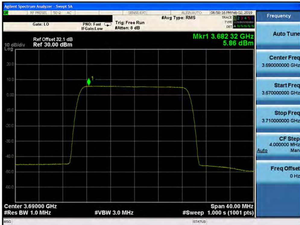
Plot 7-352. Peak Power Spectral Density Plot (1CC- 3690 MHz- 20.0MHz 64QAM- High Channel) Port 19
