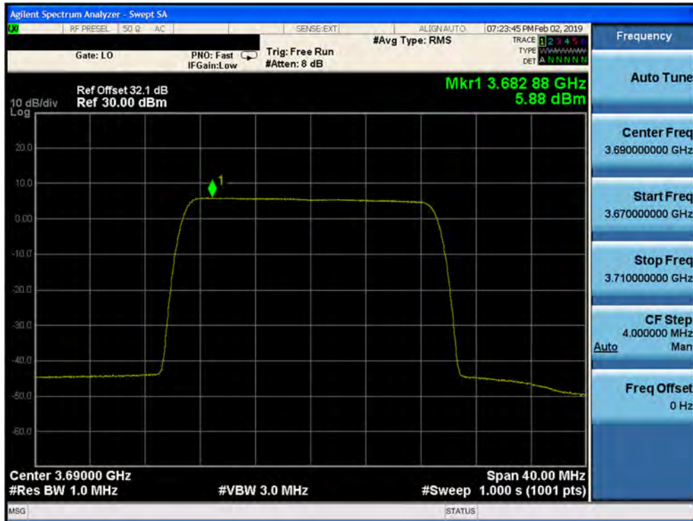
Plot 7-401. Peak Power Spectral Density Plot (1CC– 3690 MHz- 20.0MHz 256QAM- High Channel) Port 15
