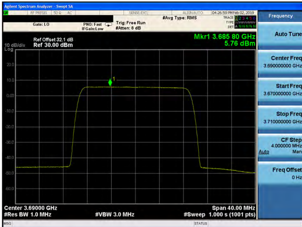
Plot 7-406. Peak Power Spectral Density Plot (1CC– 3690 MHz- 20.0MHz 256QAM- High Channel) Port 29
