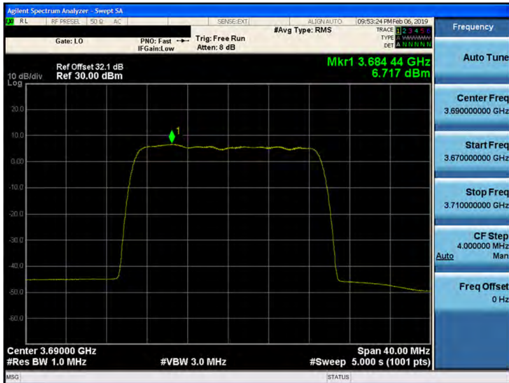
Plot 7-328. Peak Power Spectral Density Plot (1CC- 3690 MHz- 20.0MHz 16QAM- High Channel) Port 23
