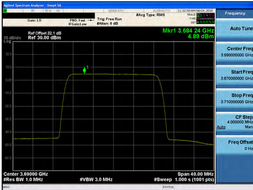
Plot 7-394. Peak Power Spectral Density Plot (1CC– 3690 MHz- 20.0MHz 256QAM- High Channel) Port 10
