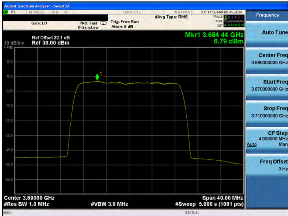
Plot 7-340. Peak Power Spectral Density Plot (1CC- 3690 MHz- 20.0MHz 16QAM- High Channel) Port 12
