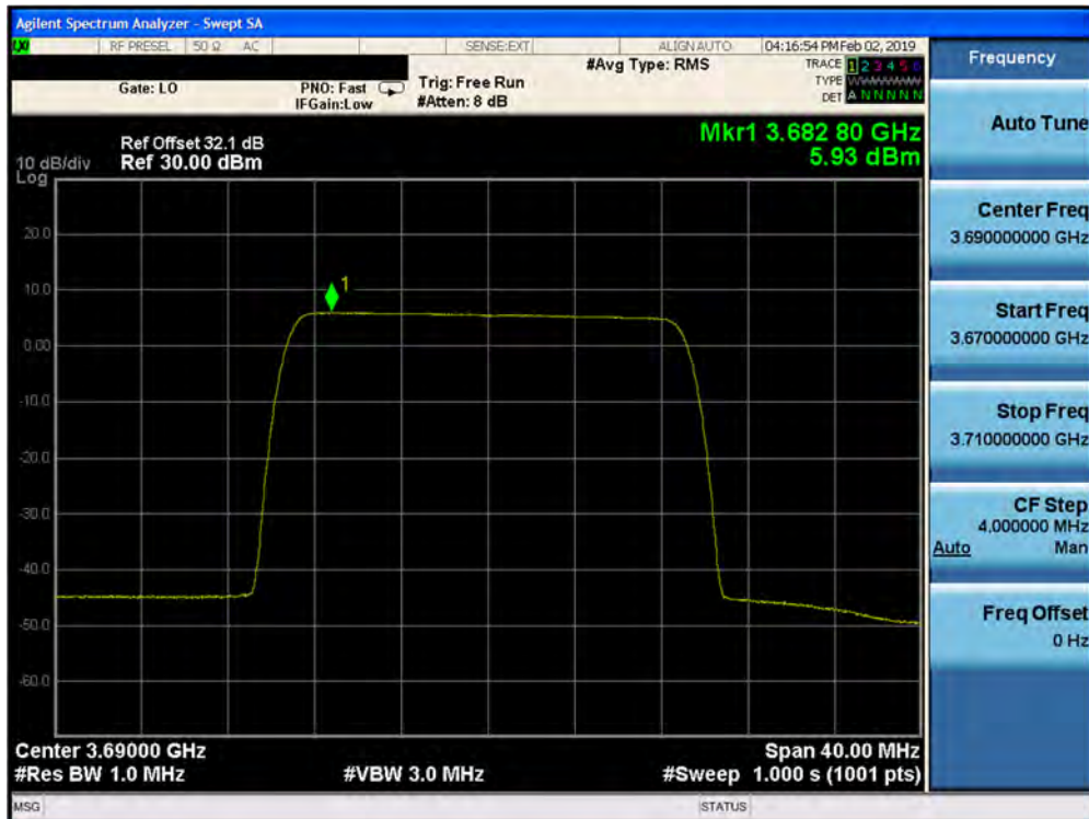
Plot 7-308. Peak Power Spectral Density Plot (1CC– 3690 MHz- 20.0MHz QPSK- High Channel) Port 12
