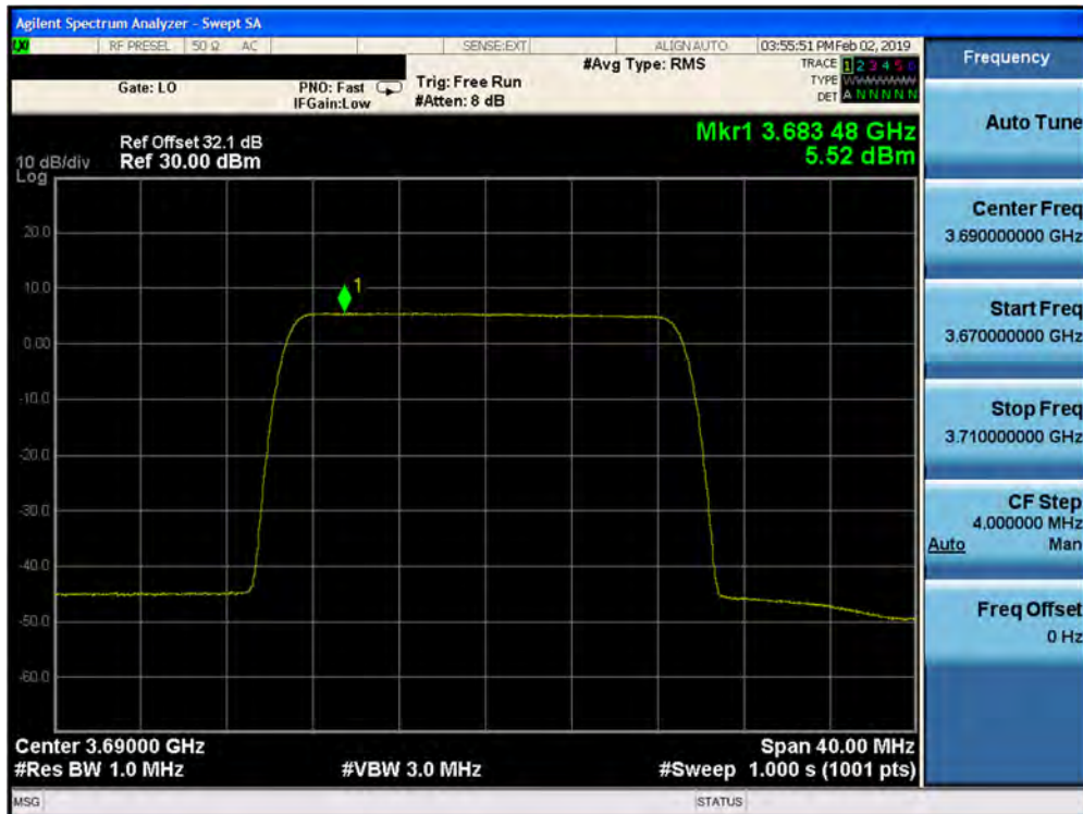
Plot 7-356. Peak Power Spectral Density Plot (1CC- 3690 MHz- 20.0MHz 64QAM- High Channel) Port 04
