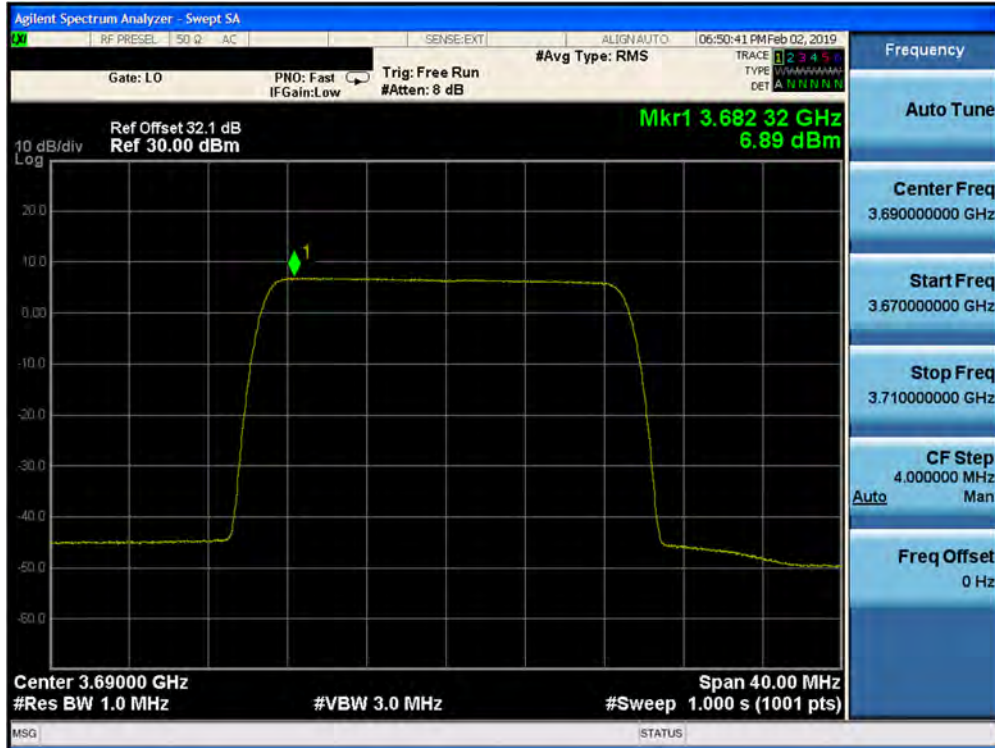
Plot 7-375. Peak Power Spectral Density Plot (1CC- 3690 MHz- 20.0MHz 64QAM- High Channel) Port 30
