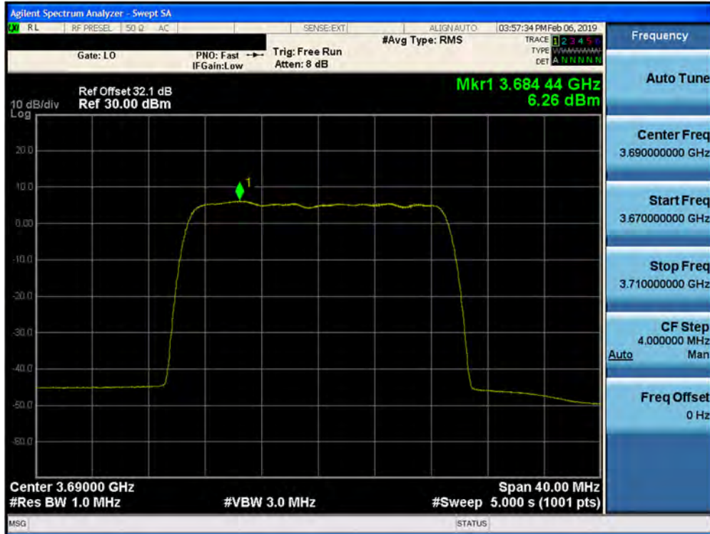
Plot 7-317. Peak Power Spectral Density Plot (1CC- 3690 MHz- 20.0MHz 16QAM- High Channel) Port 16
