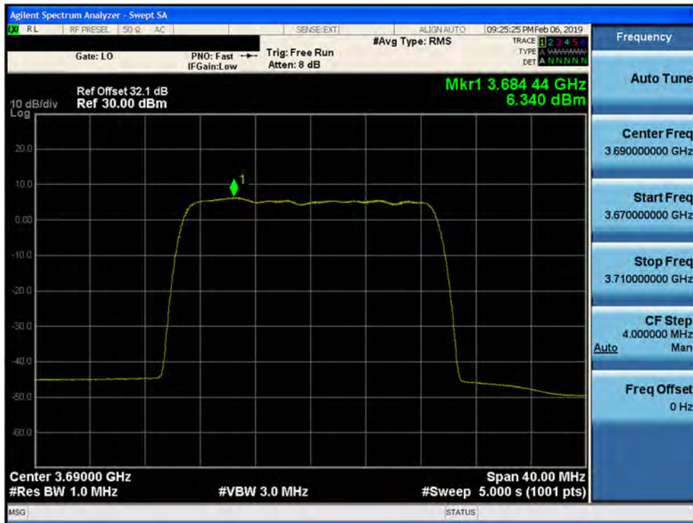
Plot 7-314. Peak Power Spectral Density Plot (1CC– 3690 MHz- 20.0MHz 16QAM- High Channel) Port 02
