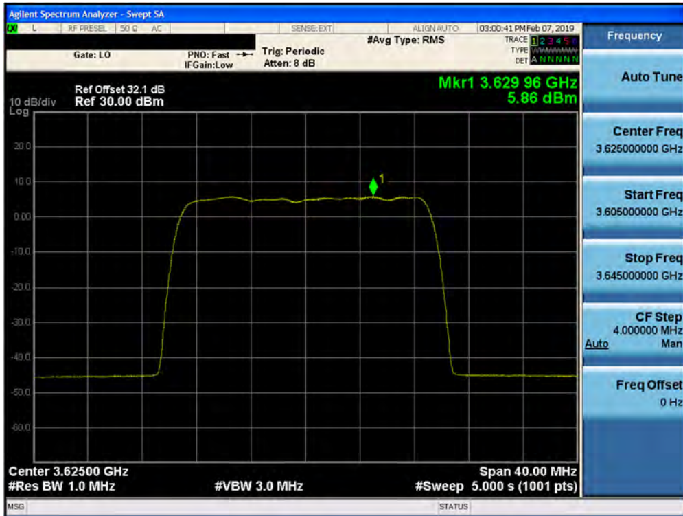
Plot 7-203. Peak Power Spectral Density Plot (1CC– 3625 MHz- 20.0MHz 16QAM- Mid Channel) Port 09
