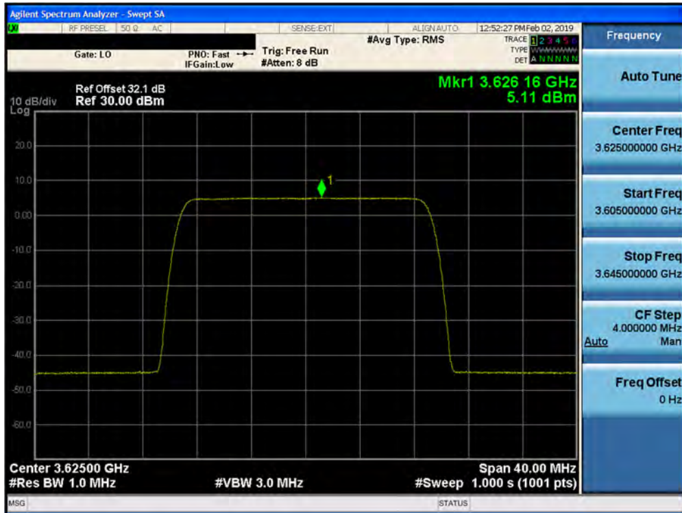
Plot 7-265. Peak Power Spectral Density Plot (1CC- 3625 MHz- 20.0MHz 256QAM- Mid Channel) Port 11
