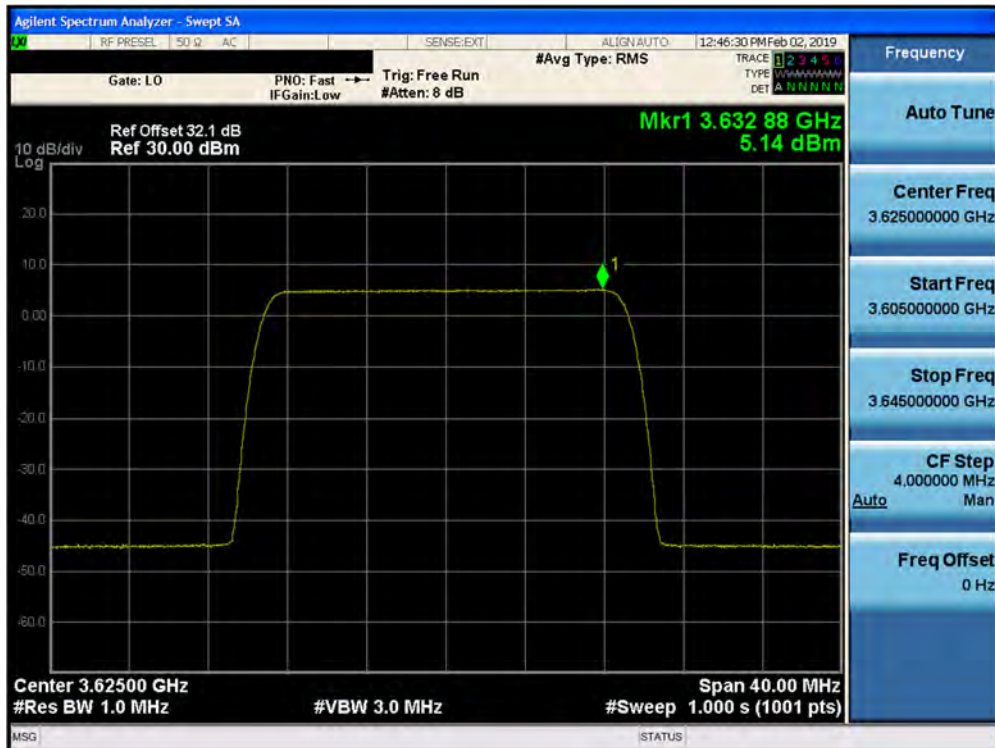
Plot 7-232. Peak Power Spectral Density Plot (1CC– 3625 MHz- 20.0MHz 64QAM- Mid Channel) Port 23
