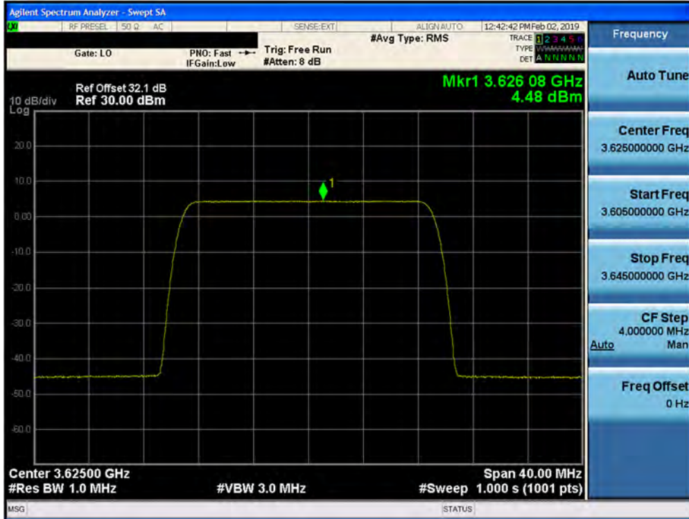
Plot 7-225. Peak Power Spectral Density Plot (1CC– 3625 MHz- 20.0MHz 64QAM- Mid Channel) Port 07
