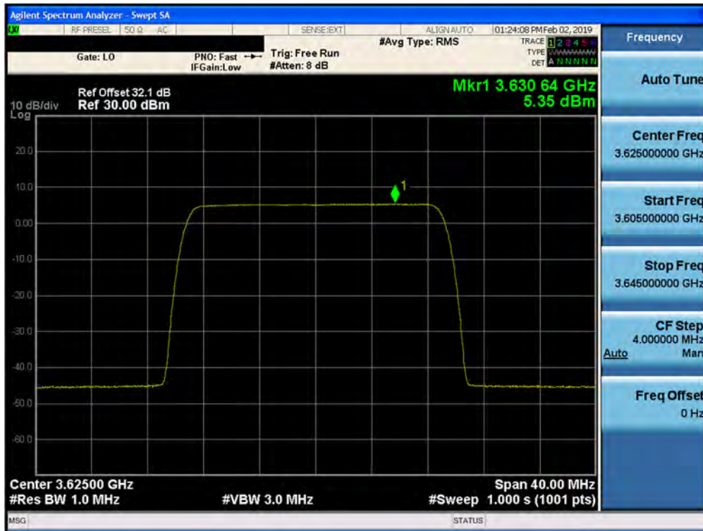
Plot 7-178. Peak Power Spectral Density Plot (1CC- 3625 MHz- 20.0MHz QPSK- Mid Channel) Port 14
