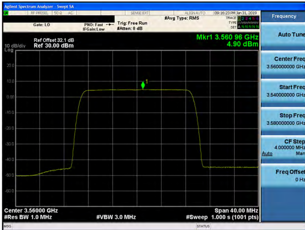
Plot 7-148. Peak Power Spectral Density Plot (1CC– 3560 MHz- 20.0MHz 256QAM- Low Channel) Port 12
