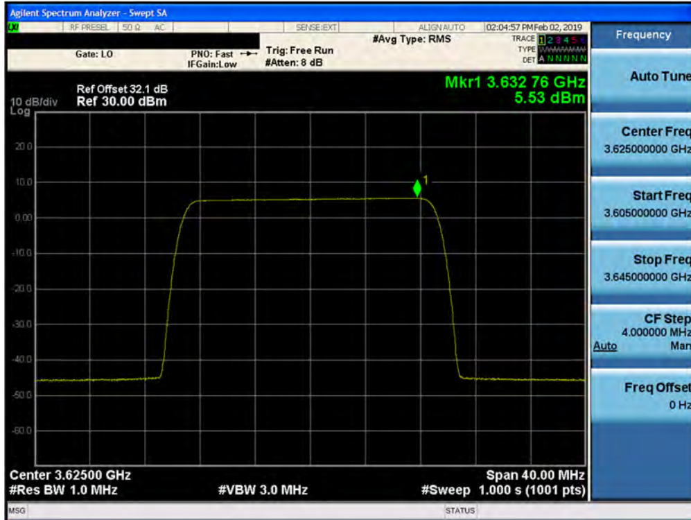
Plot 7-163. Peak Power Spectral Density Plot (1CC– 3625 MHz- 20.0MHz QPSK- Mid Channel) Port 05
