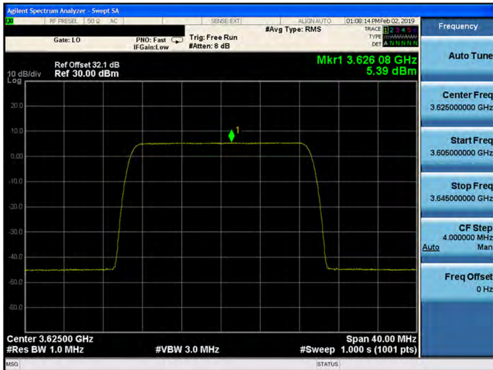
Plot 7-248. Peak Power Spectral Density Plot (1CC– 3625 MHz- 20.0MHz 64QAM- Mid Channel) Port 31
