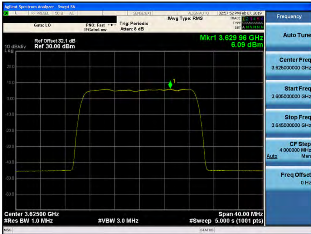
Plot 7-198. Peak Power Spectral Density Plot (1CC– 3625 MHz- 20.0MHz 16QAM- Mid Channel) Port 21
