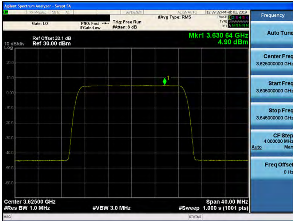
Plot 7-160. Peak Power Spectral Density Plot (1CC– 3625 MHz- 20.0MHz QPSK- Mid Channel) Port 19
