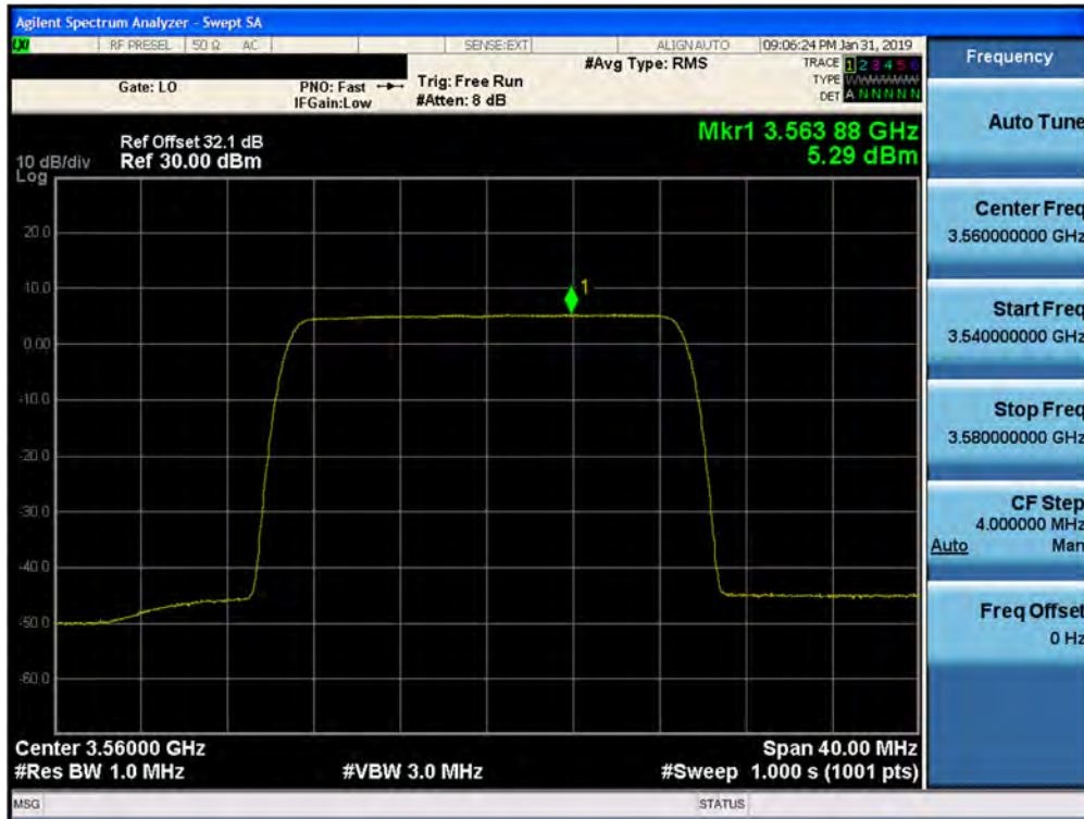
Plot 7-147. Peak Power Spectral Density Plot (1CC– 3560 MHz- 20.0MHz 256QAM- Low Channel) Port 13
