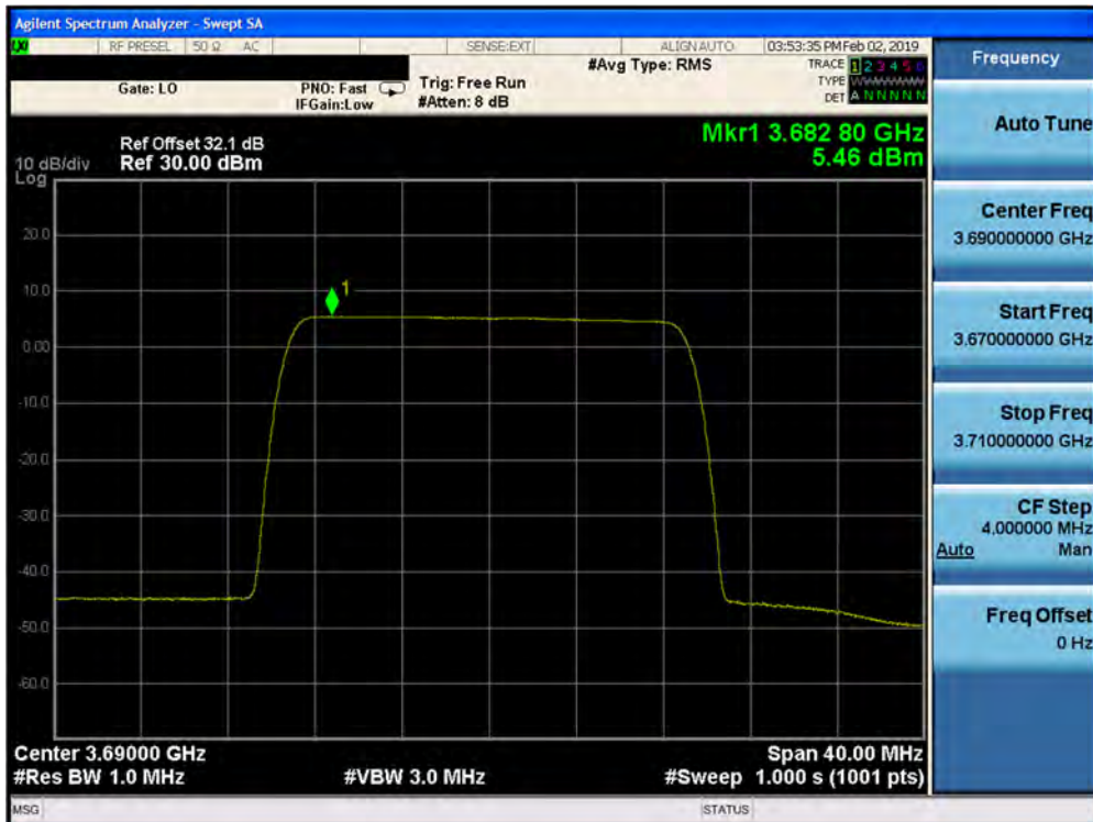
Plot 7-292. Peak Power Spectral Density Plot (1CC– 3690 MHz- 20.0MHz QPSK- High Channel) Port 04
