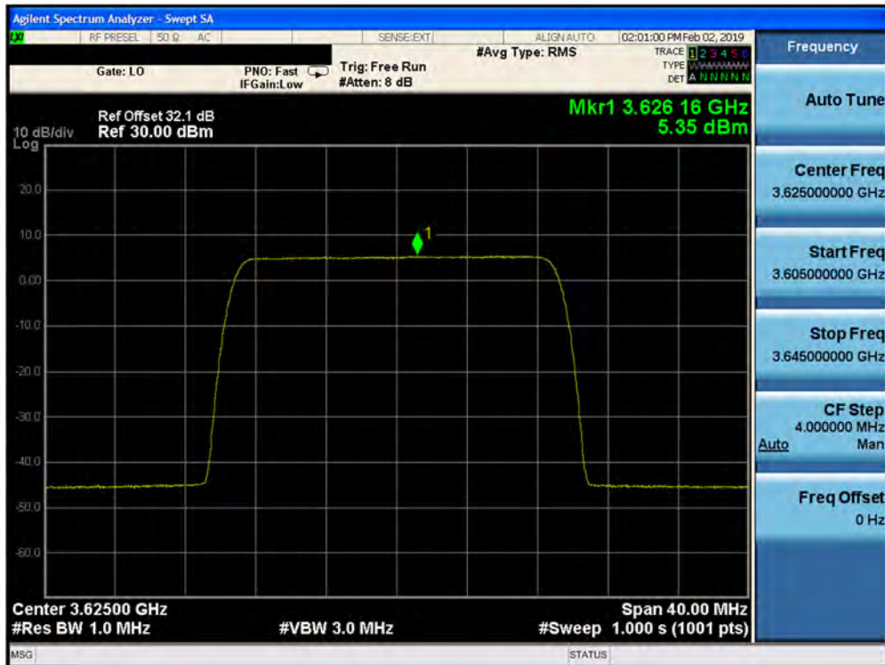
Plot 7-254. Peak Power Spectral Density Plot (1CC- 3625 MHz- 20.0MHz 256QAM- Mid Channel) Port 17
