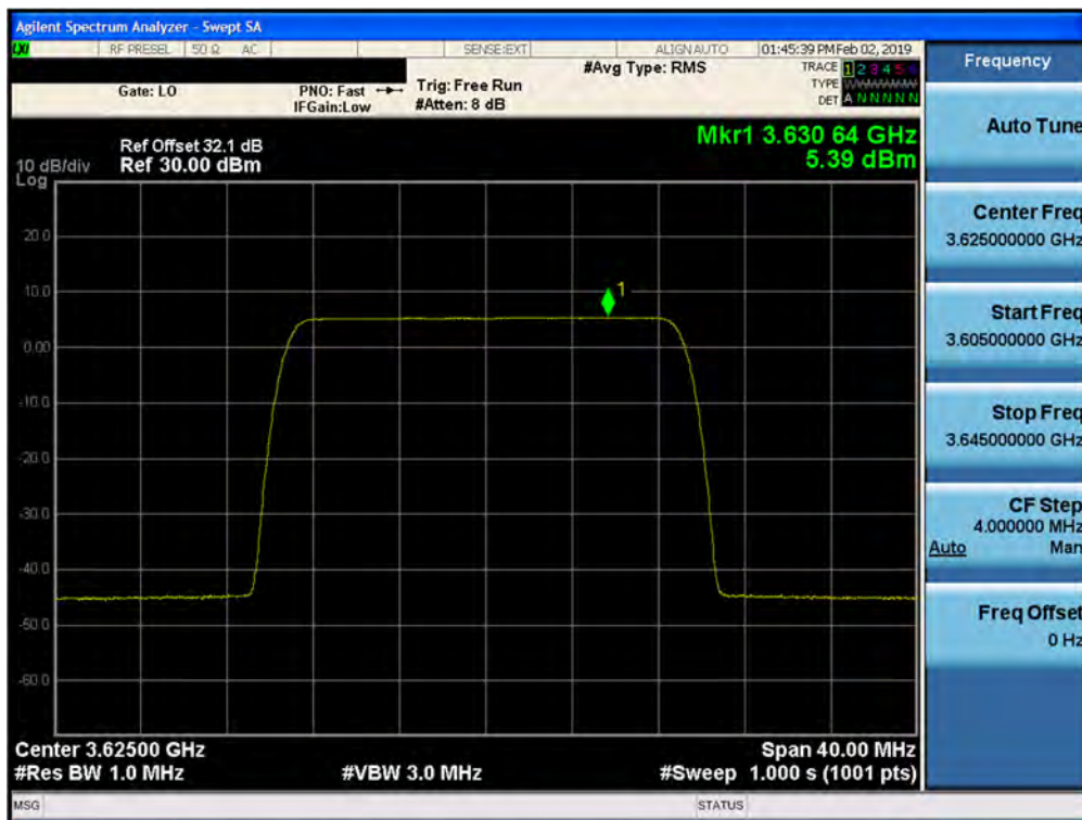
Plot 7-162. Peak Power Spectral Density Plot (1CC- 3625 MHz- 20.0MHz QPSK- Mid Channel) Port 06
