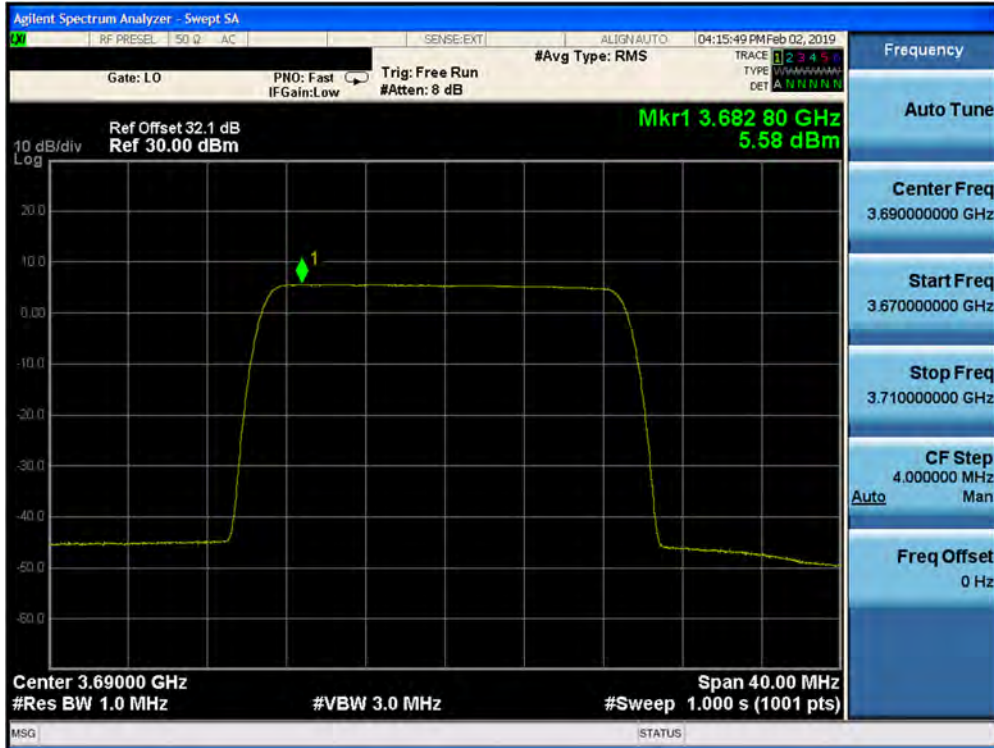
Plot 7-301. Peak Power Spectral Density Plot (1CC– 3690 MHz- 20.0MHz QPSK- High Channel) Port 24
