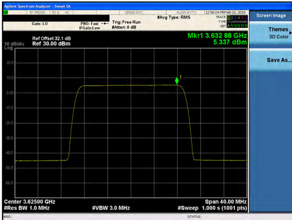
Plot 7-240. Peak Power Spectral Density Plot (1CC– 3625 MHz- 20.0MHz 64QAM- Mid Channel) Port 27
