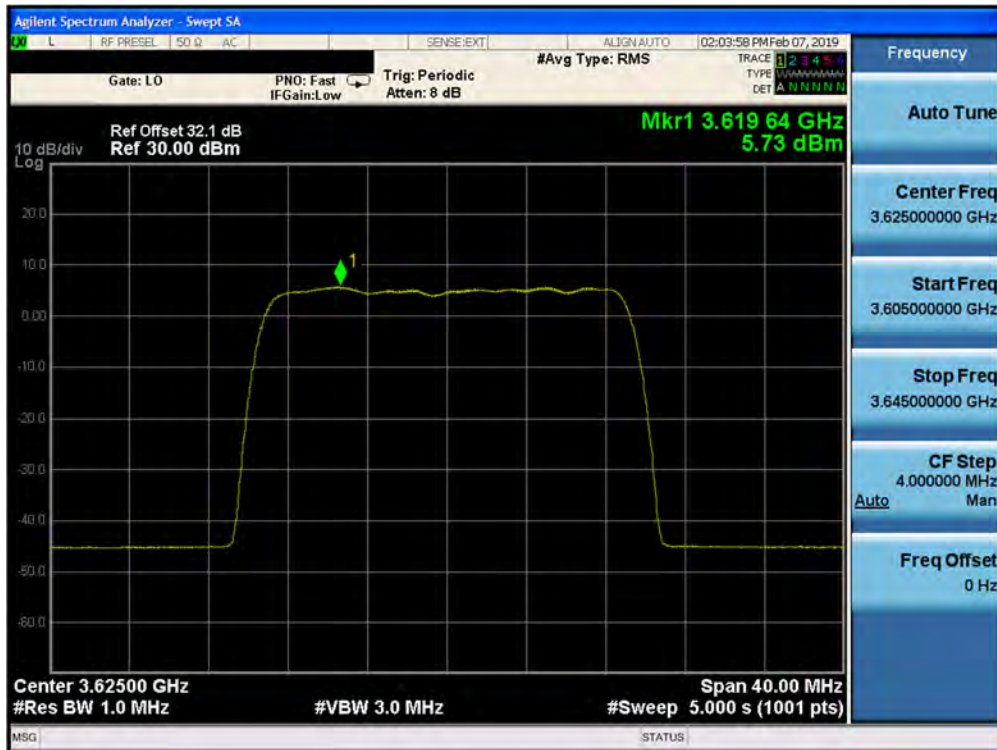
Plot 7-200. Peak Power Spectral Density Plot (1CC– 3625 MHz- 20.0MHz 16QAM- Mid Channel) Port 23
