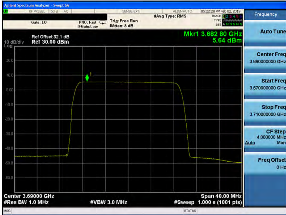
Plot 7-295. Peak Power Spectral Density Plot (1CC– 3690 MHz- 20.0MHz QPSK- High Channel) Port 22
