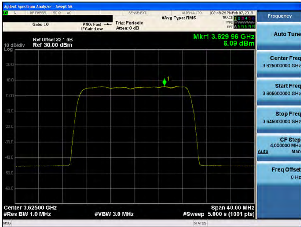
Plot 7-210. Peak Power Spectral Density Plot (1CC– 3625 MHz- 20.0MHz 16QAM- Mid Channel) Port 14
