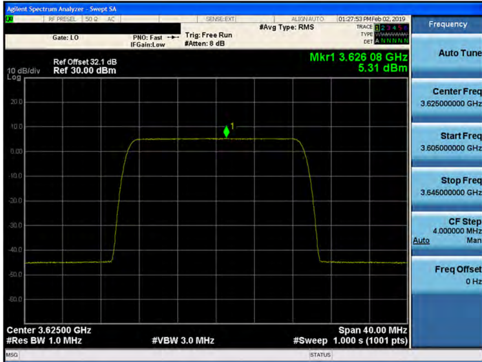
Plot 7-239. Peak Power Spectral Density Plot (1CC– 3625 MHz- 20.0MHz 64QAM- Mid Channel) Port 26
