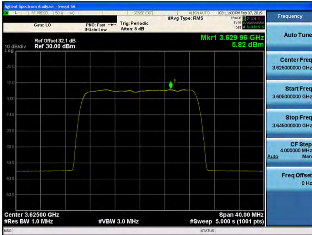
Plot 7-189. Peak Power Spectral Density Plot (1CC– 3625 MHz- 20.0MHz 16QAM- Mid Channel) Port 16
