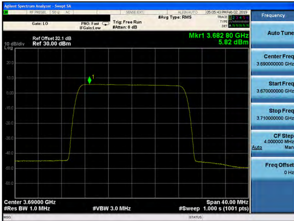
Plot 7-282. Peak Power Spectral Density Plot (1CC– 3690 MHz- 20.0MHz QPSK- High Channel) Port 02
