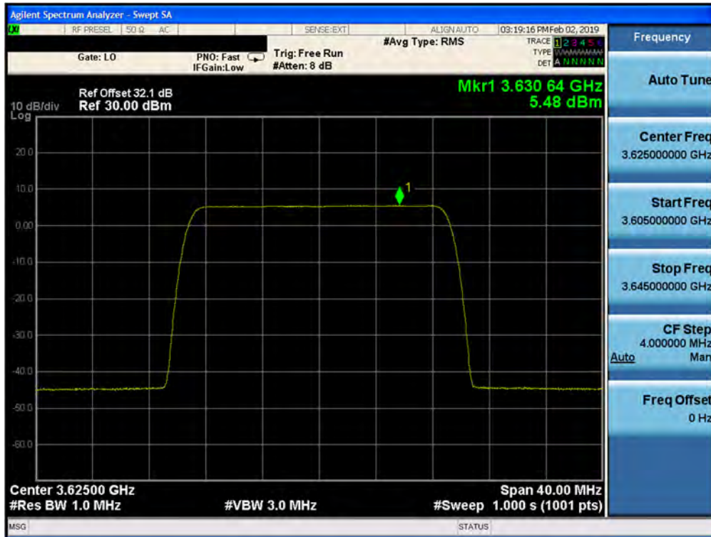
Plot 7-156. Peak Power Spectral Density Plot (1CC– 3625 MHz- 20.0MHz QPSK- Mid Channel) Port 00
