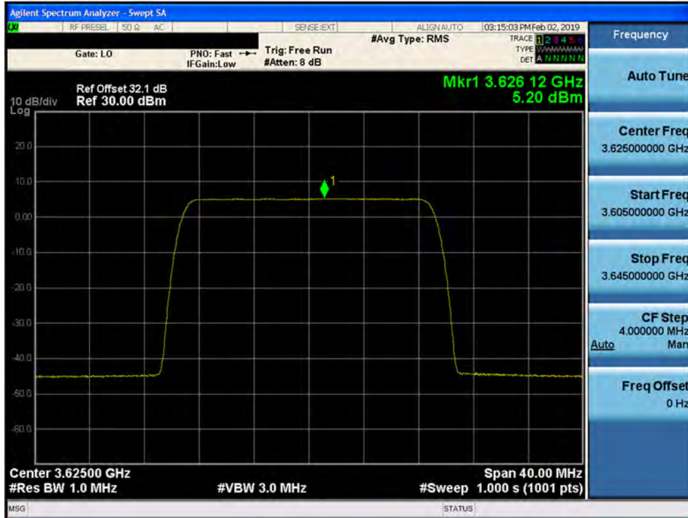
Plot 7-157. Peak Power Spectral Density Plot (1CC– 3625 MHz- 20.0MHz QPSK- Mid Channel) Port 16
