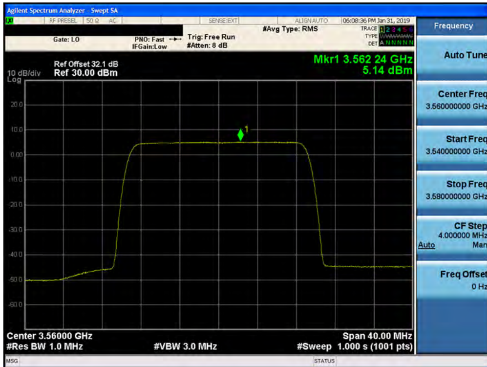
Plot 7-152. Peak Power Spectral Density Plot (1CC– 3560 MHz- 20.0MHz 256QAM- Low Channel) Port 31
