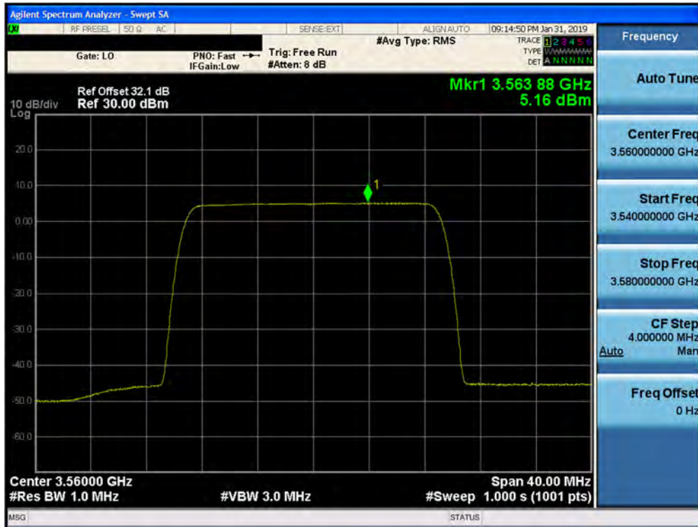
Plot 7-149. Peak Power Spectral Density Plot (1CC– 3560 MHz- 20.0MHz 256QAM- Low Channel) Port 28
