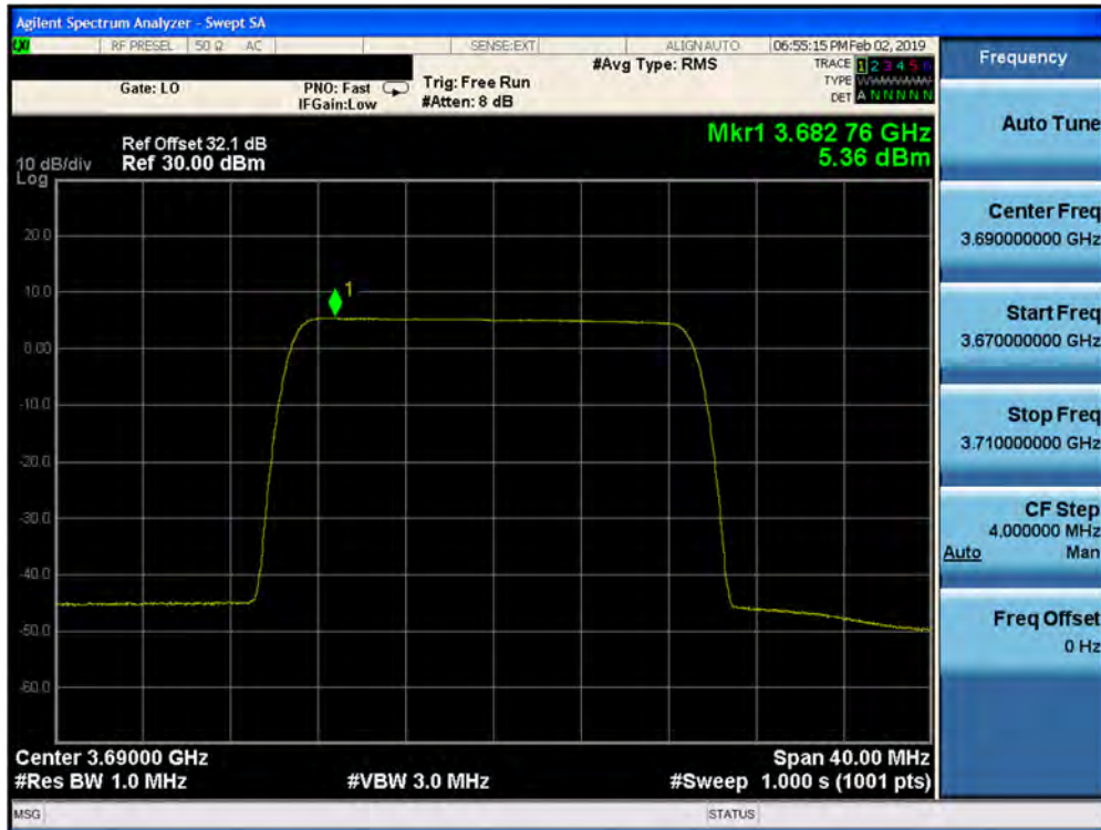
Plot 7-281. Peak Power Spectral Density Plot (1CC– 3690 MHz- 20.0MHz QPSK- High Channel) Port 03
