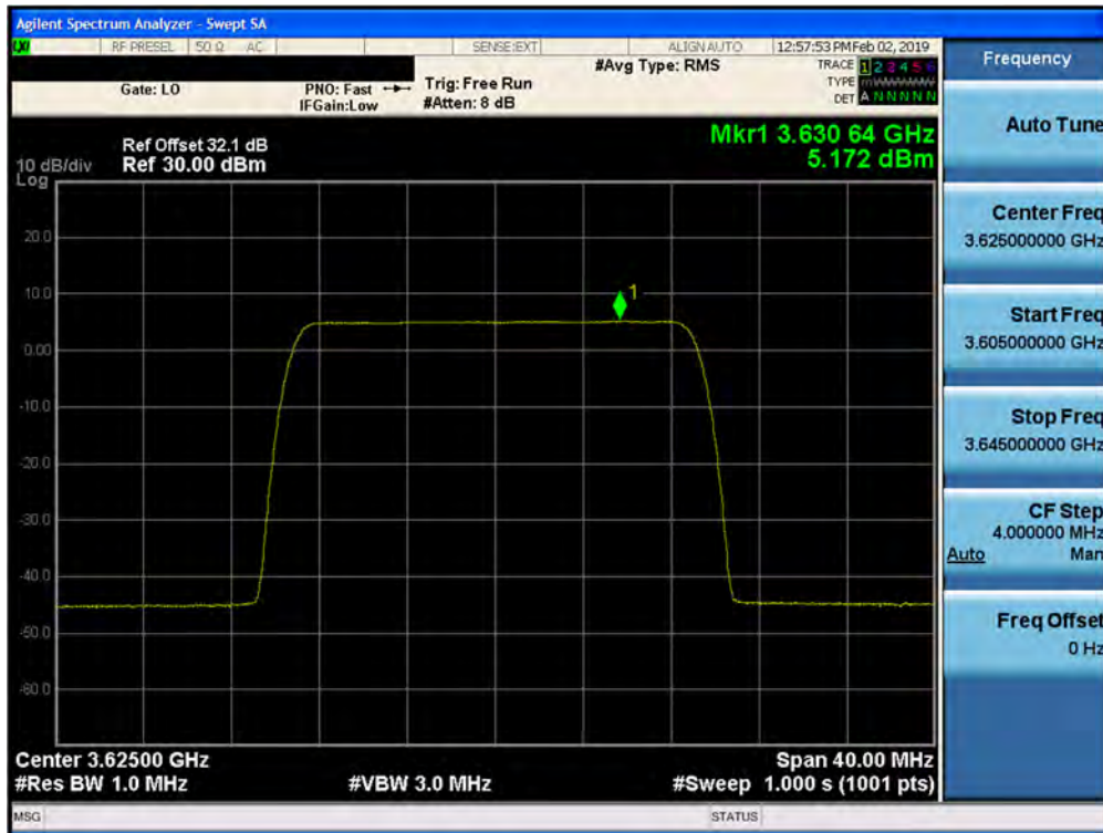
Plot 7-176. Peak Power Spectral Density Plot (1CC– 3625 MHz- 20.0MHz QPSK- Mid Channel) Port 27
