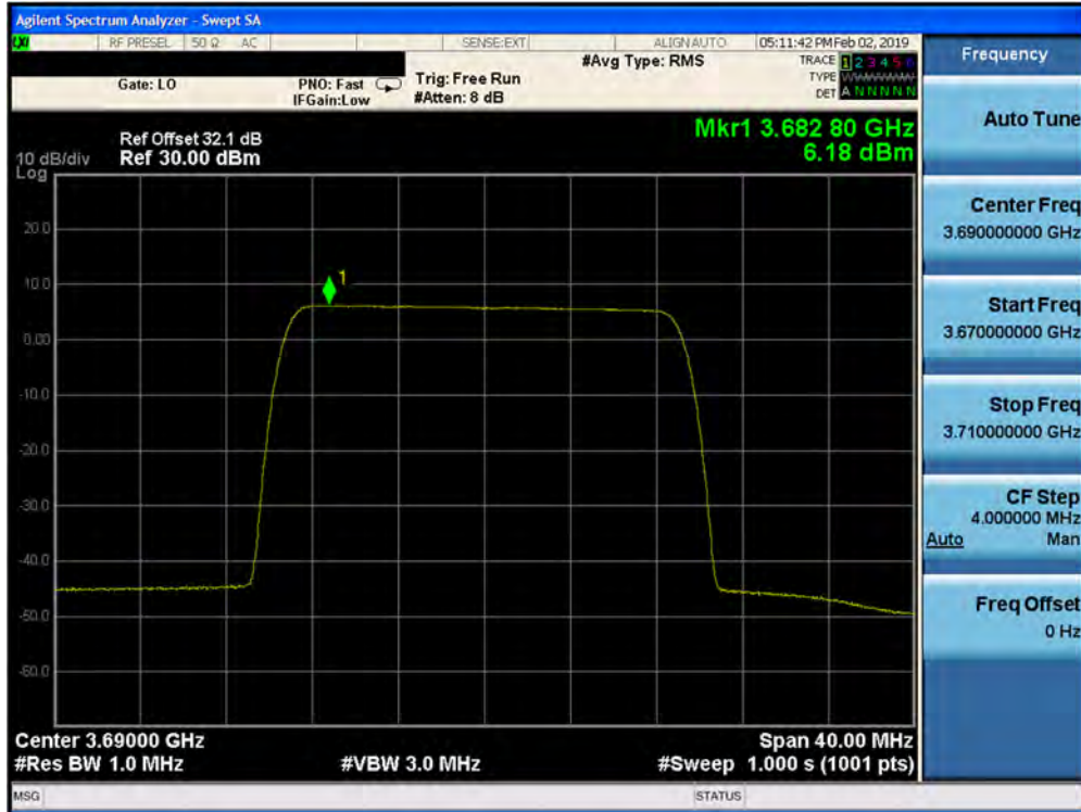
Plot 7-287. Peak Power Spectral Density Plot (1CC– 3690 MHz- 20.0MHz QPSK- High Channel) Port 18
