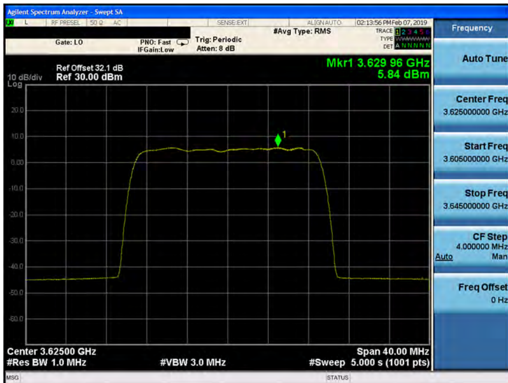
Plot 7-216. Peak Power Spectral Density Plot (1CC– 3625 MHz- 20.0MHz 16QAM- Mid Channel) Port 31
