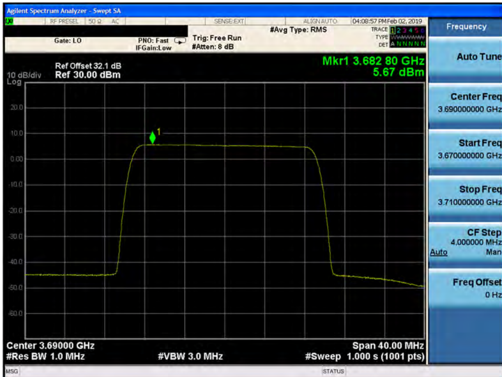
Plot 7-300. Peak Power Spectral Density Plot (1CC– 3690 MHz- 20.0MHz QPSK- High Channel) Port 08
