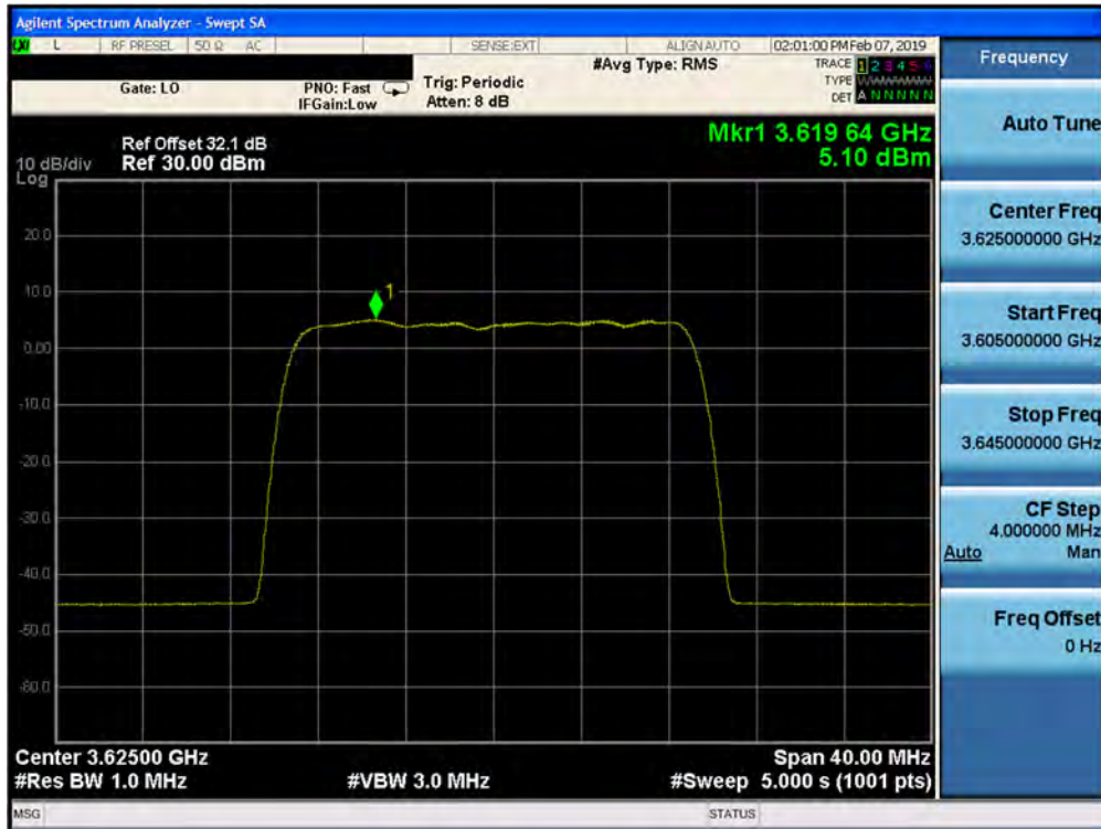
Plot 7-193. Peak Power Spectral Density Plot (1CC– 3625 MHz- 20.0MHz 16QAM- Mid Channel) Port 07
