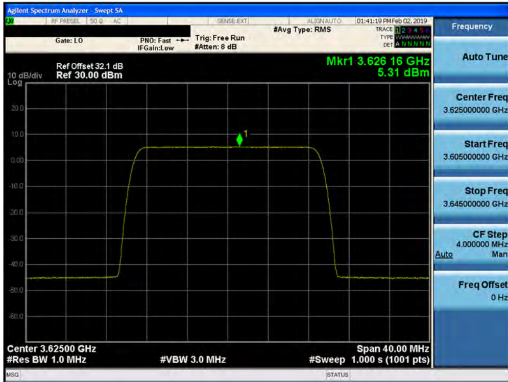
Plot 7-263. Peak Power Spectral Density Plot (1CC– 3625 MHz- 20.0MHz 256QAM- Mid Channel) Port 22
