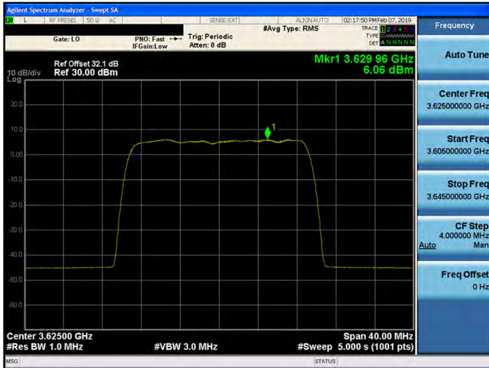
Plot 7-191. Peak Power Spectral Density Plot (1CC– 3625 MHz- 20.0MHz 16QAM- Mid Channel) Port 18
