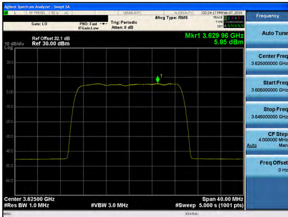
Plot 7-202. Peak Power Spectral Density Plot (1CC– 3625 MHz- 20.0MHz 16QAM- Mid Channel) Port 10
