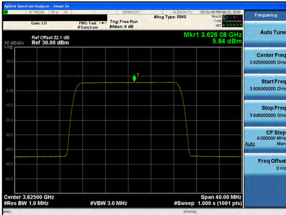
Plot 7-244. Peak Power Spectral Density Plot (1CC– 3625 MHz- 20.0MHz 64QAM- Mid Channel) Port 12
