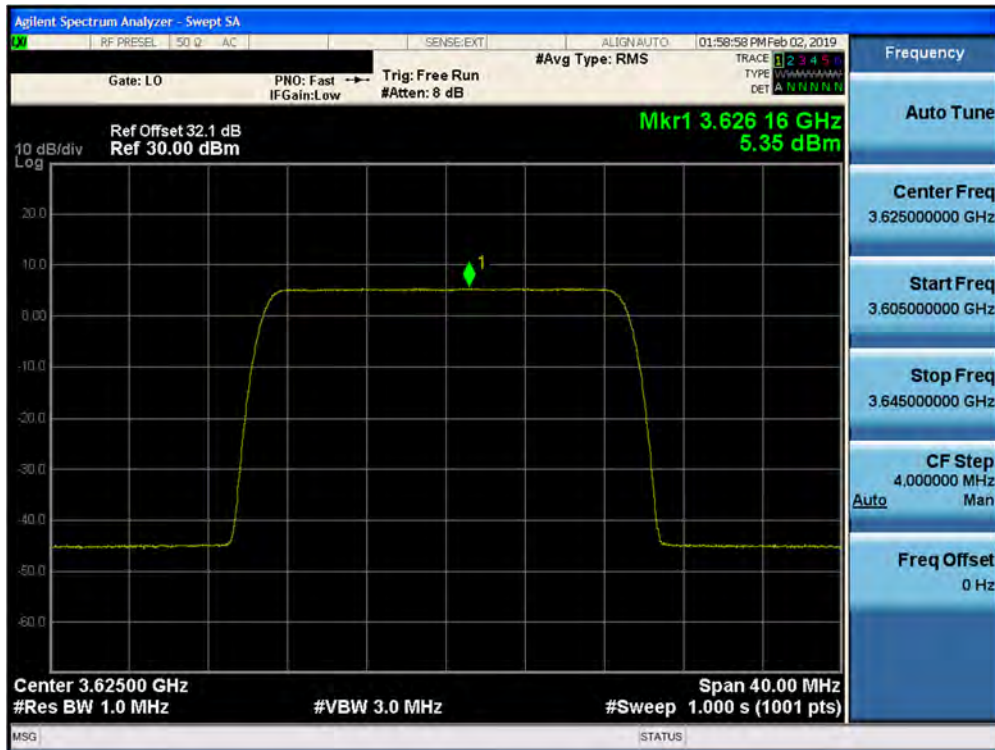
Plot 7-251. Peak Power Spectral Density Plot (1CC- 3625 MHz- 20.0MHz 256QAM- Mid Channel) Port 01
