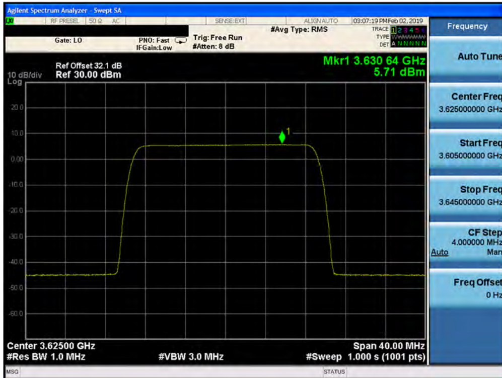
Plot 7-164. Peak Power Spectral Density Plot (1CC– 3625 MHz- 20.0MHz QPSK- Mid Channel) Port 04
