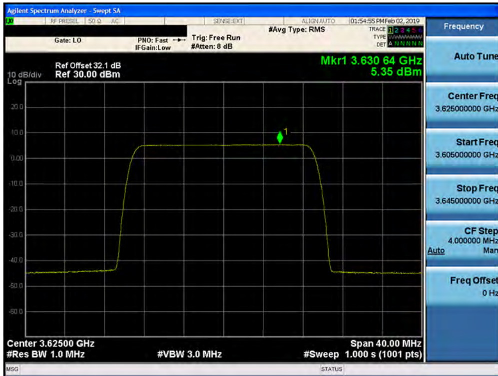
Plot 7-154. Peak Power Spectral Density Plot (1CC– 3625 MHz- 20.0MHz QPSK- Mid Channel) Port 02
