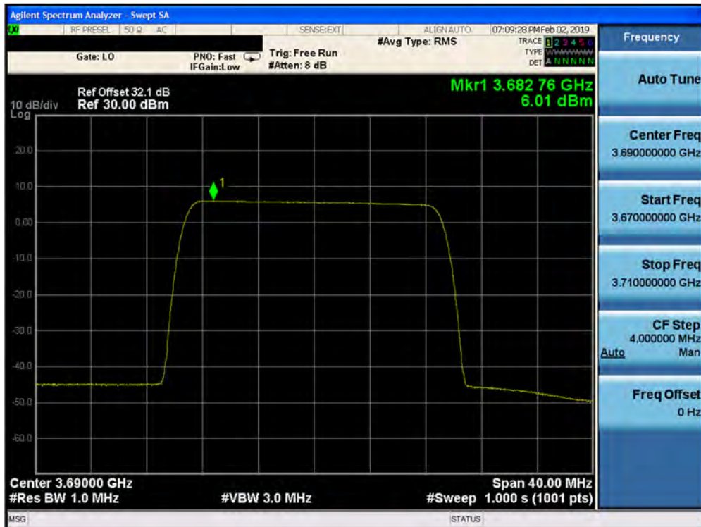
Plot 7-296. Peak Power Spectral Density Plot (1CC– 3690 MHz- 20.0MHz QPSK- High Channel) Port 23
