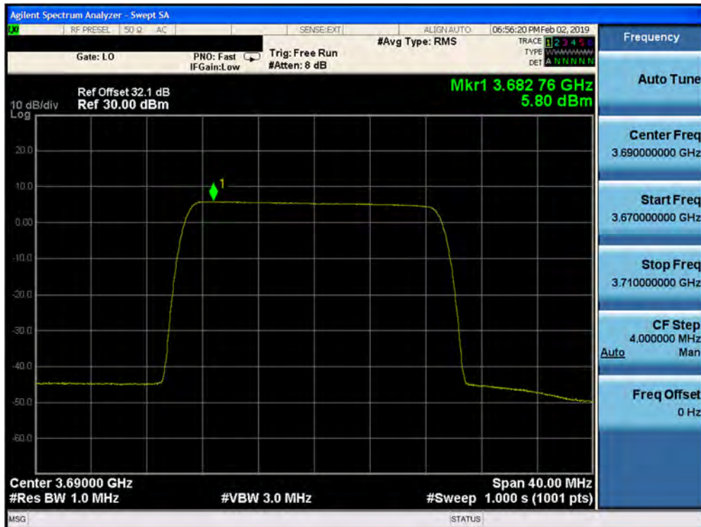
Plot 7-288. Peak Power Spectral Density Plot (1CC– 3690 MHz- 20.0MHz QPSK- High Channel) Port 19
