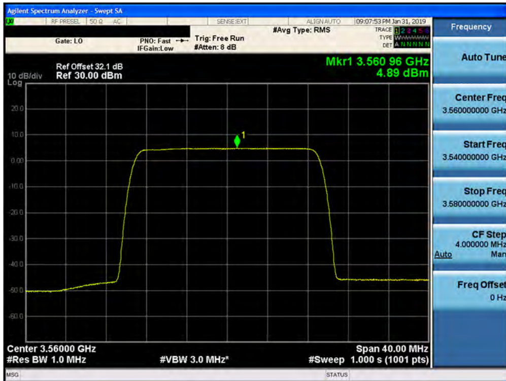
Plot 7-150. Peak Power Spectral Density Plot (1CC– 3560 MHz- 20.0MHz 256QAM- Low Channel) Port 29
