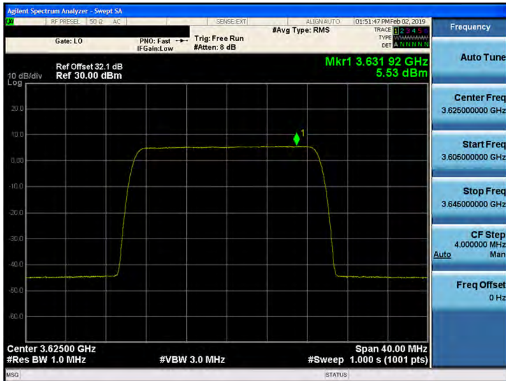
Plot 7-250. Peak Power Spectral Density Plot (1CC– 3625 MHz- 20.0MHz 256QAM- Mid Channel) Port 02
