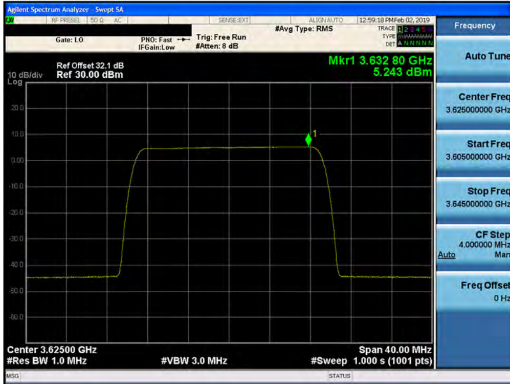
Plot 7-177. Peak Power Spectral Density Plot (1CC- 3625 MHz- 20.0MHz QPSK- Mid Channel) Port 15
