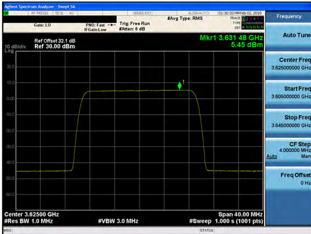
Plot 7-266. Peak Power Spectral Density Plot (1CC- 3625 MHz- 20.0MHz 256QAM- Mid Channel) Port 10
