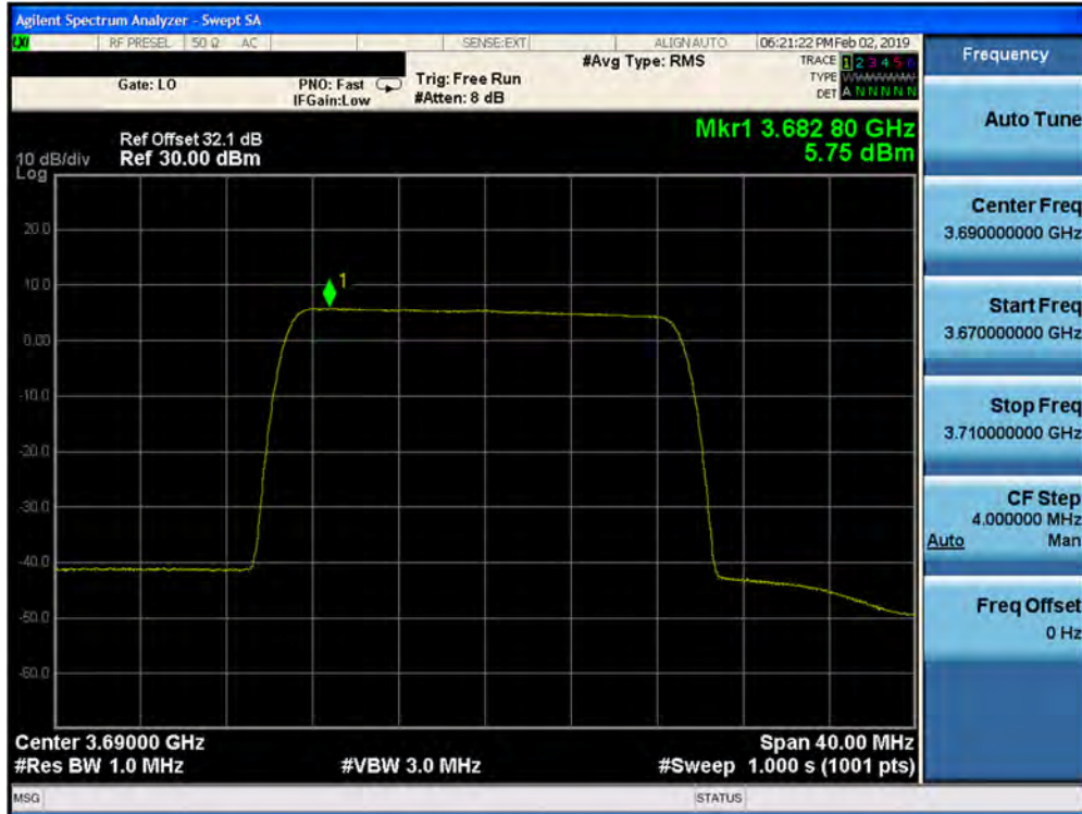
Plot 7-303. Peak Power Spectral Density Plot (1CC– 3690 MHz- 20.0MHz QPSK- High Channel) Port 26
