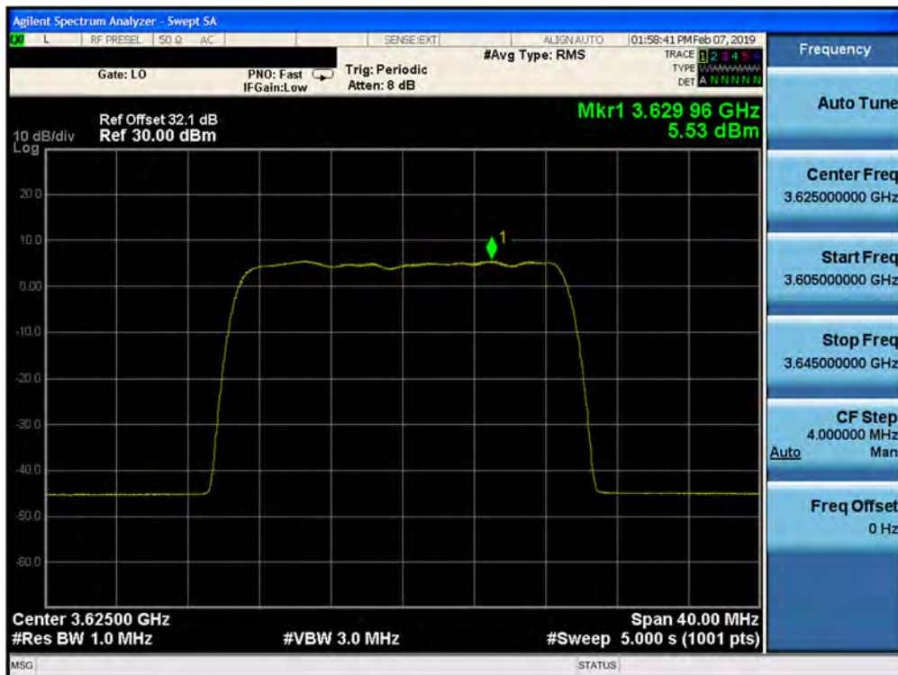
Plot 7-192. Peak Power Spectral Density Plot (1CC– 3625 MHz- 20.0MHz 16QAM- Mid Channel) Port 19
