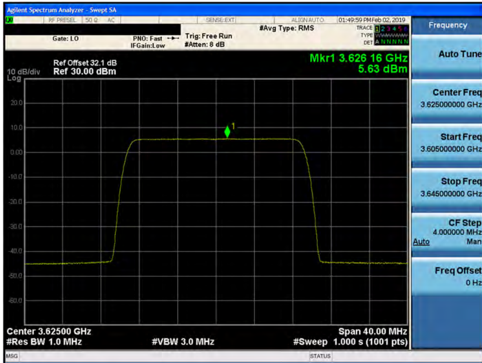
Plot 7-255. Peak Power Spectral Density Plot (1CC- 3625 MHz- 20.0MHz 256QAM- Mid Channel) Port 18
