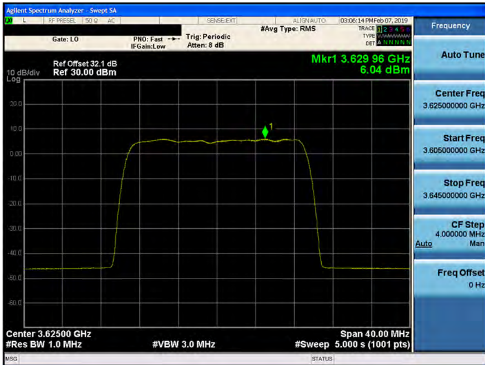
Plot 7-214. Peak Power Spectral Density Plot (1CC– 3625 MHz- 20.0MHz 16QAM- Mid Channel) Port 29
