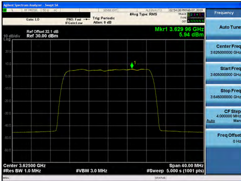
Plot 7-190. Peak Power Spectral Density Plot (1CC– 3625 MHz- 20.0MHz 16QAM- Mid Channel) Port 17
