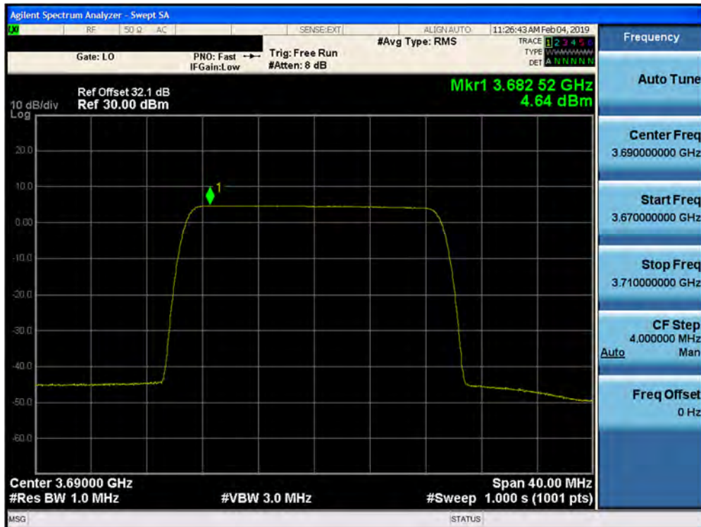
Plot 7-298. Peak Power Spectral Density Plot (1CC– 3690 MHz- 20.0MHz QPSK- High Channel) Port 10
