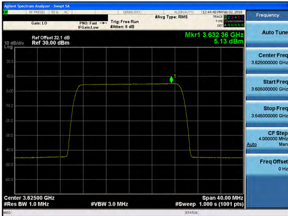
Plot 7-264. Peak Power Spectral Density Plot (1CC– 3625 MHz- 20.0MHz 256QAM- Mid Channel) Port 23
