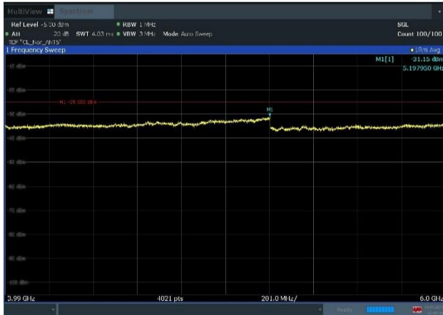
Plot 8-91. Conducted Spurious Emission Plot (3990MHz to 6GHz) (n77_2C_100M+40M_16QAM - Mid Channel, Port 5)
