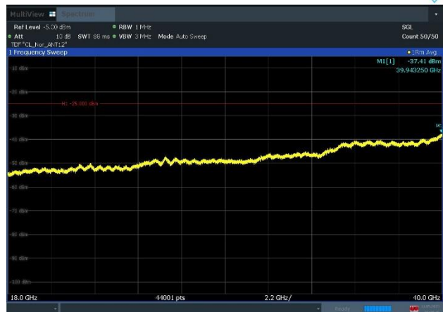
Plot 8-84. Conducted Spurious Emission Plot (18GHz to 40GHz) (n77_1C_100M_QPSK - Low Channel, Port 12)
