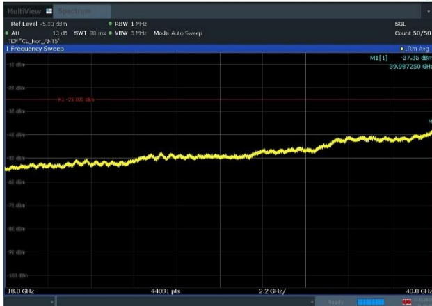
Plot 8-93. Conducted Spurious Emission Plot (18GHz to 40GHz) (n77_2C_100M+40M_16QAM - Mid Channel, Port 5)
