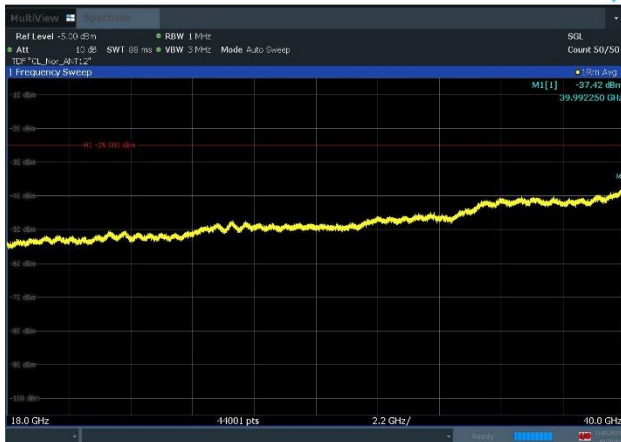
Plot 8-75. Conducted Spurious Emission Plot (18GHz to 40GHz) (n77_1C_80M_16QAM - High Channel, Port 12)
