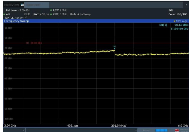
Plot 8-100. Conducted Spurious Emission Plot (3990MHz to 6GHz) (n77_2C_100M+100M_16QAM - Mid Channel, Port 4)
