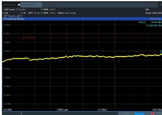
Plot 8-101. Conducted Spurious Emission Plot (6GHz to 18GHz) (n77_2C_100M+100M_16QAM - Mid Channel, Port 4)
