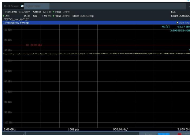
Plot 8-71. Conducted Spurious Emission Plot (3690MHz to 3699MHz) (n77_1C_80M_16QAM - High Channel, Port 12)
