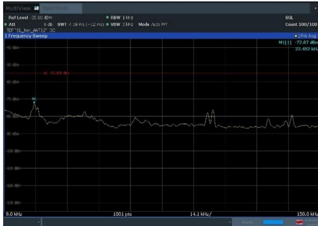
Plot 8-49. Conducted Spurious Emission Plot (9KHz to 150KHz) (n77_1C_40M_256QAM - High Channel, Port 12)
