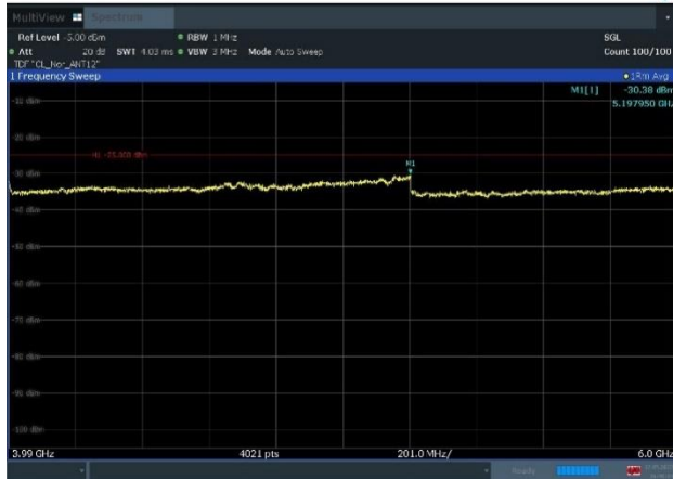
Plot 8-55. Conducted Spurious Emission Plot (3990MHz to 6GHz) (n77_1C_40M_256QAM - High Channel, Port 12)
