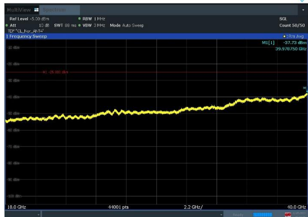
Plot 8-66. Conducted Spurious Emission Plot (18GHz to 40GHz) (n77_1C_60M_QPSK - Low Channel, Port 4)
