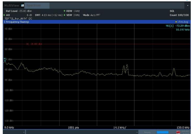
Plot 8-58. Conducted Spurious Emission Plot (9KHz to 150KHz) (n77_1C_60M_QPSK - Low Channel, Port 4)
