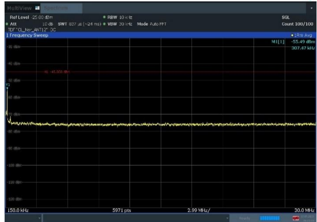
Plot 8-50. Conducted Spurious Emission Plot (150KHz to 30MHz) (n77_1C_40M_256QAM - High Channel, Port 12)
