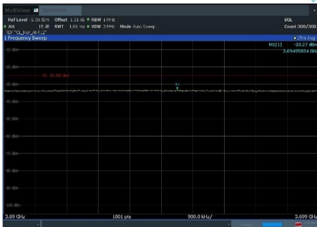
Plot 8-53. Conducted Spurious Emission Plot (3690MHz to 3699MHz) (n77_1C_40M_256QAM - High Channel, Port 12)
