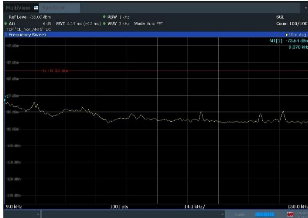
Plot 8-85. Conducted Spurious Emission Plot (9KHz to 150KHz) (n77_2C_100M+40M_16QAM - Mid Channel, Port 5)
