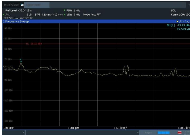
Plot 8-67. Conducted Spurious Emission Plot (9KHz to 150KHz) (n77_1C_80M_16QAM - High Channel, Port 12)
