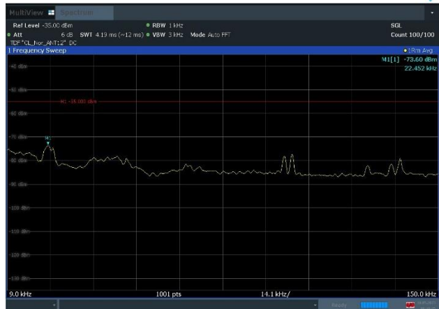
Plot 8-76. Conducted Spurious Emission Plot (9KHz to 150KHz) (n77_1C_100M_QPSK - Low Channel, Port 12)
