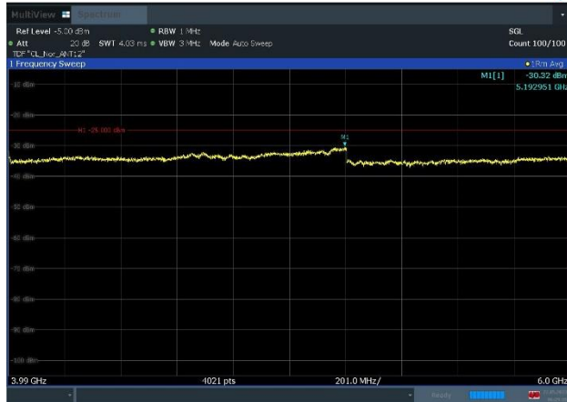
Plot 8-73. Conducted Spurious Emission Plot (3990MHz to 6GHz) (n77_1C_80M_16QAM - High Channel, Port 12)
