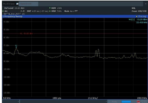
Plot 8-94. Conducted Spurious Emission Plot (9KHz to 150KHz) (n77_2C_100M+100M_16QAM - Mid Channel, Port 4)
