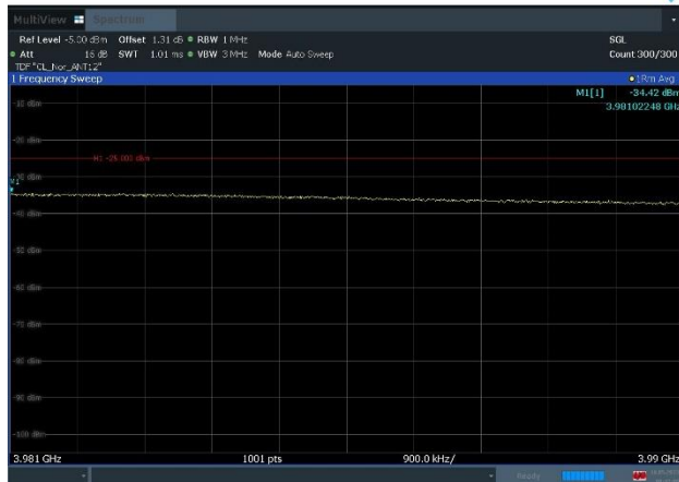
Plot 8-81. Conducted Spurious Emission Plot (3981MHz to 3990GHz) (n77_1C_100M_QPSK - Low Channel, Port 12)
