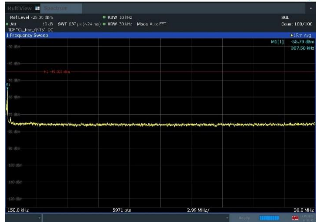
Plot 8-86. Conducted Spurious Emission Plot (150KHz to 30MHz) (n77_2C_100M+40M_16QAM - Mid Channel, Port 5)
