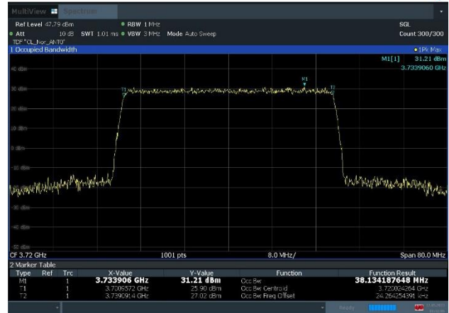
Plot 8-2. Occupied Bandwidth Plot (n77_1C_40M_64AM - Low Channel)
