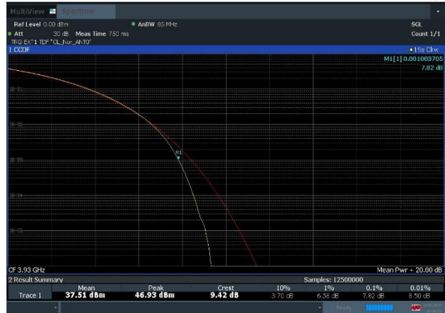
Plot 8-32. Peak To Average Power Ratio Plot (n77_1C_100M_256QAM - High Channel)
