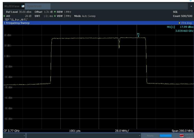
Plot 8-22. Peak Power Spectral Density Plot (n77_2C_100M+40M_16QAM - Mid Channel, Port 1)
