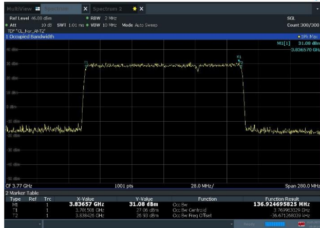
Plot 8-9. Occupied Bandwidth Plot (n77_2C_100+40M_QPSK - Mid Channel)
