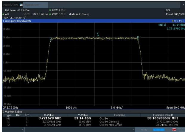
Plot 8-1. Occupied Bandwidth Plot (n77_1C_40M_QPSK - Low Channel)
