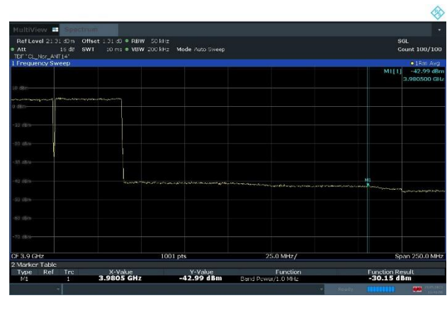
Plot 8-46. Band Edge Emission Plot (n77_2C_100M+40M_QPSK - Mid Channel High Edge, Port 14)
