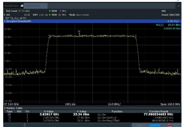
Plot 8-6. Occupied Bandwidth Plot (n77_1C_80M_64QAM - Mid Channel)
