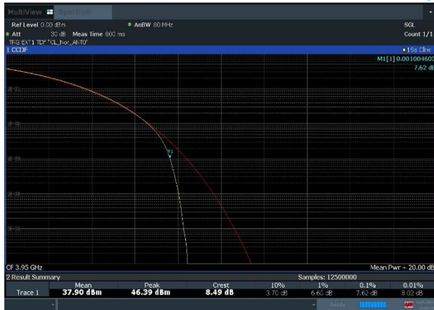
Plot 8-27. Peak To Average Power Ratio Plot (n77_1C_60M_QPSK - High Channel)
