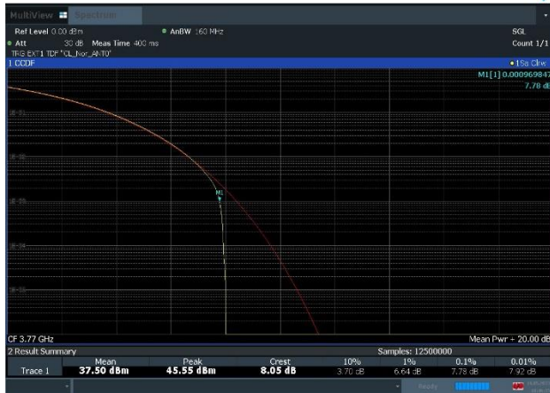
Plot 8-33. Peak To Average Power Ratio Plot (n77_2C_100M+40M_QPSK - Mid Channel)
