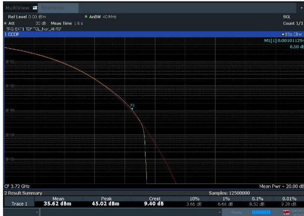
Plot 8-25. Peak To Average Power Ratio Plot (n77_1C_40M_QPSK - Low Channel)
