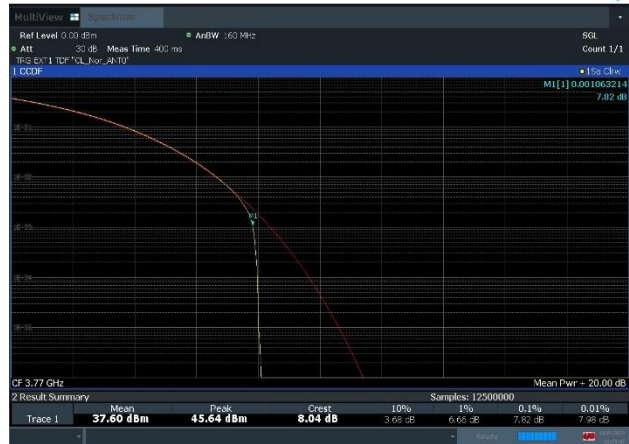
Plot 8-34. Peak To Average Power Ratio Plot (n77_2C_100M+40M_16QAM - Mid Channel)
