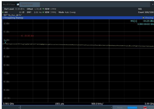
Plot 8-63. Conducted Spurious Emission Plot (3981MHz to 3990GHz) (n77_1C_60M_QPSK - Low Channel, Port 4)
