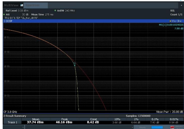
Plot 8-36. Peak To Average Power Ratio Plot (n77_2C_100M+100M_16QAM - Mid Channel)
