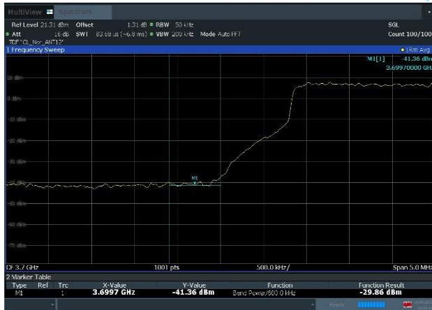
Plot 8-39. Band Edge Emission Plot (n77_1C_60M_16QAM - Low Channel, Port 12)
