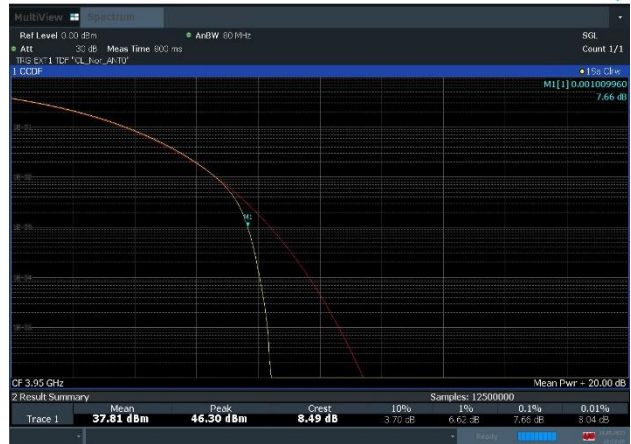
Plot 8-28. Peak To Average Power Ratio Plot (n77_1C_60M_16QAM - High Channel)
