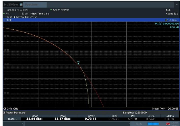
Plot 8-26. Peak To Average Power Ratio Plot (n77_1C_40M_256QAM - High Channel)
