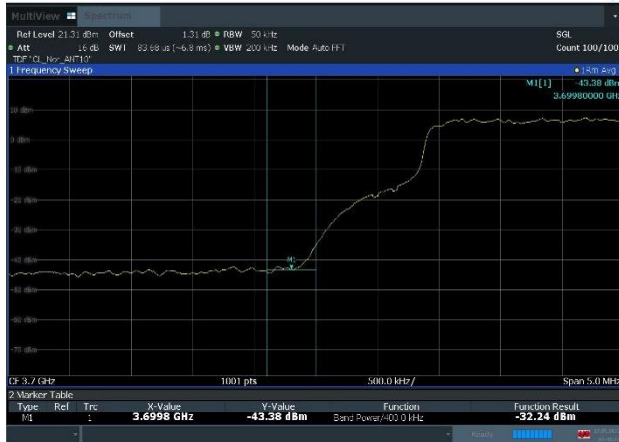
Plot 8-37. Band Edge Emission Plot (n77_1C_40M_64QAM - Low Channel, Port 10)
