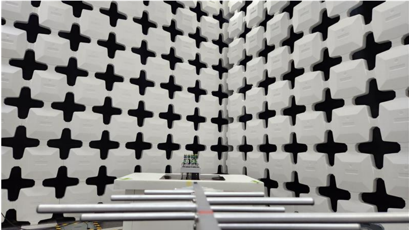
Below 1GHz Test Instrument & Measurement Setup
