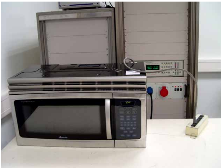
Fig. 2 Test Setup for Input power
