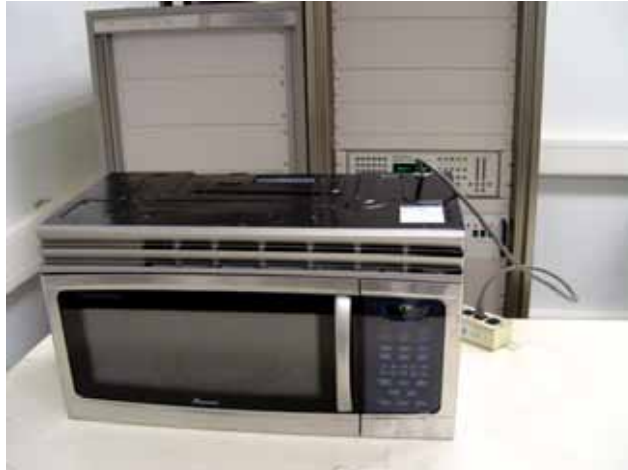
Fig.3 Test Setup for RF output power
