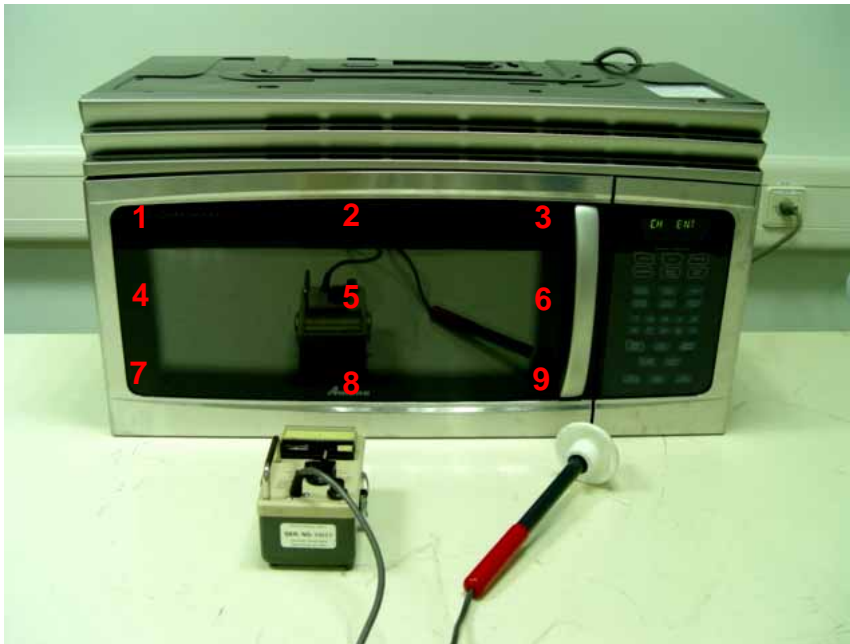
Fig. 1 Test Setup for Radiation Hazard Measurement
