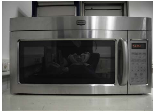
Fig.3 Test Setup for RF output power
