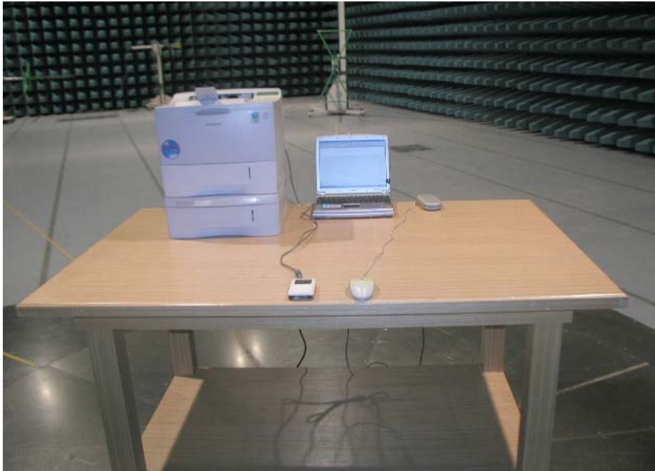
Pic. 3 Radiated Emission (Front)
