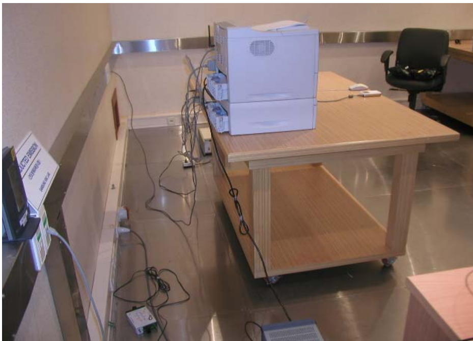
Pic. 2 Conducted Emission (Rear)
