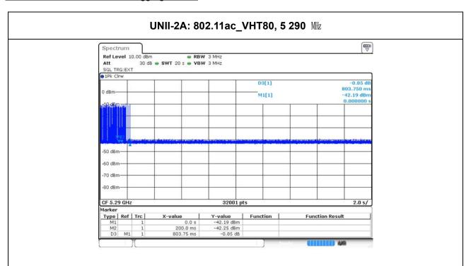
Channel move time = 0.803750 sClosing time =  $0.000625 \text{ s} \times 42 = 0.026250 \text{ s}$
