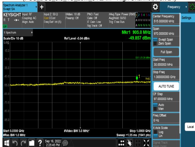
Plot 8-173. Conducted Spurious Emission Plot 30 MHz to 1 GHz (PCS_DSS_5:5_1C_20M_64QAM - High Channel, Port 24)
