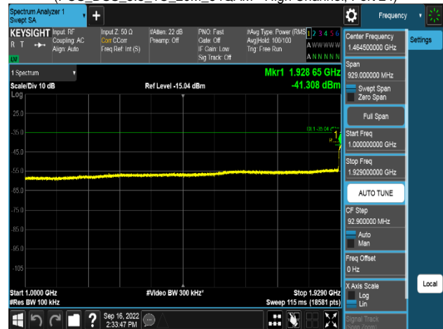
Plot 8-174. Conducted Spurious Emission Plot 1 GHz to 1.929 GHz (PCS_DSS_5:5_1C_20M_64QAM - High Channel, Port 24)
