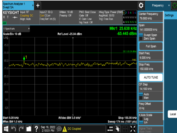
Plot 8-171. Conducted Spurious Emission Plot 9 kHz to 150 kHz (PCS_DSS_5:5_1C_20M_64QAM - High Channel, Port 24)
