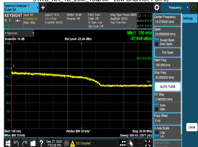
Plot 8-188. Conducted Spurious Emission Plot 150 kHz to 30 MHz (PCS_DSS_1C_15M + LTE_1C_5M_256QAM - High Channel, Port 30)
