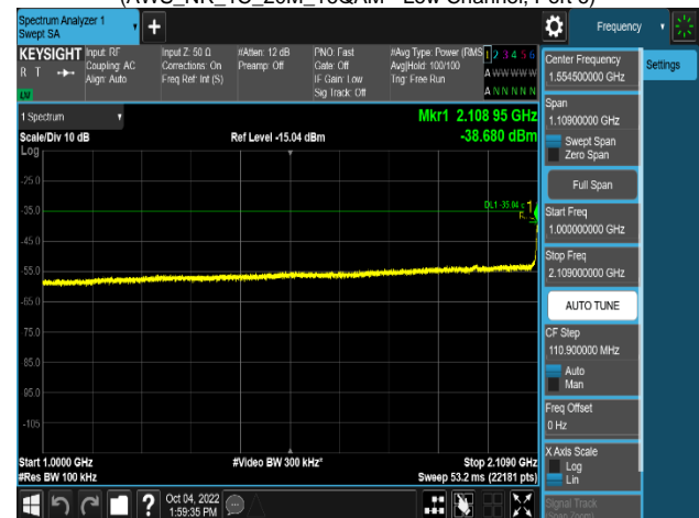
Plot 8-182. Conducted Spurious Emission Plot 1 GHz to 2.109 GHz (AWS_NR_1C_20M_16QAM - Low Channel, Port 6)
