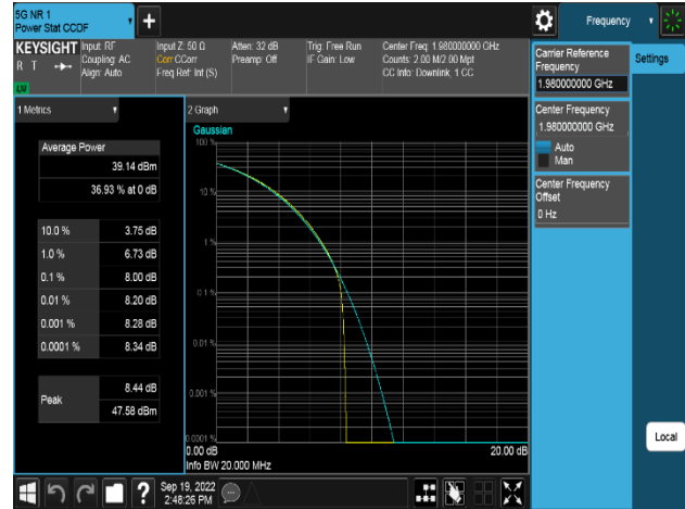
Plot 8-116. Peak To Average Power Ratio Plot (PCS_DSS 5:5_1C_20M_256QAM - High Channel, Port 25)
