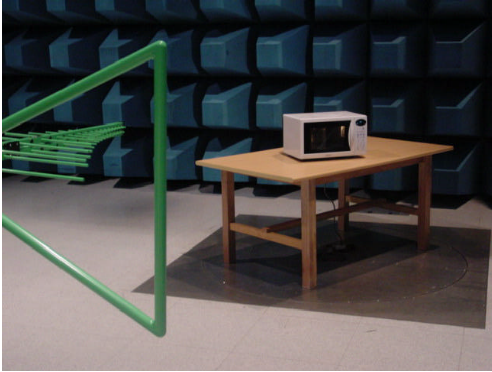
Fig. 4 Test Setup for Radiated Emission(1 - 25GHz)
