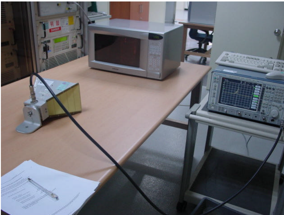
Fig. 2 Test Setup for Operating Frequency Measurements
