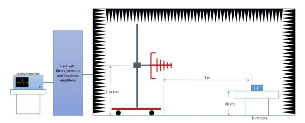
4) Radiated Setup (1 GHz ~ 18 GHz)
