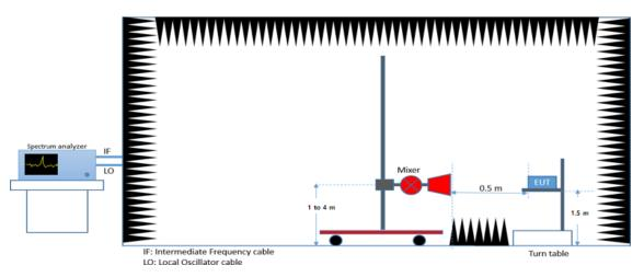
According to ANSI C63.10-2013, Clause 9, the measurement should be performed at a distance greater than or equal to the far field boundary distance. This later is given by
