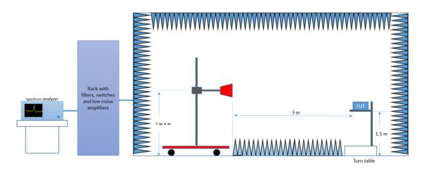
5) Radiated Setup (18 GHz ~ 40 GHz)
