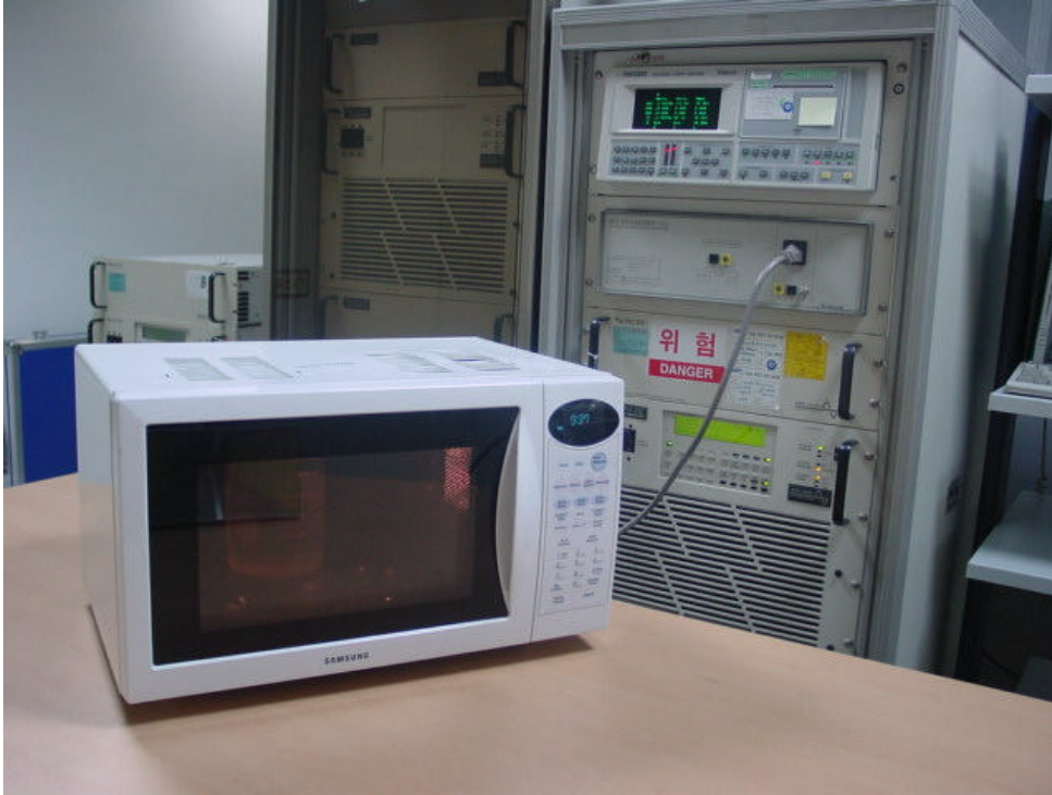
Fig. 1 Test Setup for Input power & RF output power
