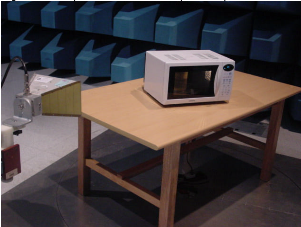
Fig. 4 Test Setup for Radiated Emission(1 - 25GHz)
