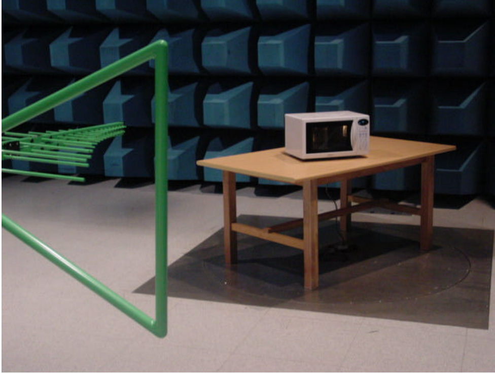
Fig. 3 Test Setup for Radiated Emission(30 - 1000MHz)
