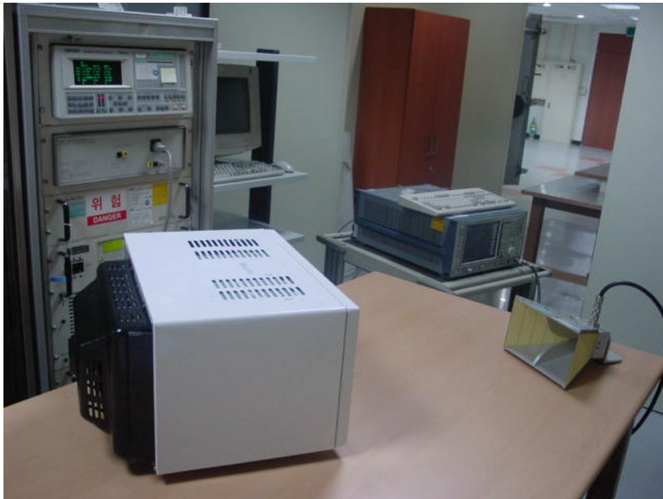
Fig. 2 Test Setup for Operating Frequency Measurements
